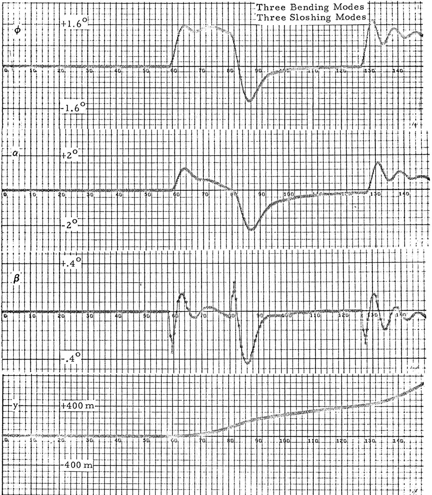
Figure 2-14a - Saturn V, S-IC Stage Response to  $\phi_c$  with all Bending Mode Signs Reversed - Digital Nonlinear Filter ( $\omega_s = 96$  rad/sec)
