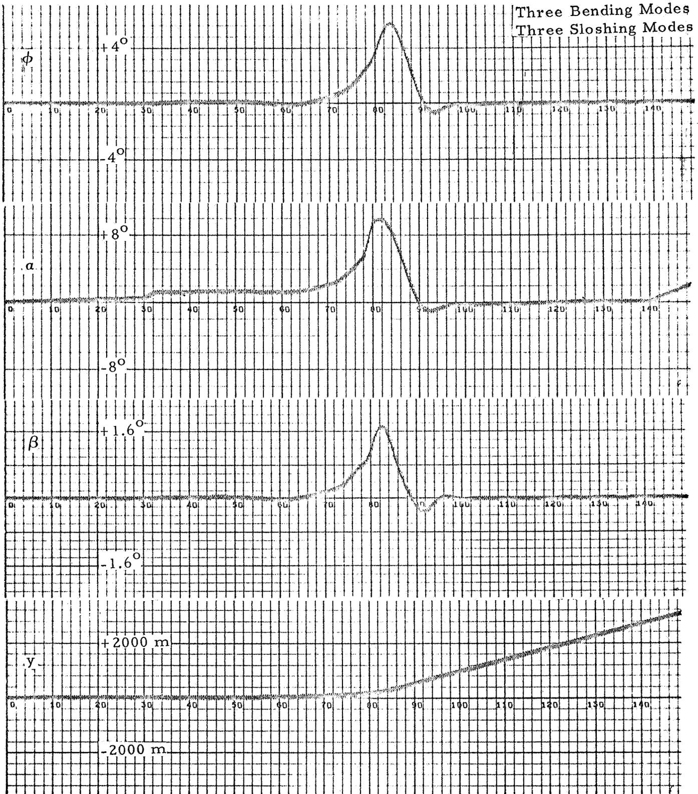
Figure 2-6a - Saturn V, S-IC Stage Response to Wind Disturbance - Digital Nonlinear Filter ( $\omega_s = 24$  rad/sec).
