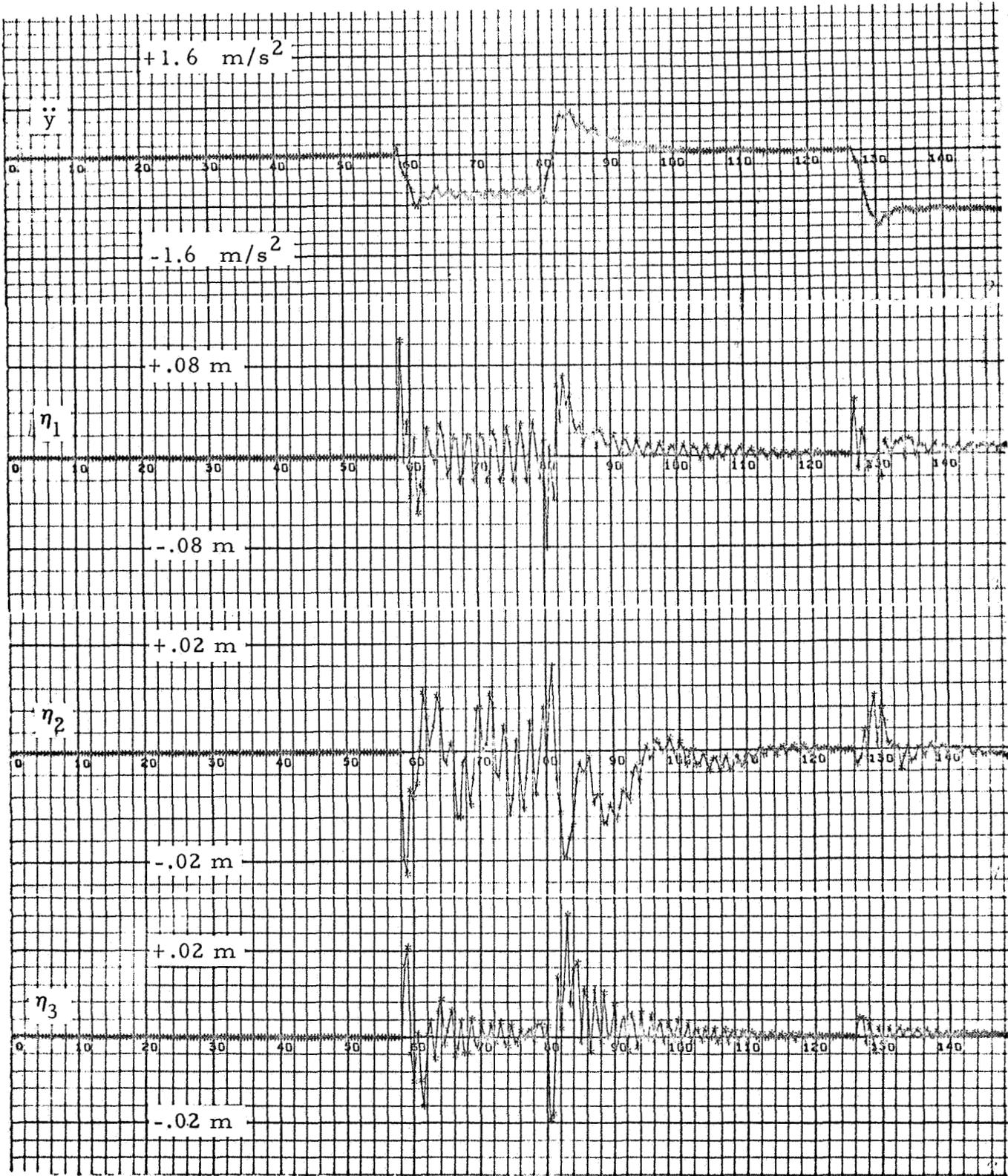
Figure 2-9b - Saturn V, S-IC Stage Response to  $\phi_C$  - AS-503 Linear Filters.
