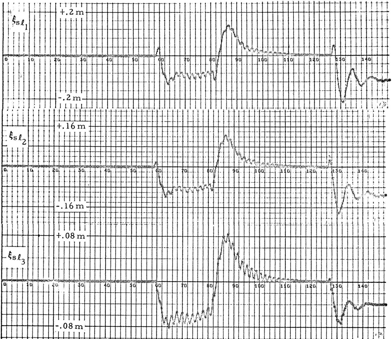
Figure 2-13c - Saturn V, S-IC Stage Response to  $\phi_c$  - Digital Nonlinear Filter ( $\omega_s = 96\text{ rad/sec}$ )
