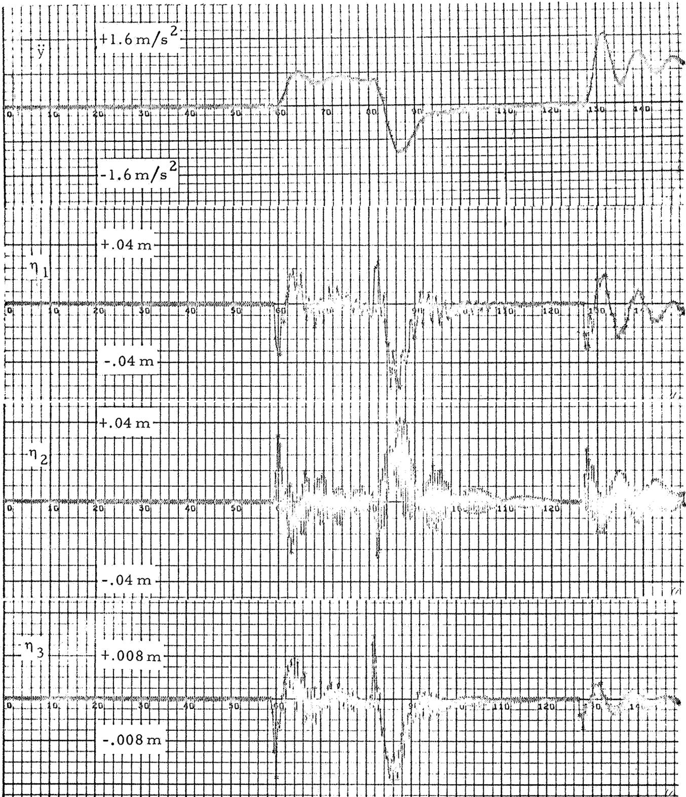
Figure 2-11b - Saturn V, S-IC Stage Response to  $\phi_c$  - Digital Nonlinear Filter ( $\omega_s = 24$  rad/sec).
