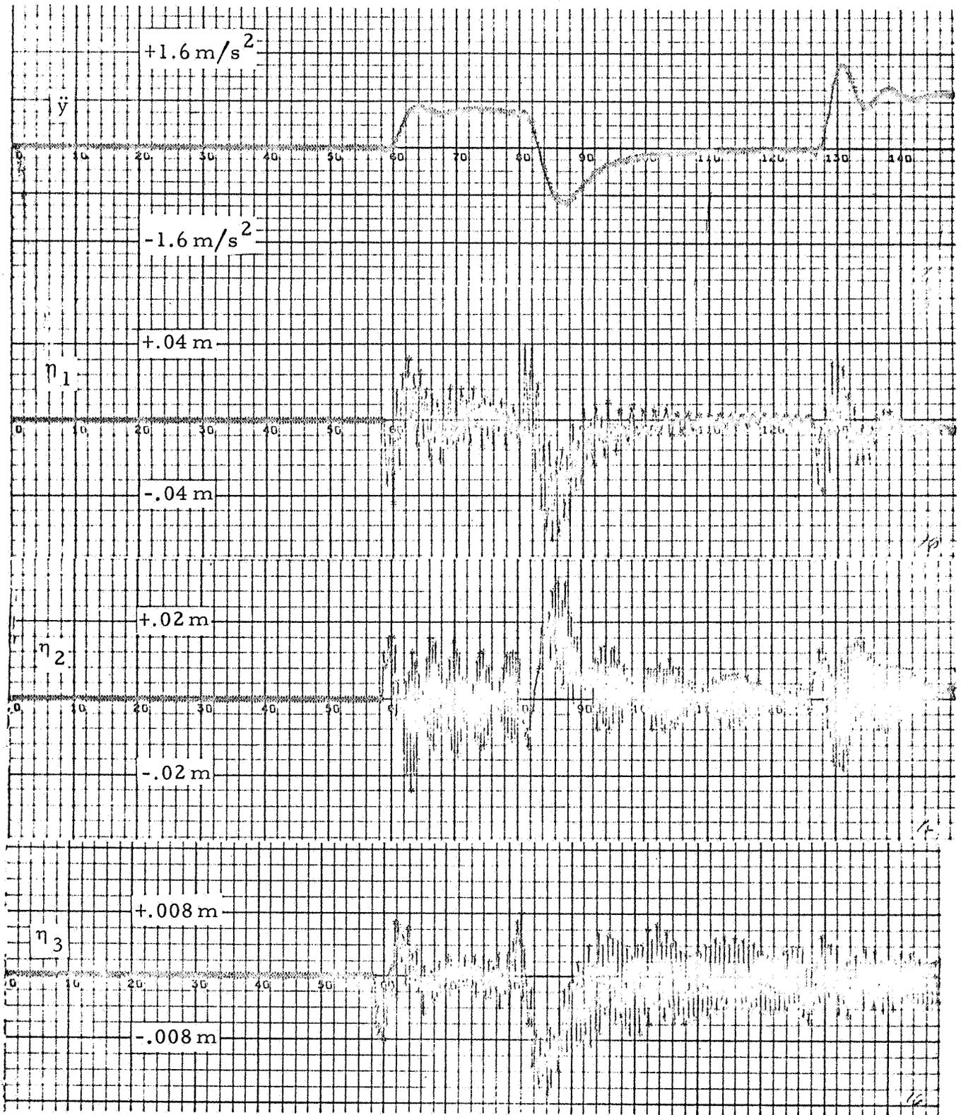
Figure 2-16b - Saturn V, S-IC Stage Response to  $\phi_c$  with all Bending Mode Damping Ratios Reduced by a Factor 10 - Digital Nonlinear Filter ( $\omega_s = 96$  rad/sec)
