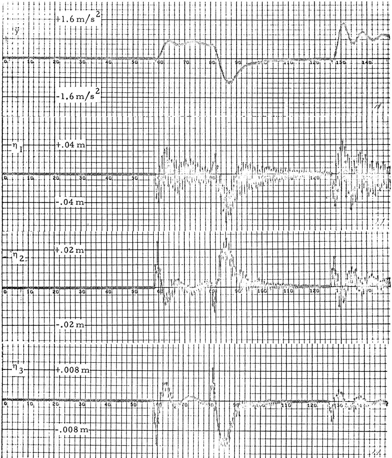
Figure 2-14b - Saturn V, S-IC Stage Response to  $\phi_c$  with all Bending Mode Signs Reversed - Digital Nonlinear Filter ( $\omega_s = 96$  rad/sec)
