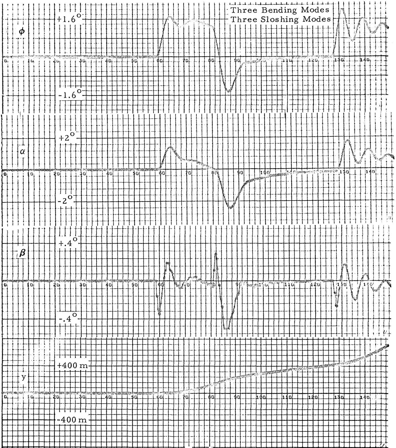
Figure 2-11a - Saturn V, S-IC Stage Response to  $\phi_c$  - Digital Nonlinear Filter ( $\omega_s = 24$  rad/sec).
