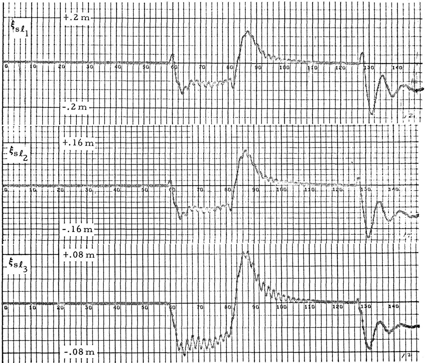
Figure 2-12c - Saturn V, S-IC Stage Response to  $\phi^c$  - Digital Nonlinear Filter ( $\omega_s = 48 \text{ rad/sec}$ )<sup>c</sup>
