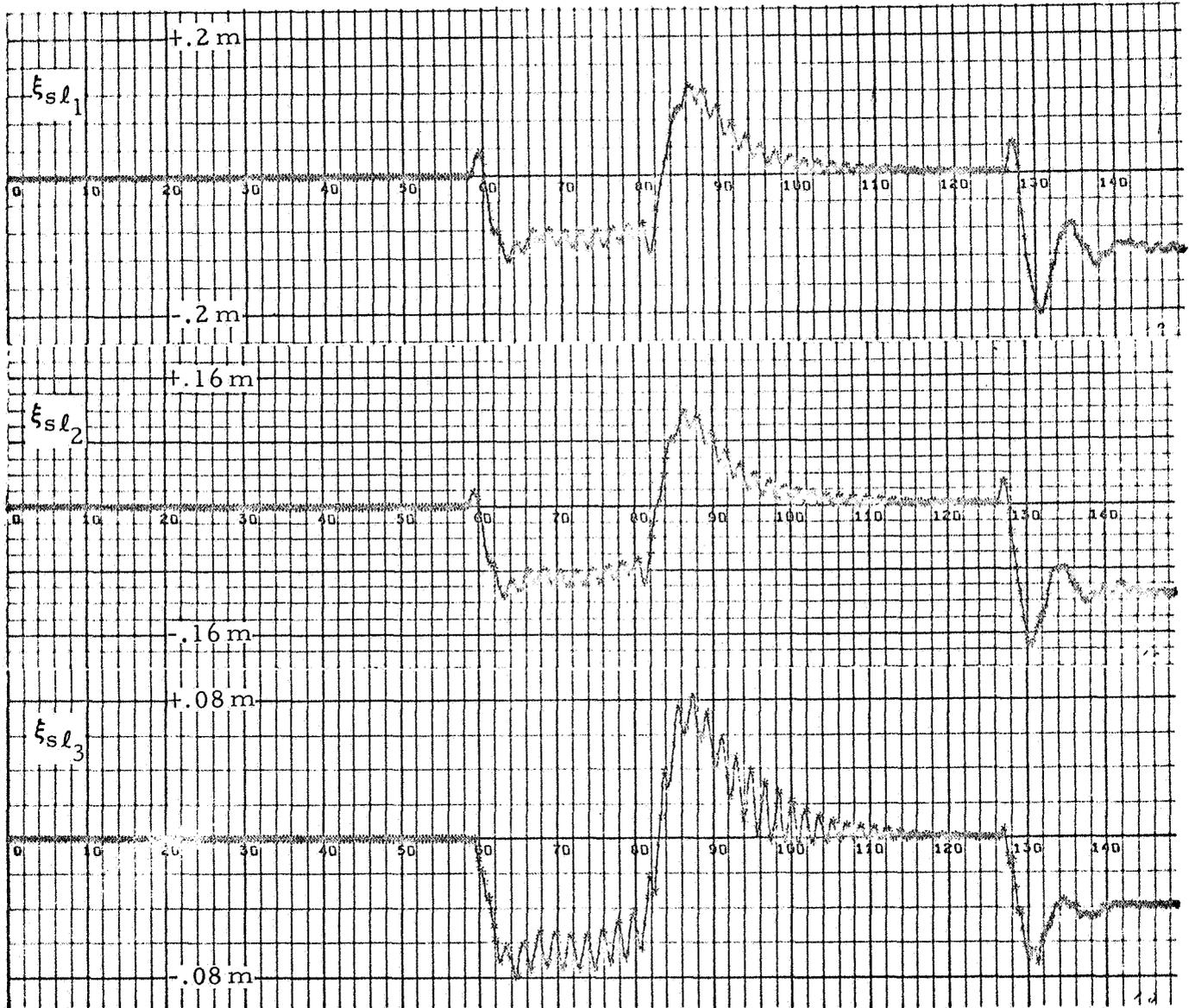
Figure 2-10c - Saturn V, S-IC Stage Response to  $\phi_c$ , Continuous Nonlinear Filter
