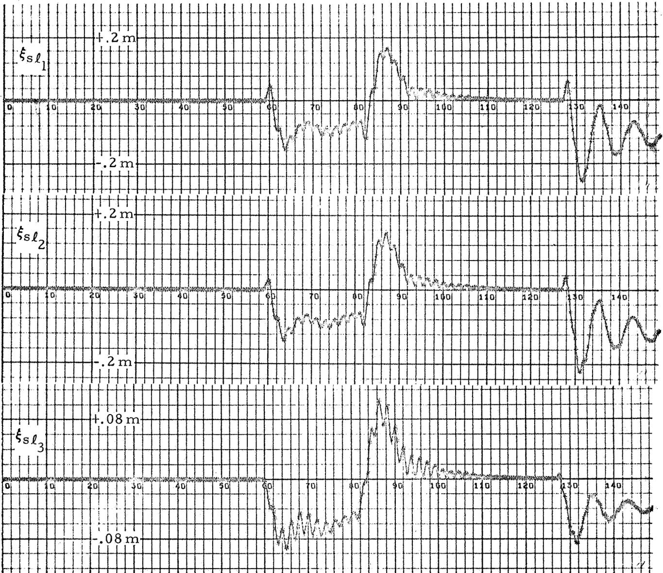
Figure 2-11c - Saturn V, S-IC Stage Response to  $\phi_c$  - Digital Nonlinear Filter ( $\omega_s = 24$  rad/sec).
