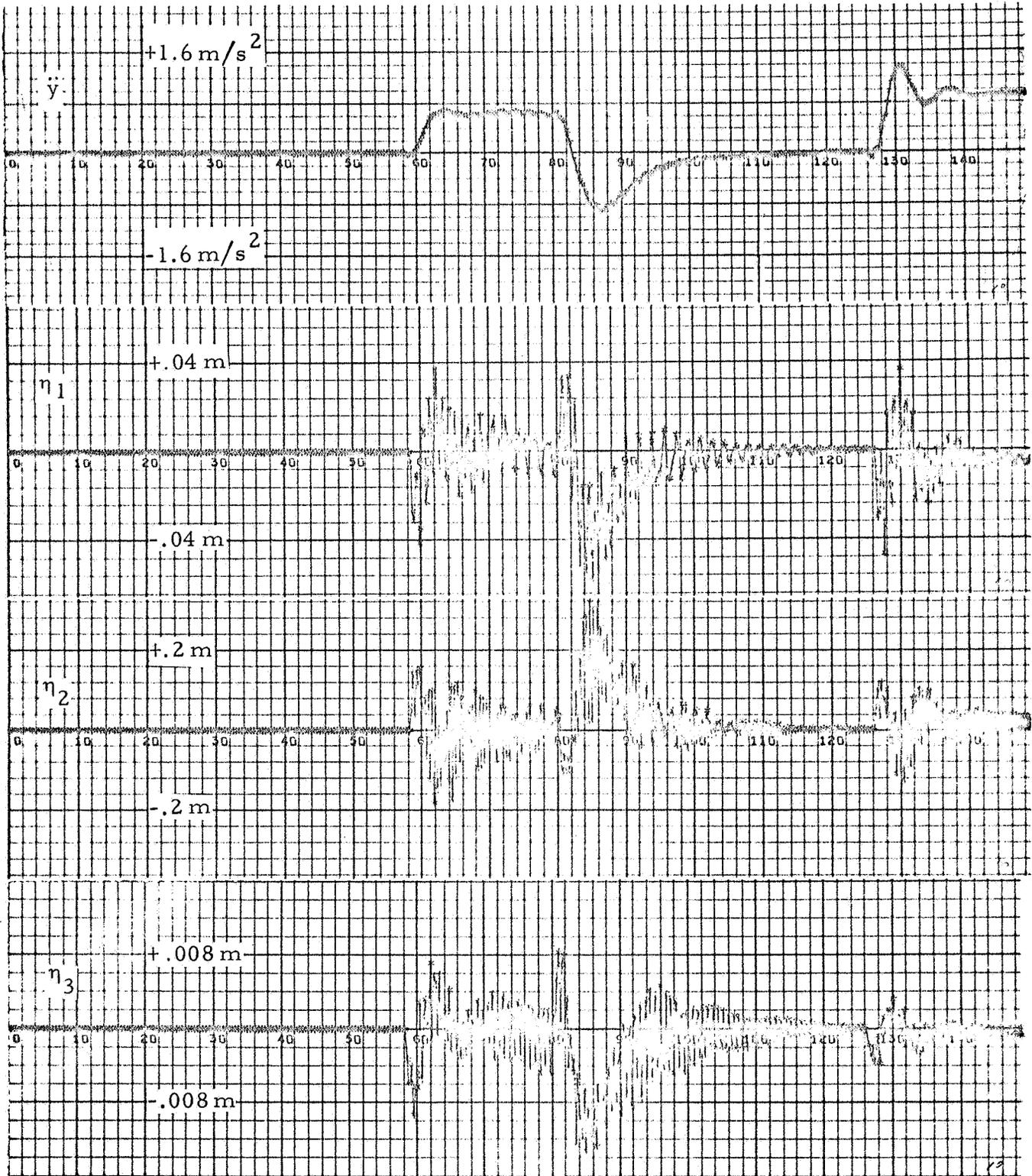
Figure 2-10b - Saturn V, S-IC Stage Response to  $\phi_c$ , Continuous Nonlinear Filter
