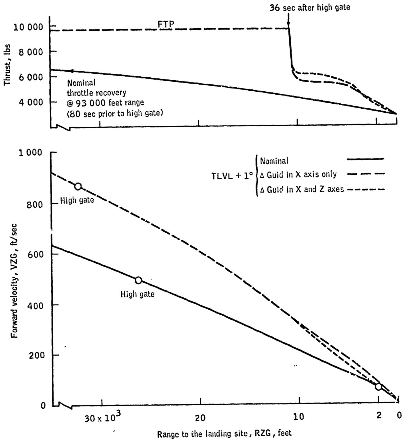
Figure 3. - Maintain desired forward approach speed with Delta horizontal guidance when throttle recovery occurs after high gate for TLVL + 1° condition.
