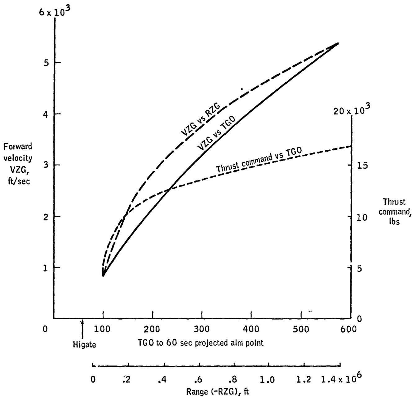
Figure 1. - Profiles considered for velocity control throttle logic.
