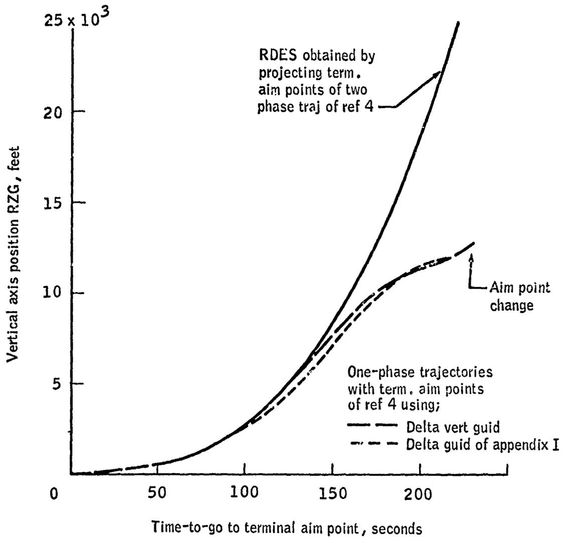
Figure 2. - A one-phase trajectory shaped to old high gate-low gate final approach with delta guidance.
