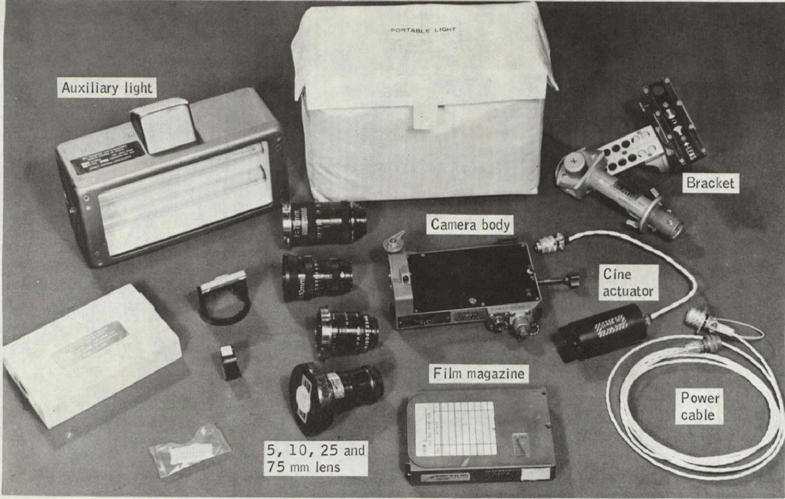
Figure A-22.- The 16-mm data acquisition camera system.
