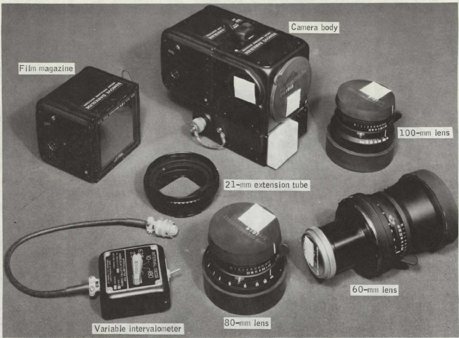
Figure A-24.- The 70-mm data acquisition camera system.
