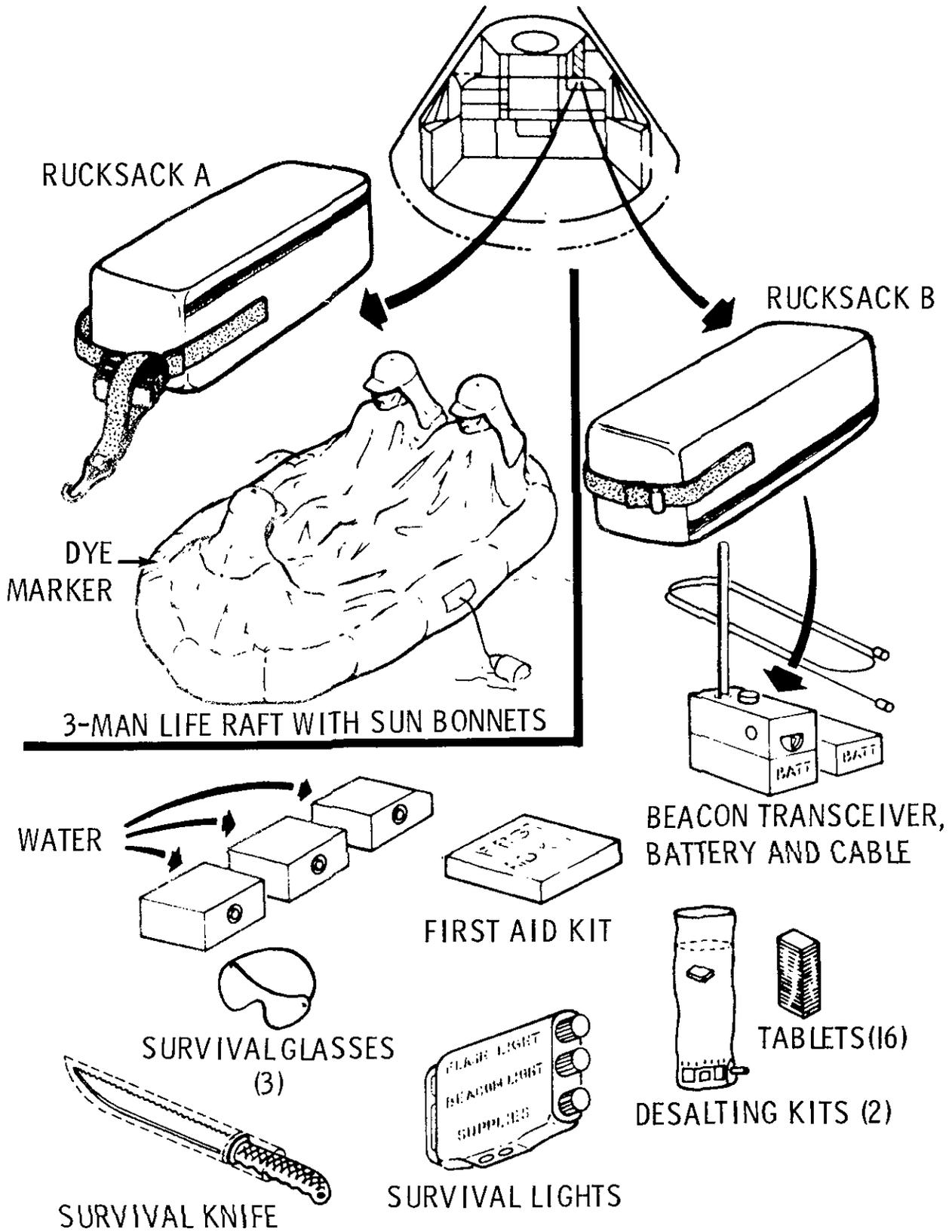
Rucksack No. 2: one three-man life raft with CO<sub>2</sub> inflater, one sea anchor, two sea dye markers, three sun-bonnets, one mooring lanyard, three manlines, and two attach brackets.
