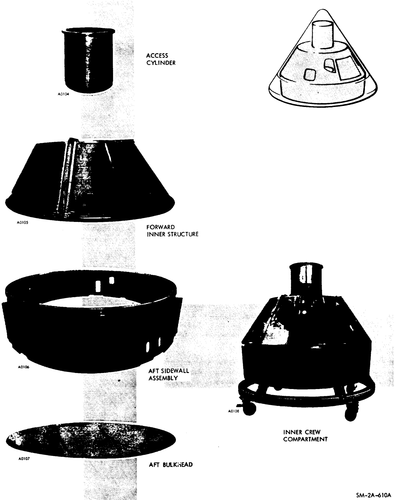
Figure 5-2. Command Module Inner Crew Compartment Structure
