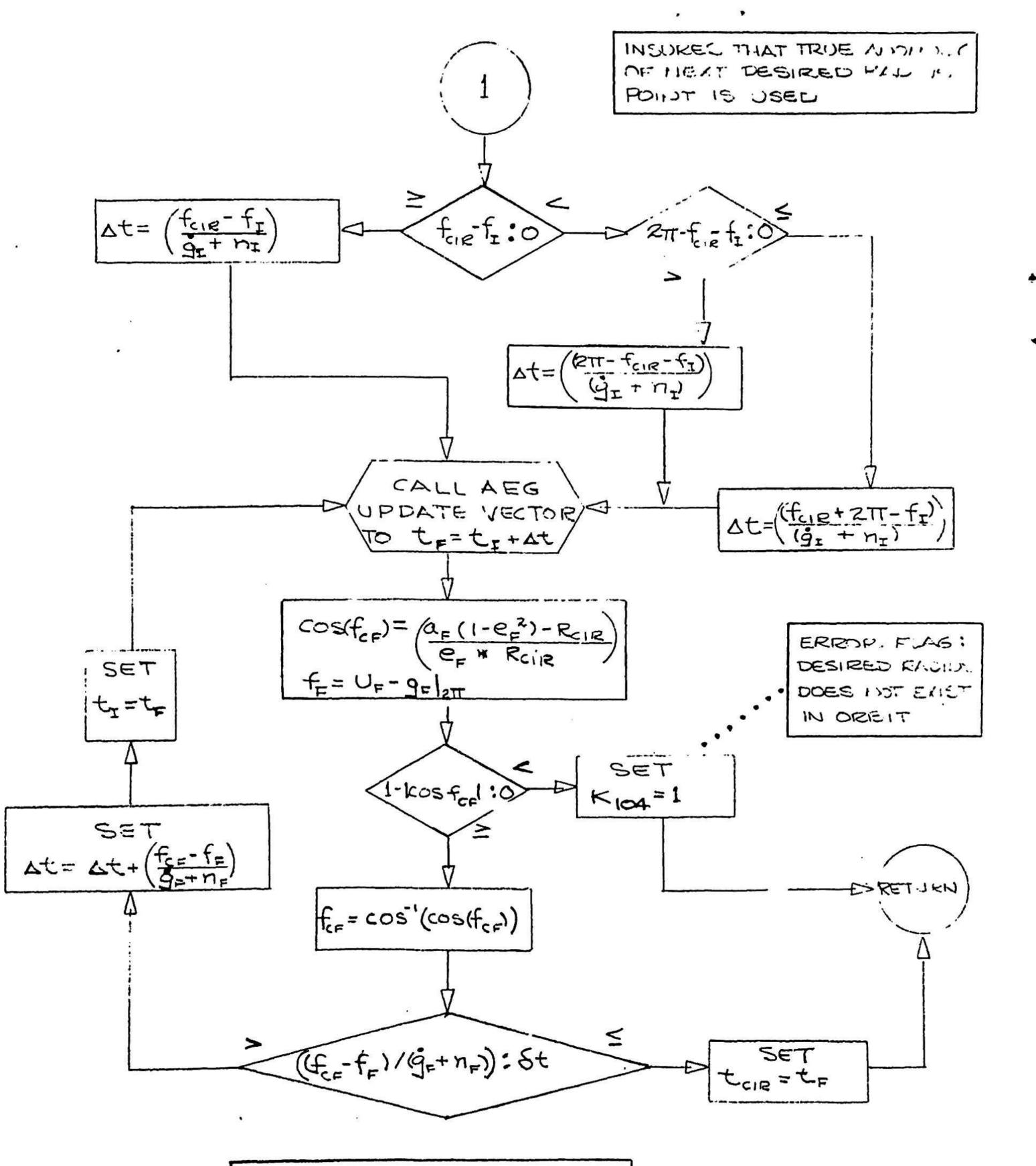
TIME OF ARRIVAL AT DESIRED RADIUS WITHIN A TIME TOLERANCE ST
