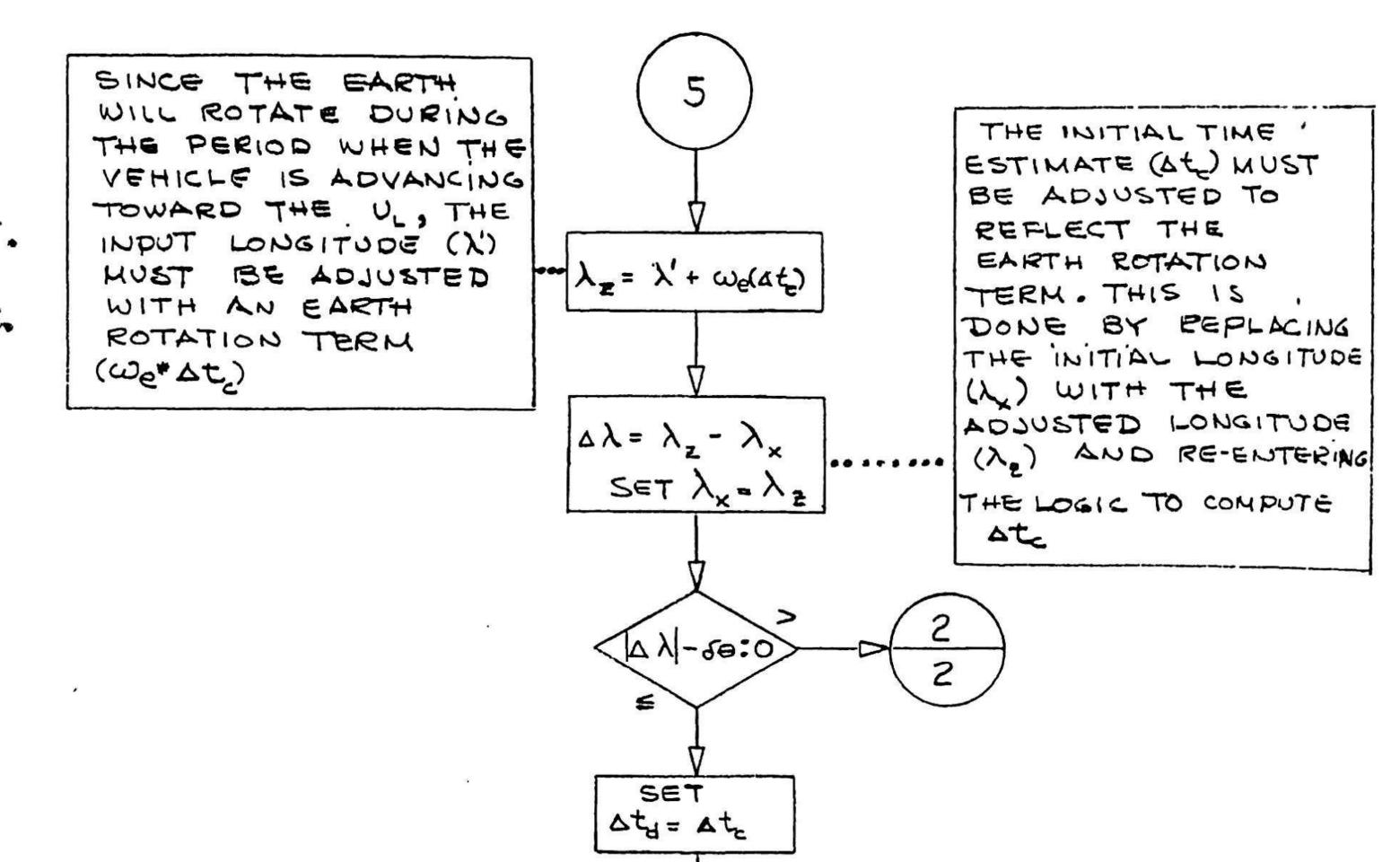
THE UL COMPUTED IN THE ABOVE CALL AEG - UP DATE ITERATION IS VECTOR TO the = (t + std) ITERATED UPON TO DETERMINE THE CORRECT TIME OF ARRIVAL AT THE ARSJMENT OF LATITUDE OF THE DESIRED SET UL-UE-St  $\Delta t_d = \Delta t_d + \left( \frac{U_L - U_F}{1 + F} \right)$ LCNGITUDE SET RETURN tLON = tF
