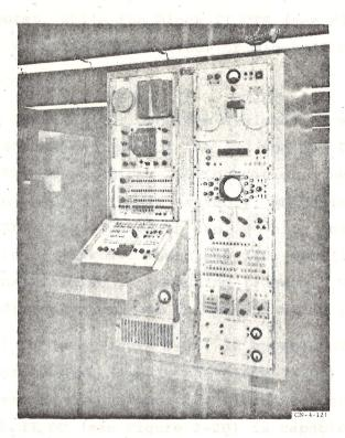
Figure 2-23 Block I(0) Computer Test Set
