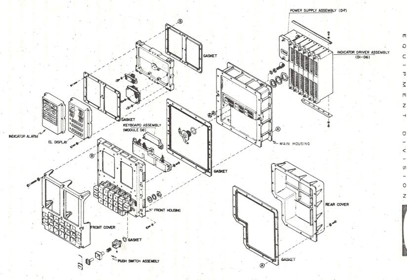
Figure 2-20 Block II DSKY (Exploded View)
