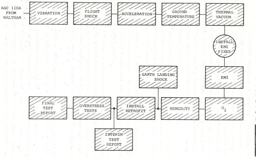
Figure 3-1 Block I(100) AGC 110A Qualification Test Sequence
