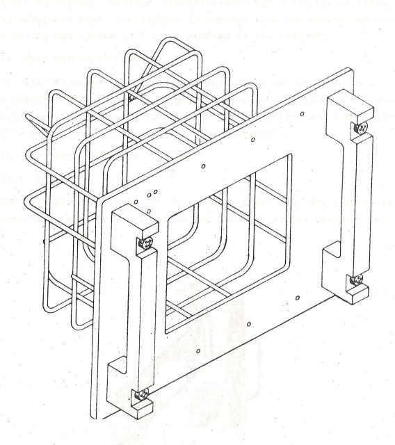
Figure 2-49 Block II DSKY Handling Fixture
