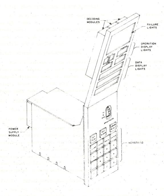
Figure 2-8 Navigation Panel Display and Keyboard (DSKY) BLOCK I(0)
