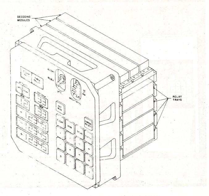
Figure 2-9 Main Panel Display and Keyboard (DSKY)
