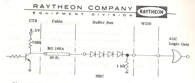
Figure 3-8 AGC Input and Noise Reduction Circuit Output Schematic
