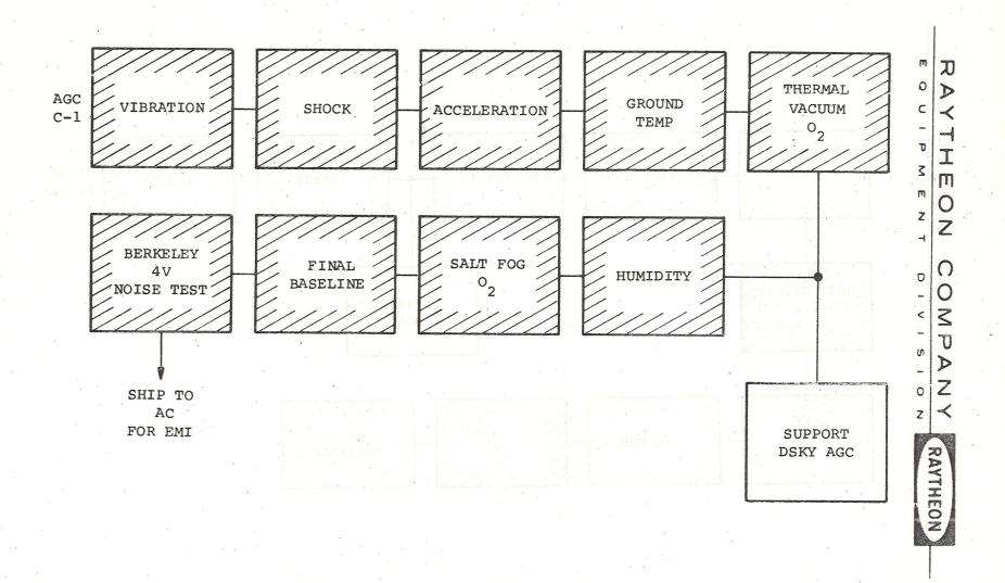
Figure 3-3 Block II AGC Qualification Test Program
