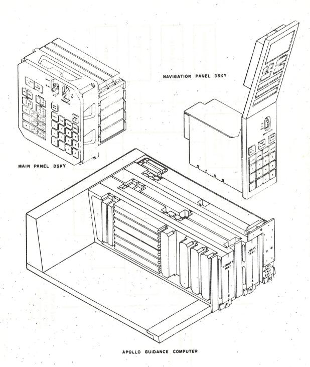
Figure 2-2 Computer Subsystem Equipment, Block I(O)
