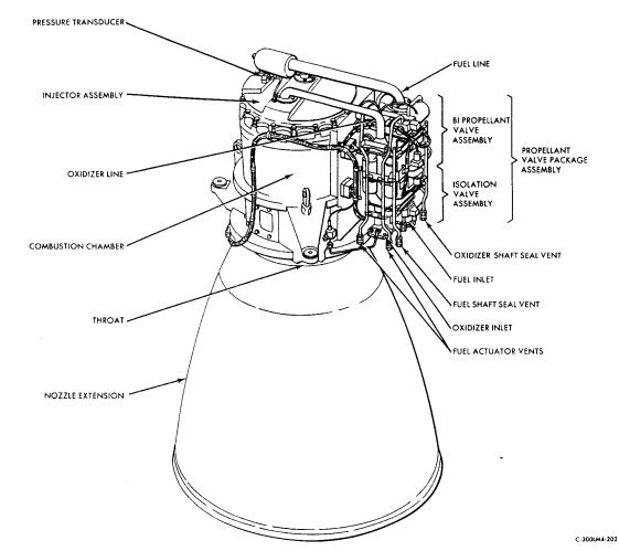
Figure 2.3-23. Ascent Engine Assembly
