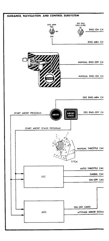
analog output of the DECA controls descent engine thrust. In the automatic mode, the thrust/translation controller assemblies (TTCA's) can be used by the astronauts to increase descent engine throttle (overriding the automatic throttle command); the TTCA's cannot be used, however, to decrease the throttle command. (Refer to paragraph 2.3.3.3.1.) In the manual throttle mode, the astronauts have complete control over descent engine thrust.
