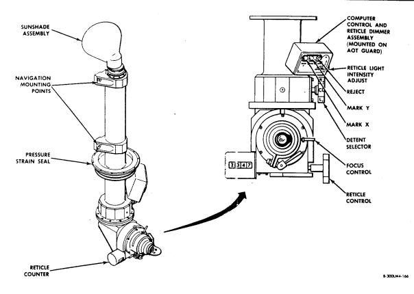
Figure 2.1-4. Alignment Optical Telescope
