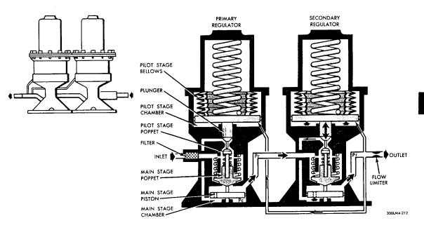
Figure 2.4-10. Helium Pressure Regulator Assembly
