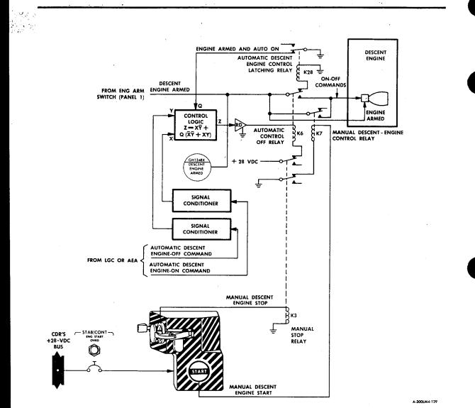
Figure 2.1-51. Descent Engine Control Assembly - Engine Control Diagram
