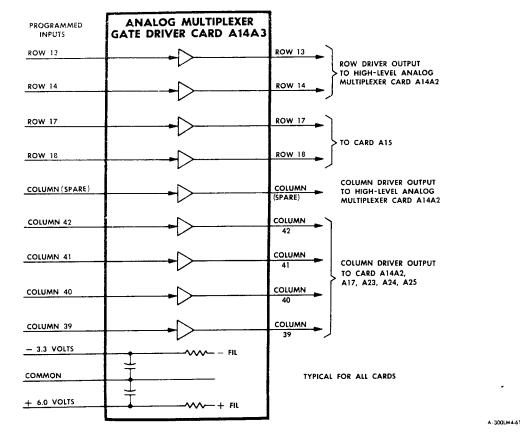
Figure 2.9-5. Typical Analog Multiplexer Driver Card - Simplified Logic Diagram
