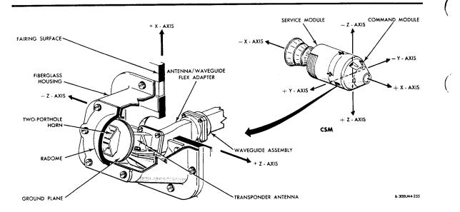
Figure 2.2-14. Transponder Antenna Assembly
