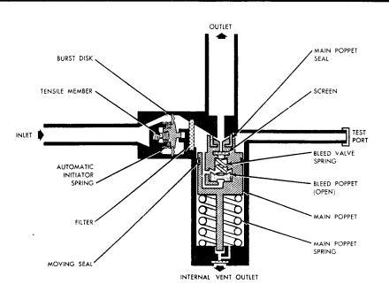
Figure 2.3-22. Ascent Propulsion Section - Relief Valve Assembly
