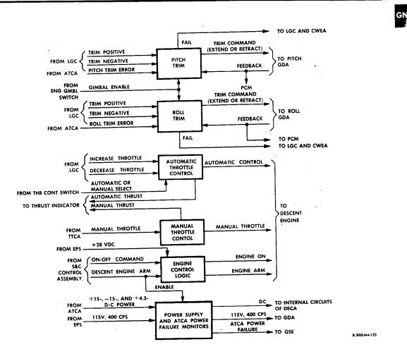
Figure 2.1-48. Descent Engine Control Assembly - Simplified Block Diagram
