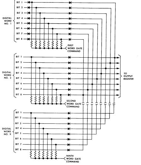
Figure 2.9-10. Digital Multiplexer - Logic Diagram
