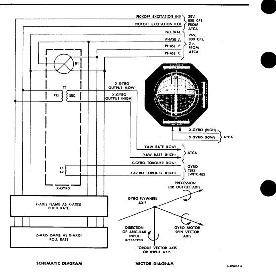
Figure 2.1-47. Rate Gyro Assembly - Schematic and Vector Diagram
