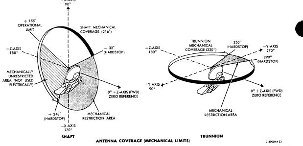
Figure 2.2-6. Rendezvous Radar - Antenna Orientation No. II
