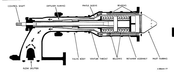
Figure 2.3-13. Flow Control Valve
