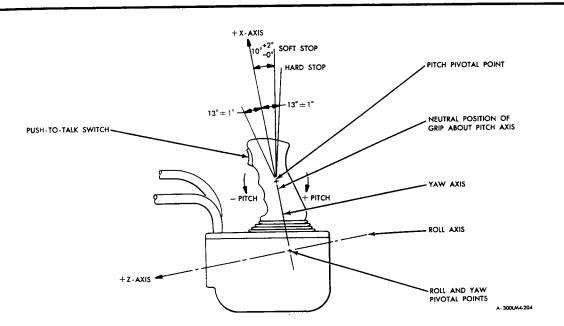
Figure 2.1-40. ACA - Angular Displacements
