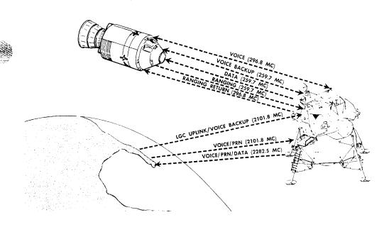
Figure 2.7-4. In-Flight Communications
