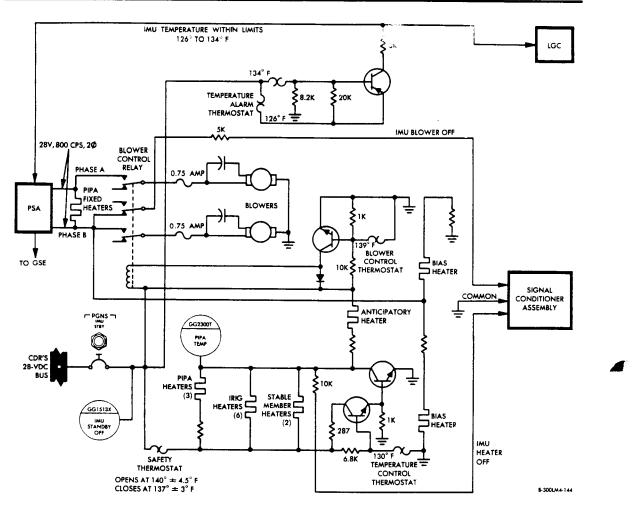
Figure 2.1-25. IMU Temperature Control
