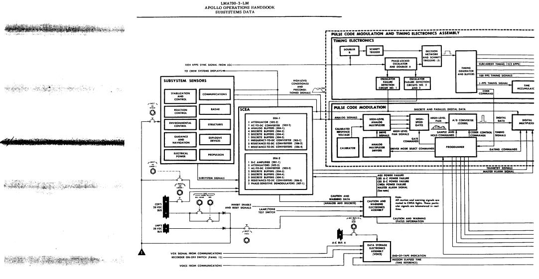
Figure 2.9-2. Instrumentation Subsystem - Overall Functional Block Diagram
