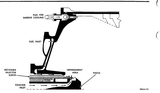
Figure 2.3-14. Variable-Area Injector - Quarter Section
