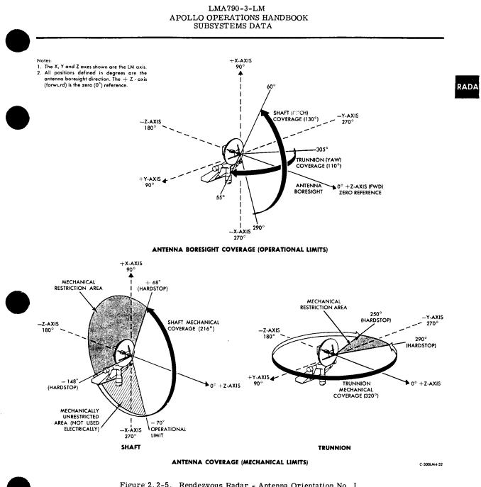
Figure 2.2-5. Rendezvous Radar - Antenna Orientation No. I
