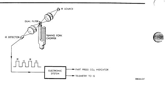
Figure 2.6-13. Carbon Dioxide Partial Pressure Sensor - Functional Schematic
