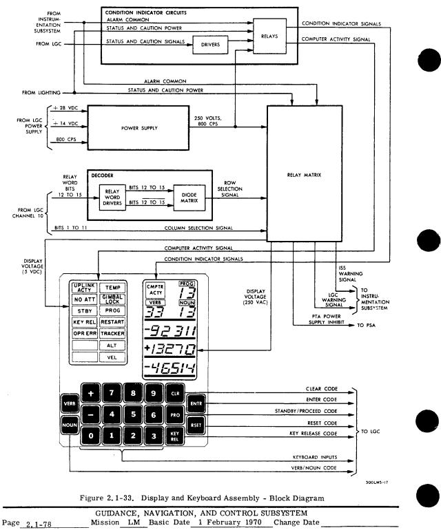
Relay Package. The relay package consists of a relay matrix and decoding circuits.
