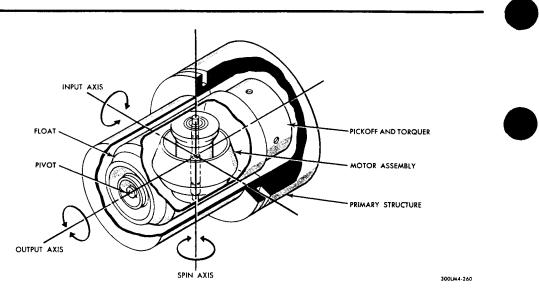
Figure 2.1-35. Abort Guidance Section - Gyro Assembly
