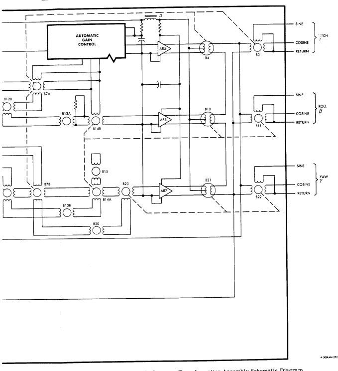
Figure 2.1-56. Gimbal Angle Sequence Transformation Assembly Schematic Diagram
