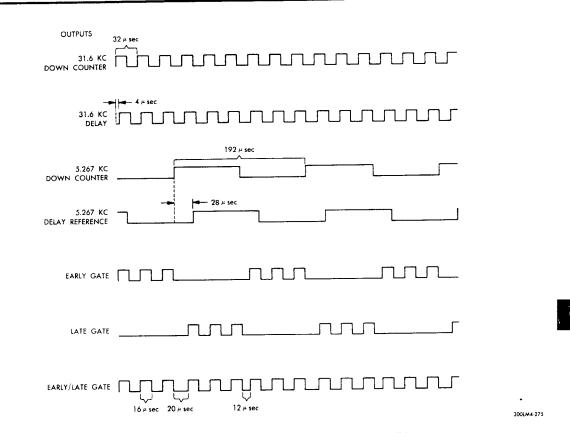
Figure 2.7-20. Ranging Tone Transfer Assembly - Timing Diagram
