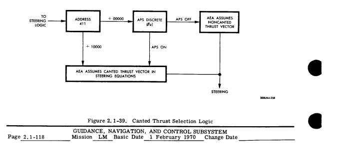
Descent or Ascent Engine Burn. To prepare for an engine burn under AGS control, the following conditions are required:
