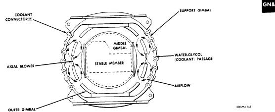
Figure 2.1-26. IMU Forced Convection Cooling
