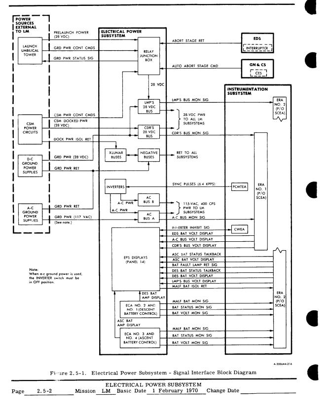
translunar bus. (Ground return in the LM is generally accomplished through the metal structure, whereas ground return in the CSM is isolated from the CSM structure.) Before LM-CSM separation, all LM internally supplied electrical power (ac and dc) is restored.
