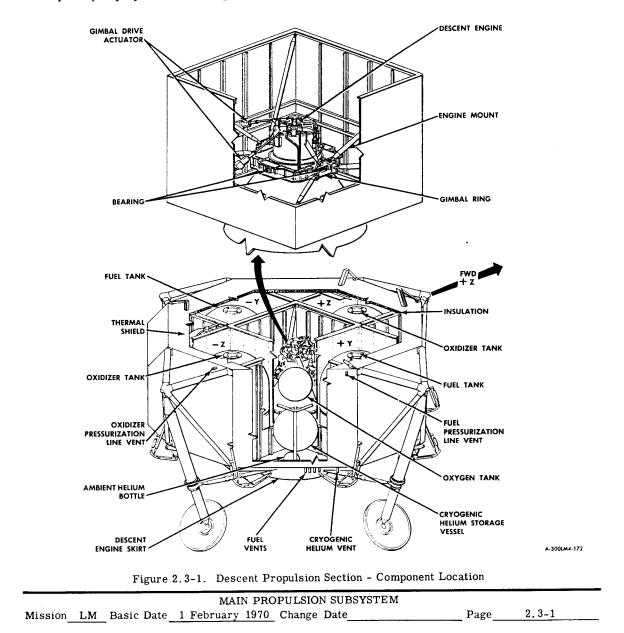
Both propulsion sections use identical hypergolic propellants: a 50-50 mixture, by weight, of hydrazine (N2H4) and unsymmetrical dimethylhydrazine (UDMH) as the fuel; nitrogen tetroxide (N2O4), as the oxidizer. The injection ratio of oxidizer to fuel is approximately 1.6 to 1, by weight.
