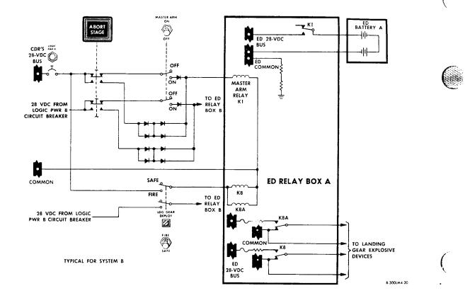
Figure 2.8-6. Landing Gear Deployment - Simplified Schematic Diagram
