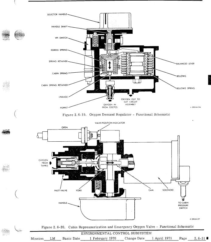
maintain cabin pressure at 3.5 psia for at least 2 minutes, allowing the astronauts to return to a closedsuit environment. The valve is controlled by a three-position handle on the oxygen control module.
