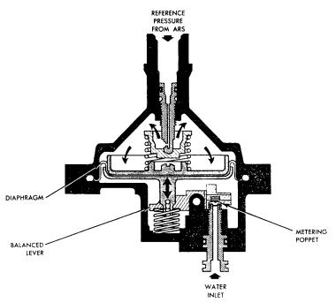
Figure 2.6-23. Water Pressure Regulator - Functional Schematic
