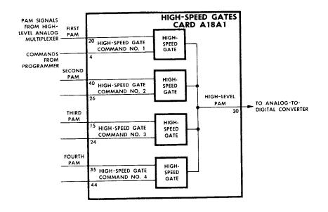
Figure 2.9-7. High-Speed Gates - Logic Diagram
