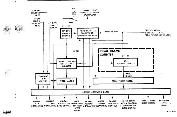
Figure 2.9-9. Programmer - Block Diagram
