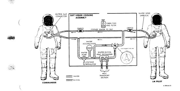
Figure 2.6-6A. Suit Liquid Cooling Assembly - Schematic Flow Diagram
