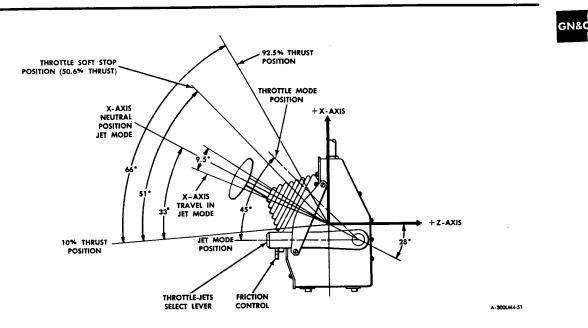
Figure 2.1-42. TTCA - Angular Displacements
