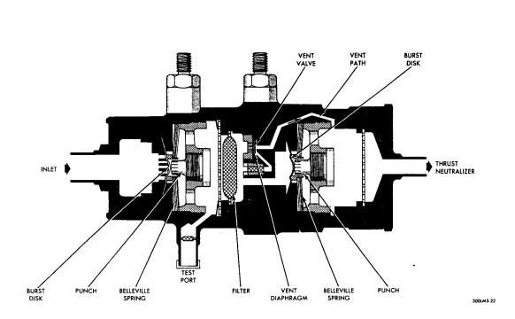
Figure 2.3-7A. Cryogenic Helium Storage Vessel - Burst Disk Assembly
