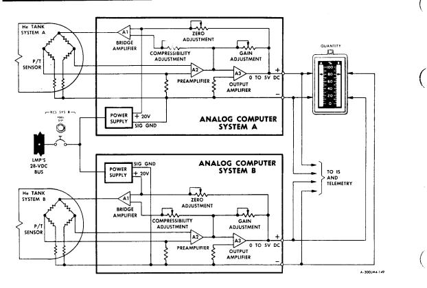
Figure 2.4-5. Propellant Quantity Measuring Device
