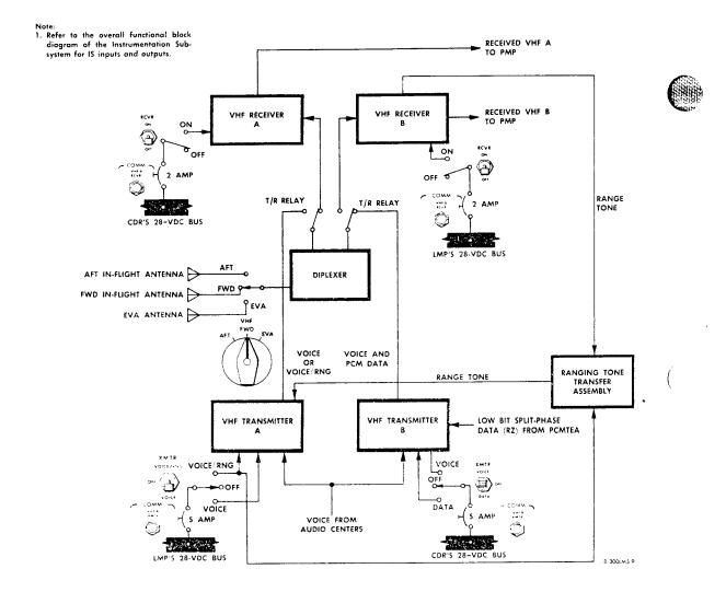
Figure 2.7-9. VHF Equipment - Block Diagram
