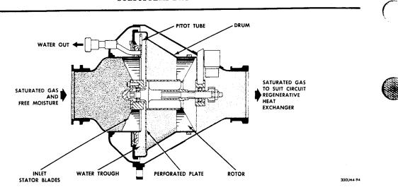
Figure 2.6-11. Water Separator - Functional Schematic
