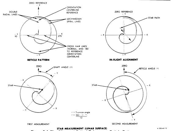
Figure 2.1-31. Alignment Optical Telescope - Reticle Pattern
