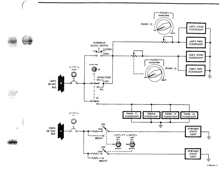
Figure 2.10-4. Floodlighting and Utility Lights - Simplified Diagram
