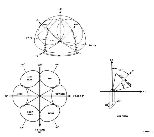
Figure 2.1-12. Alignment Optical Telescope Axes
