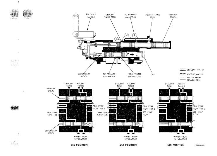
Figure 2.6-22. Water Tank Selector Valve - Functional Schematic
