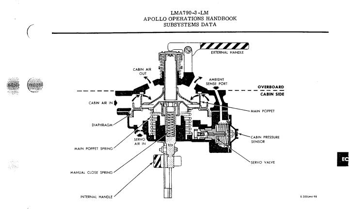
Figure 2. 6-21. Cabin Relief and Dump Valve - Functional Schematic
