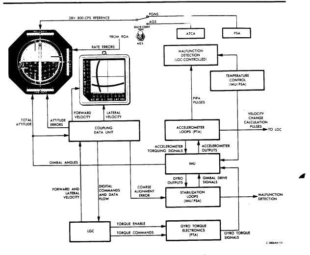
Figure 2.1-22. Inertial Subsection - Functional Diagram
