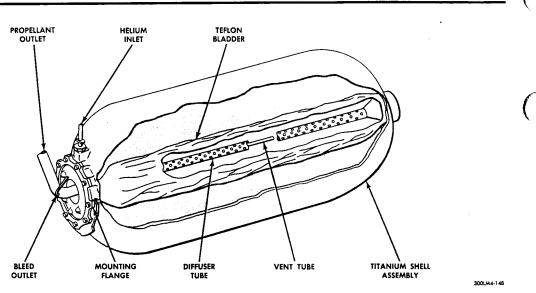
Figure 2.4-12. Propellant Tank Assembly
