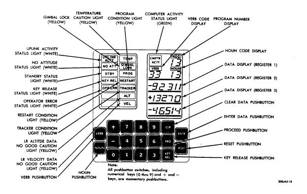
Figure 2.1-5. Display and Keyboard Assembly
