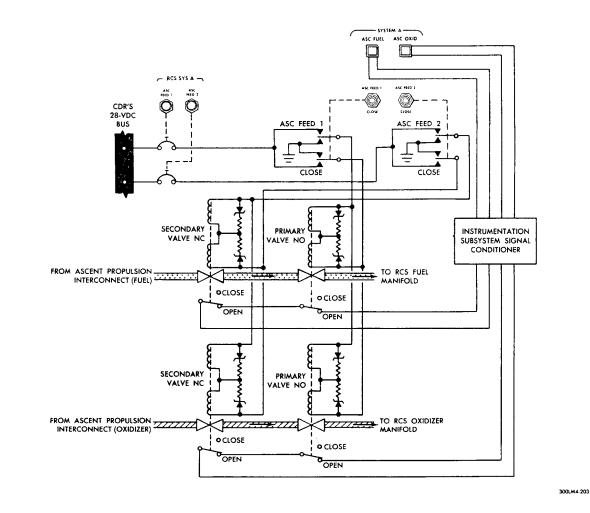
Figure 2.4-4. RCS System A - Ascent Feed Interconnect Valve Arrangement (Shown with Secondary Valves in Open Position)
