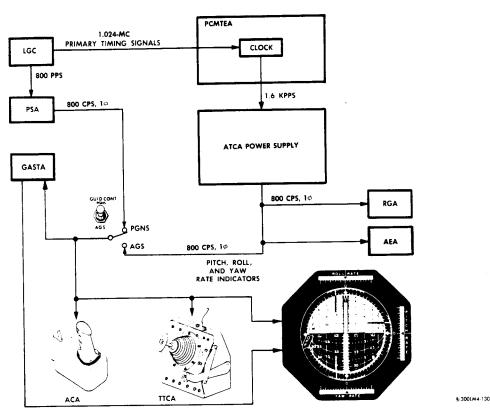
Figure 2.1-21. 800-cps Synchronization Loop
