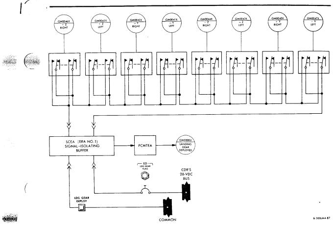
Figure 2.8-7. Landing Gear Switches - Schematic Diagram
