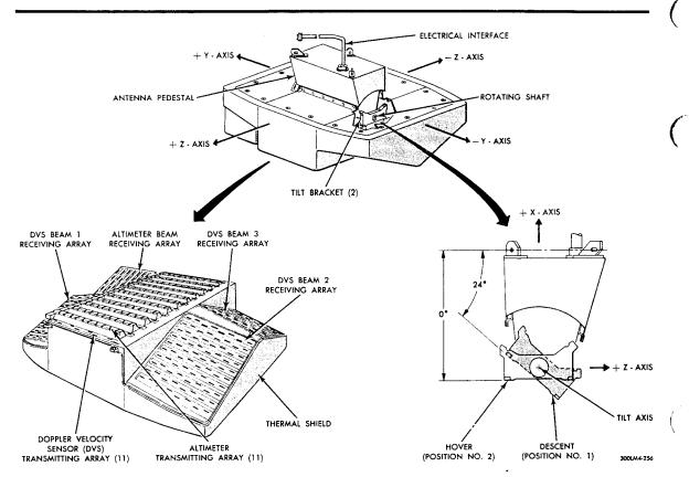
Figure 2.2-15. Landing Radar Antenna Assembly
