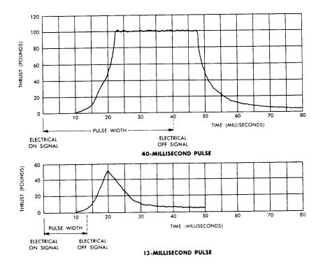
Figure 2.4-8. TCA Firing - Thrust Versus Time
