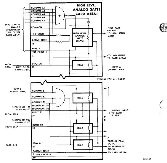
Figure 2.9-6. High-Level Analog Multiplexer Card - Simplified Logic Diagram
