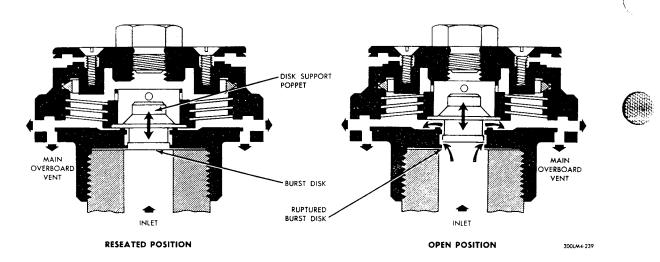
Figure 2.6-18. Burst Diaphram Assembly - Functional Schematic
