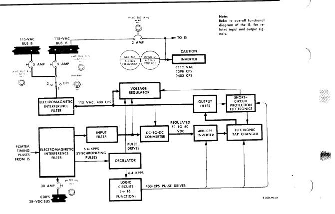
Figure 2.5-15. Inverter No. 1 - Block Diagram
