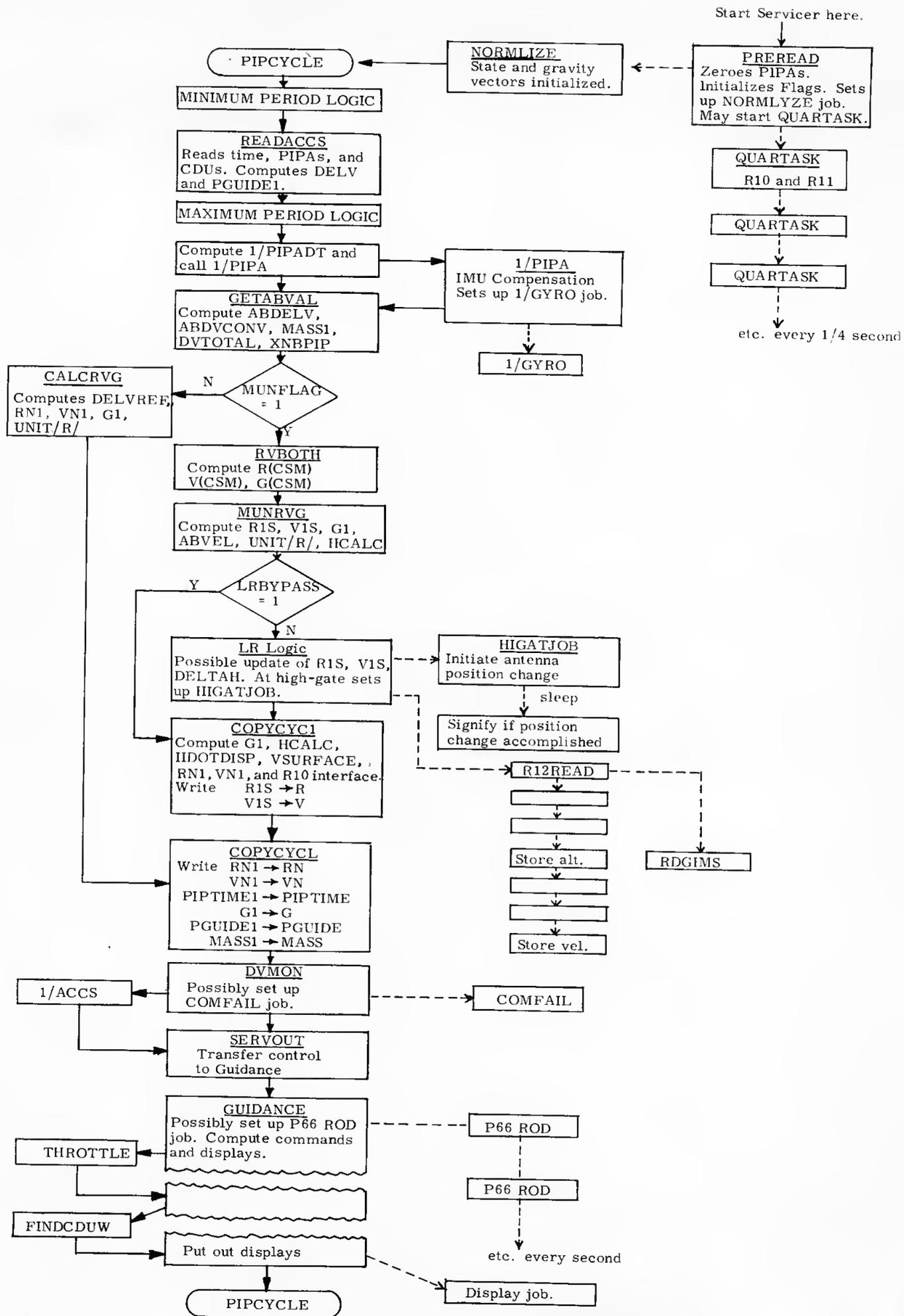
PIPCYCLE begins the Servicer cycle. NORMLIZE, the Servicer initialization routine and lead in of the Servicer job (set up by PREREAD which is called by the TIG -30 task of BURNBABY) falls through to PIPCYCLE. And it is to PIPCYCLE that Guidance returns when it finishes. But PIPCYCLE is just a tag and a restart point.
