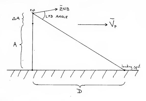
The top of the triangle is at the commander's eye. Note that altitude is shown in two segments. Since LGC altitude applies to the LR antenna,  $\Delta A$  is the distance between the antenna and the eye, approximated by the body X-axis difference, roughly 5 meters. D is the horizontal distance the spacecraft will travel while braking to zero horizontal velocity.  $\overline{Z}NB$  of course is the LM Z-axis.
