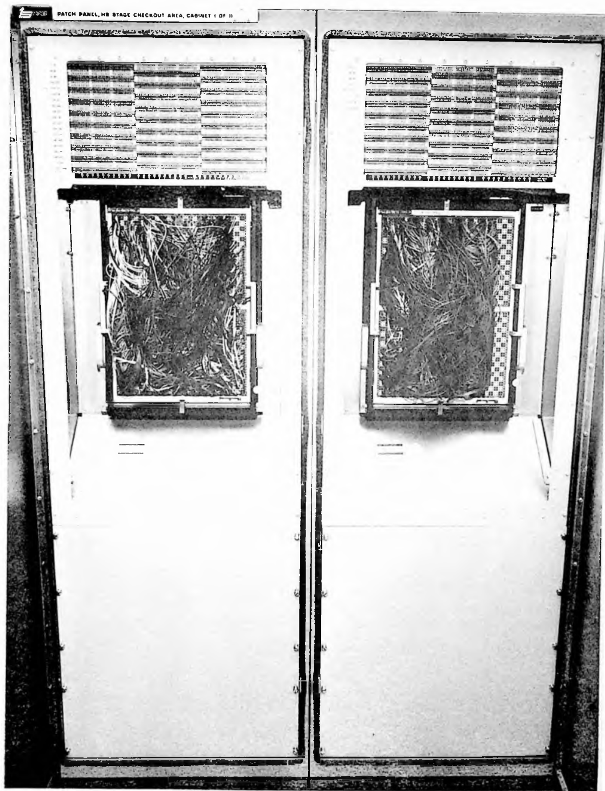
SSC007565 Figure 5-26. HB-VCO-2 Stage Checkout Area Patch Panel Distribution Box (DSV-4B-146)
