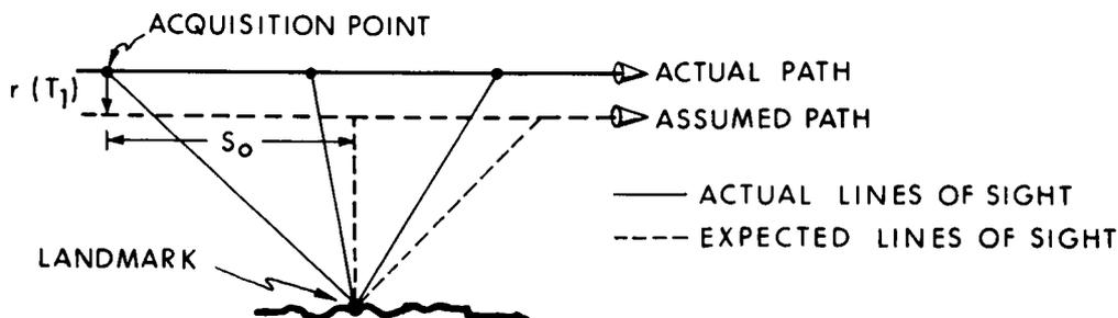
Fig. V-9 Tracking with an Erroneous Vehicle or Landmark Altitude
