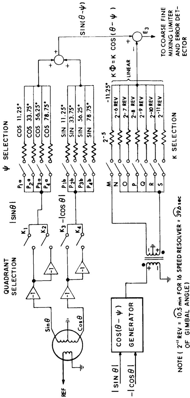
Fig. IV-25 Selection Logic - 16 Speed Resolver Digitizing Loop
