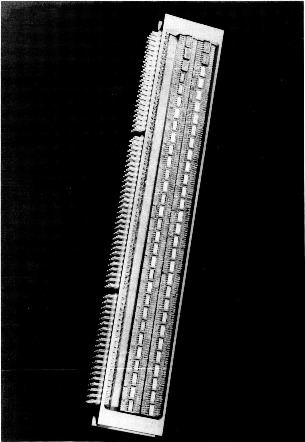
Fig. VI-7 Logic Module Containing 120 Microcircuit Units
