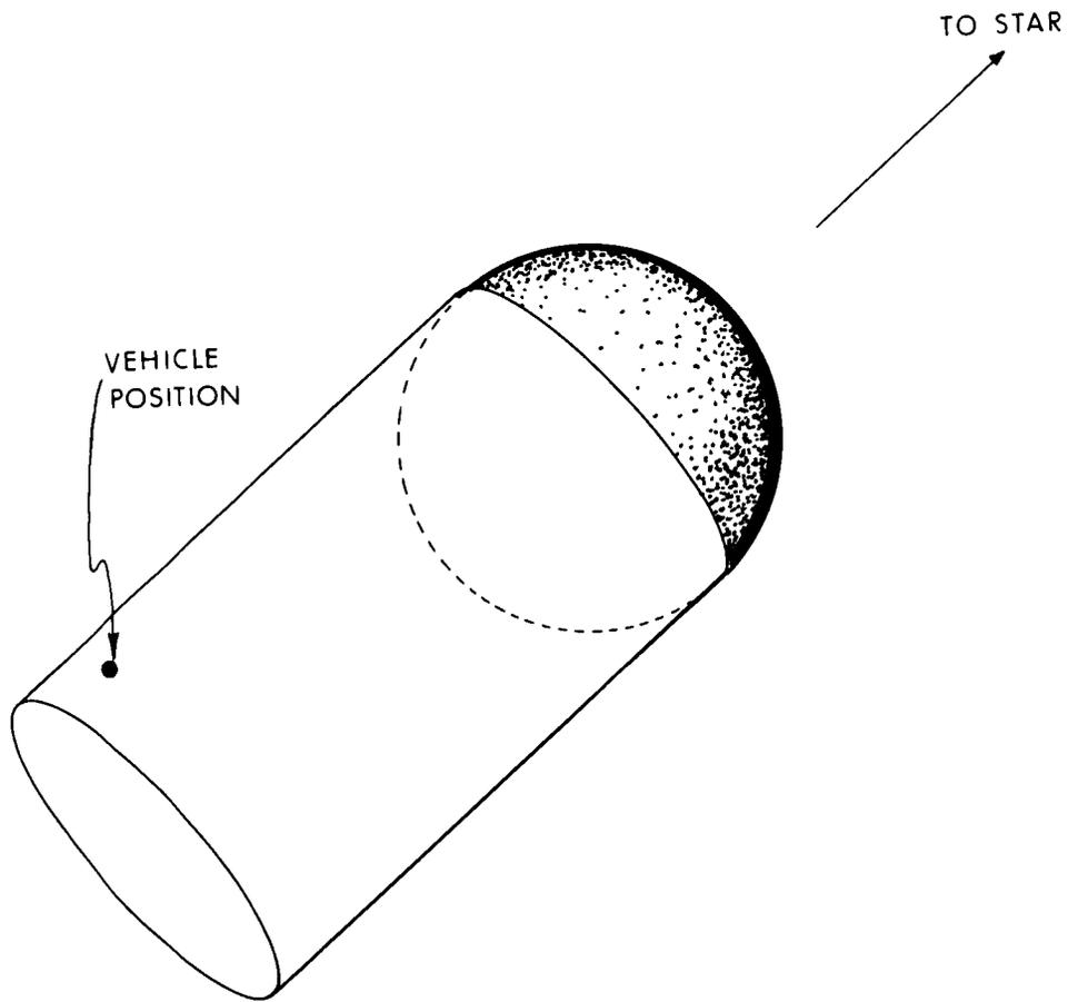
Fig. V-23 Star Occultation Measurement Geometry
