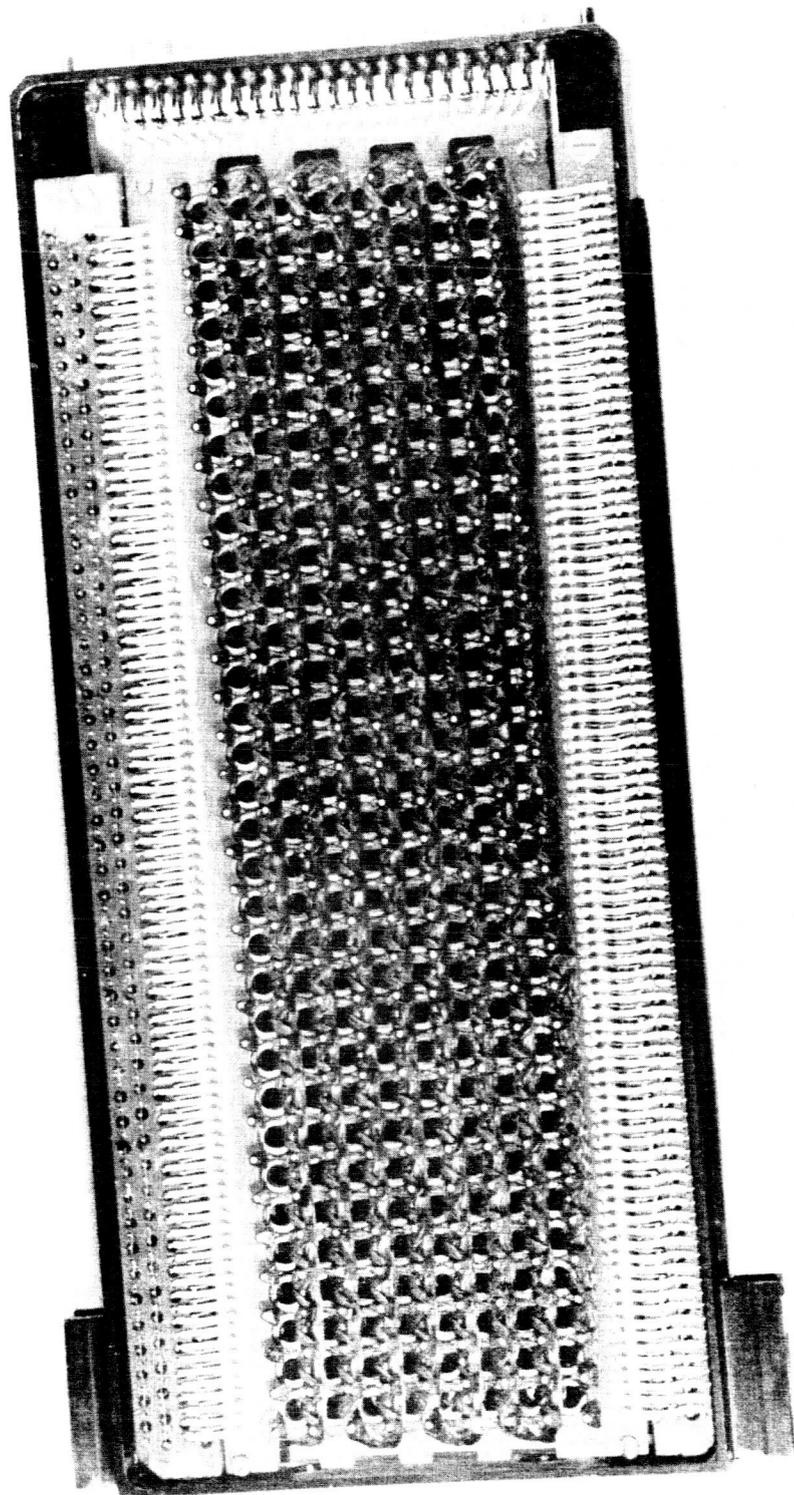
Fig. VI-16 AGC Core Rope Module
