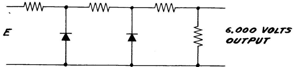
The second stage is chosen for a voltage where the temperature coefficient of the diode is nearly zero. This is slightly greater than 6 volts which is the point at which the temperature coefficient changes sign. The resistor divider network on the output is the normalization of the PVR to 6,000 volts. Voltage deviations of the PVR are less than 10 ppm/year with changes due to temperature less than 3 ppm/C<sup>o</sup>. This then forms the major portion of the constant current loop.
