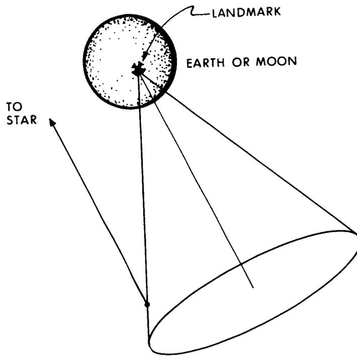
Fig. V-18 Star Landmark Measurement Geometry
