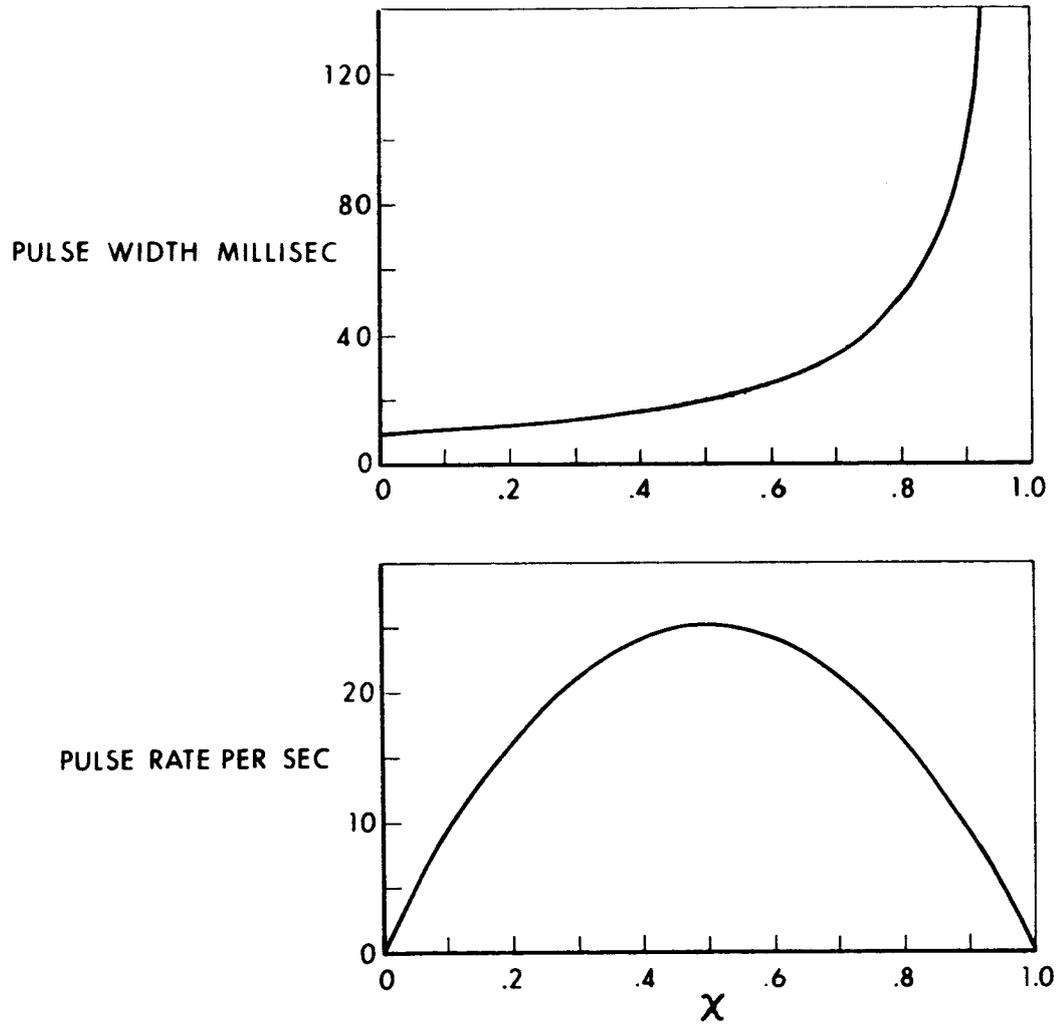
Fig. VII-22 Performance of the Pulse Ratio Modulator
