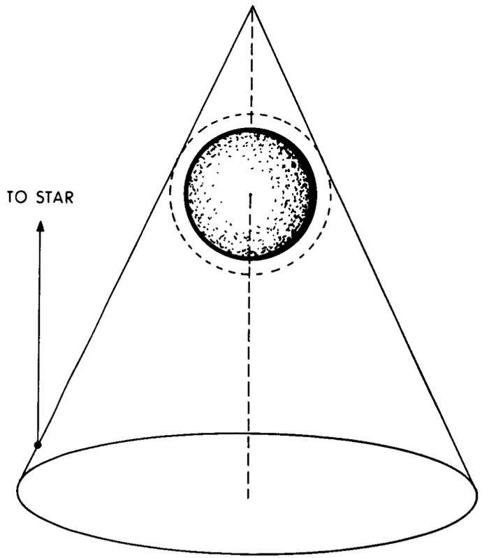
Fig. V-21 Star Horizon Measurement Geometry
