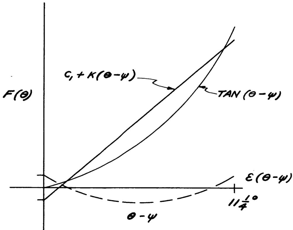
In addition, a bias is added to further reduce the errors over the entire range of linear interpolation. This results in a system whose errors are within the predicted errors.
