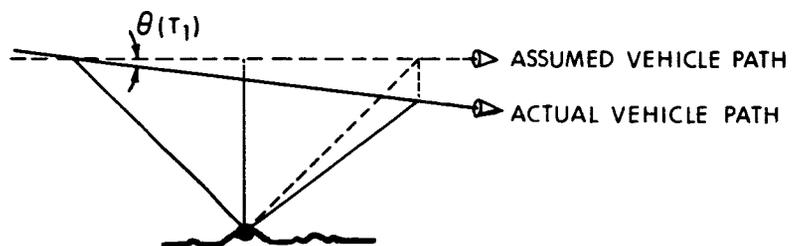
Figure V-12 Tracking with an Erroneous Range Error
