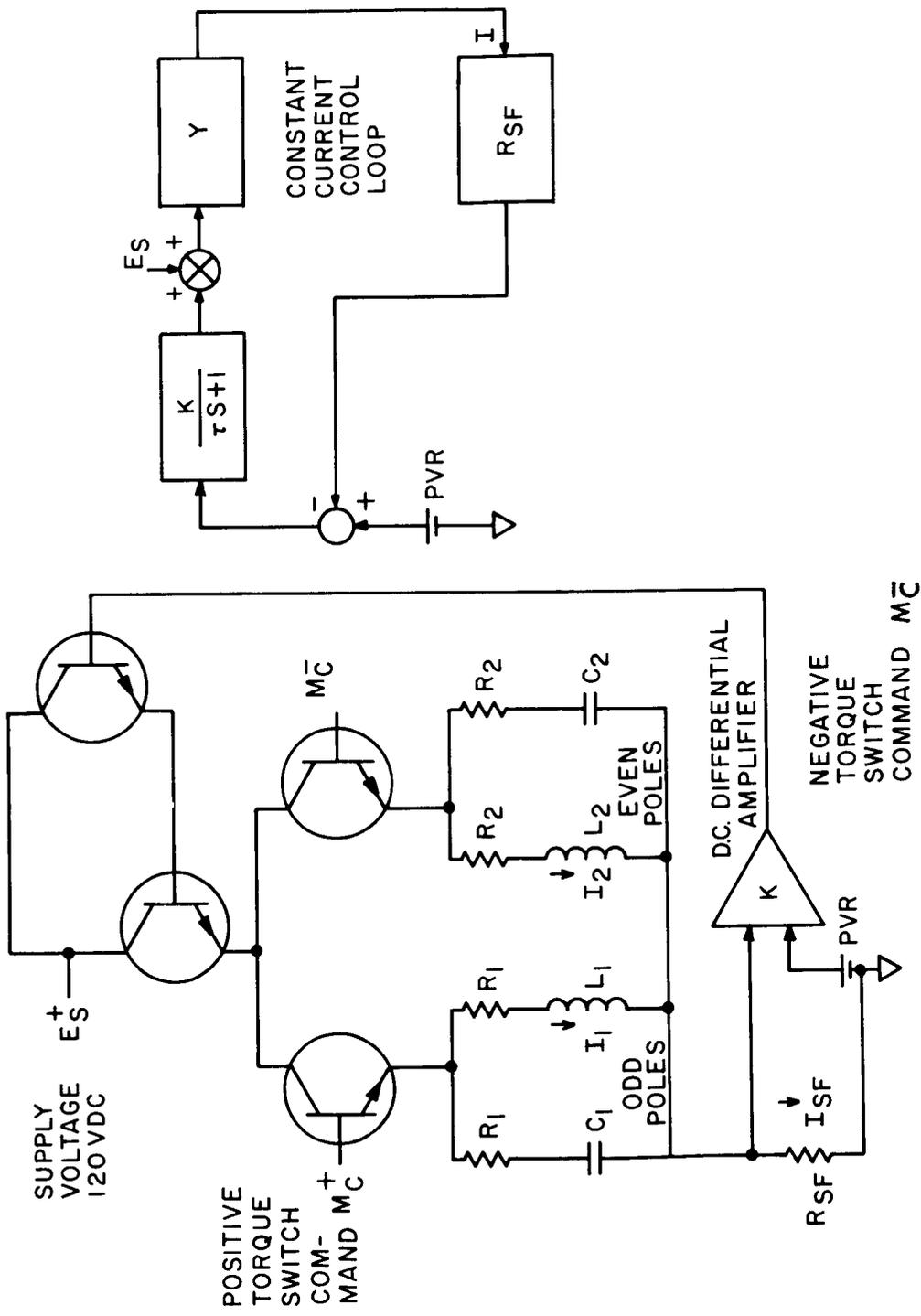
Fig. IV-22 Current Control and Current Switch
