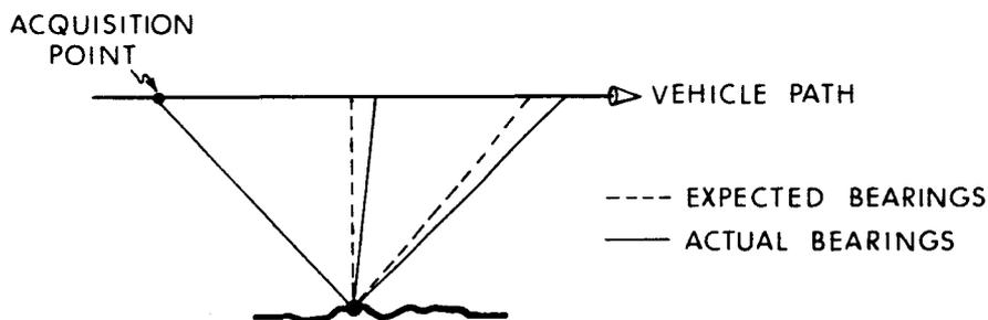
Fig. V-10 Tracking with an Erroneous Velocity Along Range
