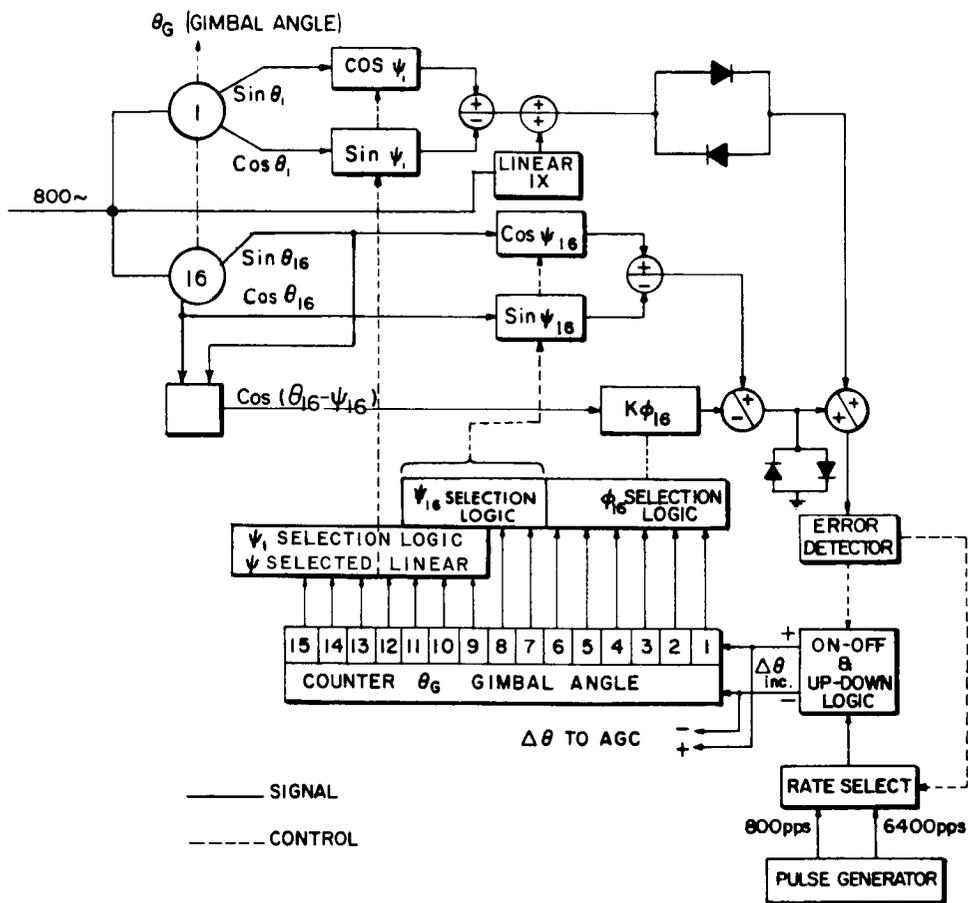
Fig IV-26 Coarse-Fine Mixing (1 and 16 Speed Resolver)
