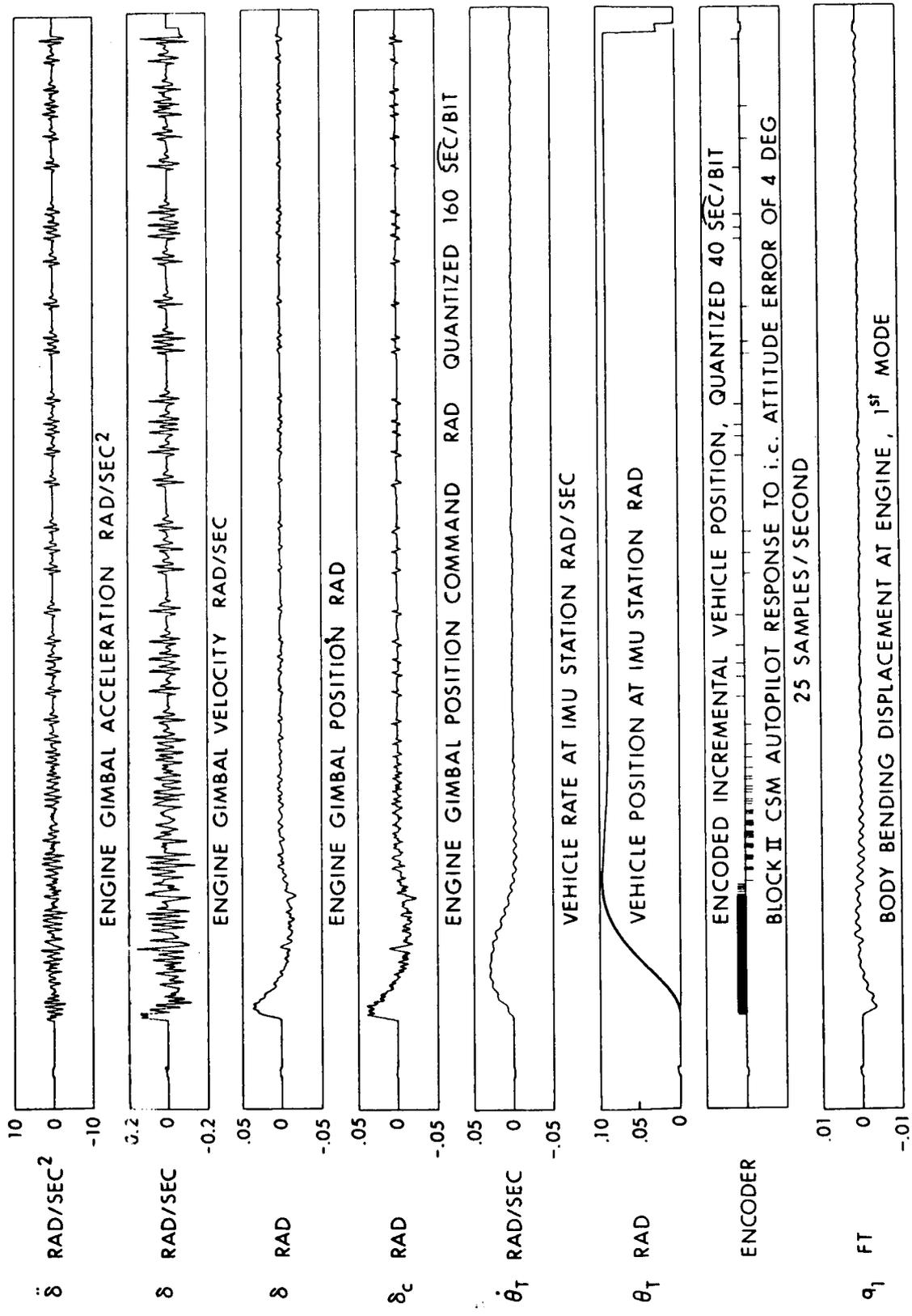
Fig. VII-11 Step Response of Attitude Control System
