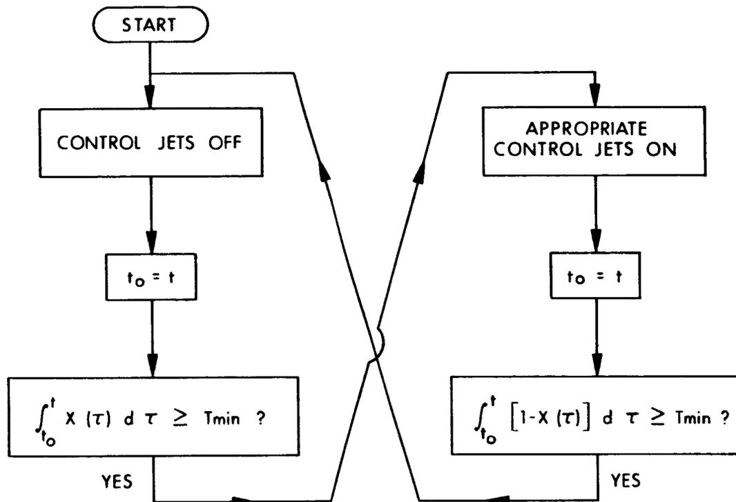
Fig. VII-20 Control Logic for Schaefer or Pulse Ratio Modulator
