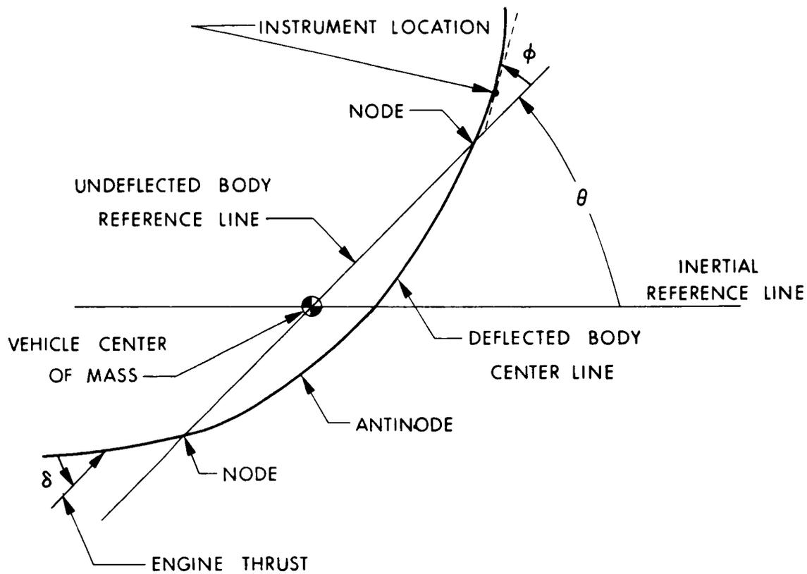
Fig. VII-1 Idealized Body Bending Mode Shape
