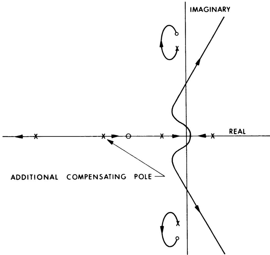
Fig. VII-4 Simplified Root Locus Plot for System with Lag Compensation for Bending Mode
