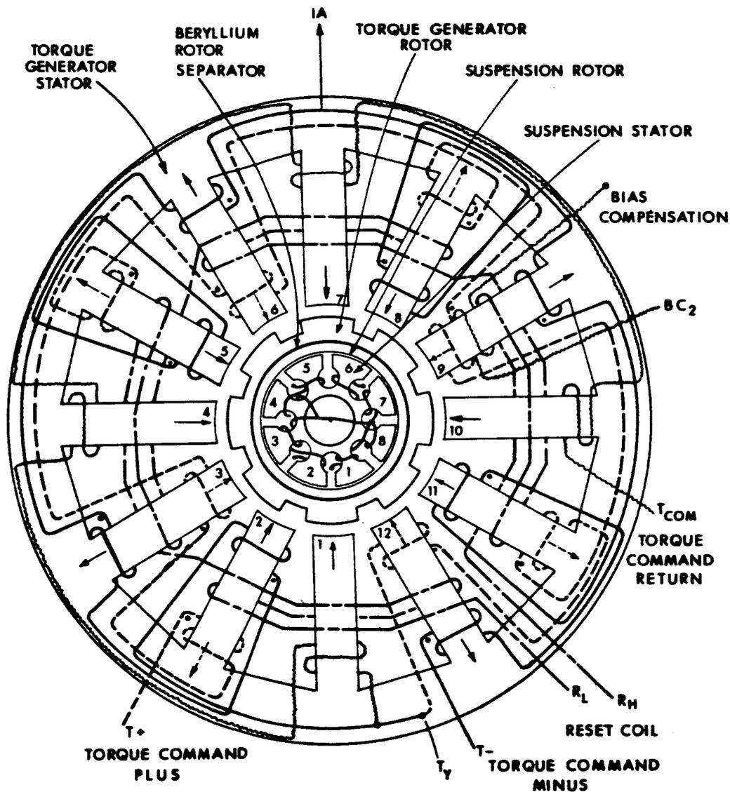
Fig. IV-14 Apollo II Torque Generator and Suspension
