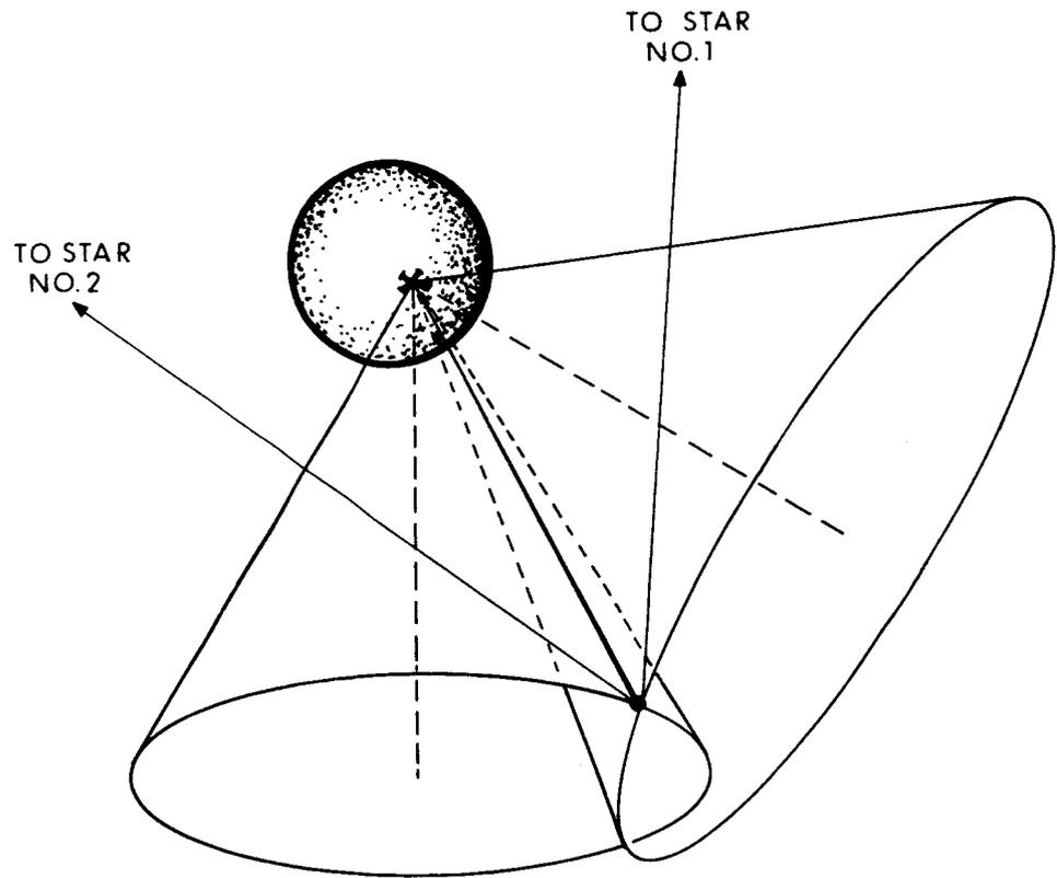
Fig. V-20 Measurement Geometry Using One Landmark and Two Stars
