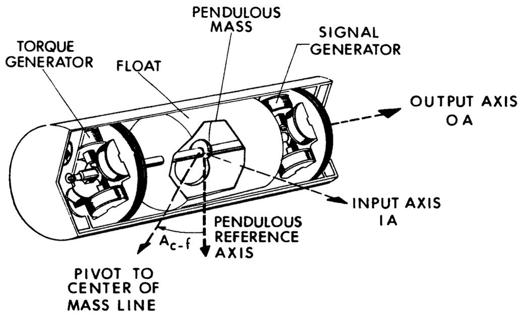
Fig. IV-18 Pulsed Integrating Pendulum Schematic
