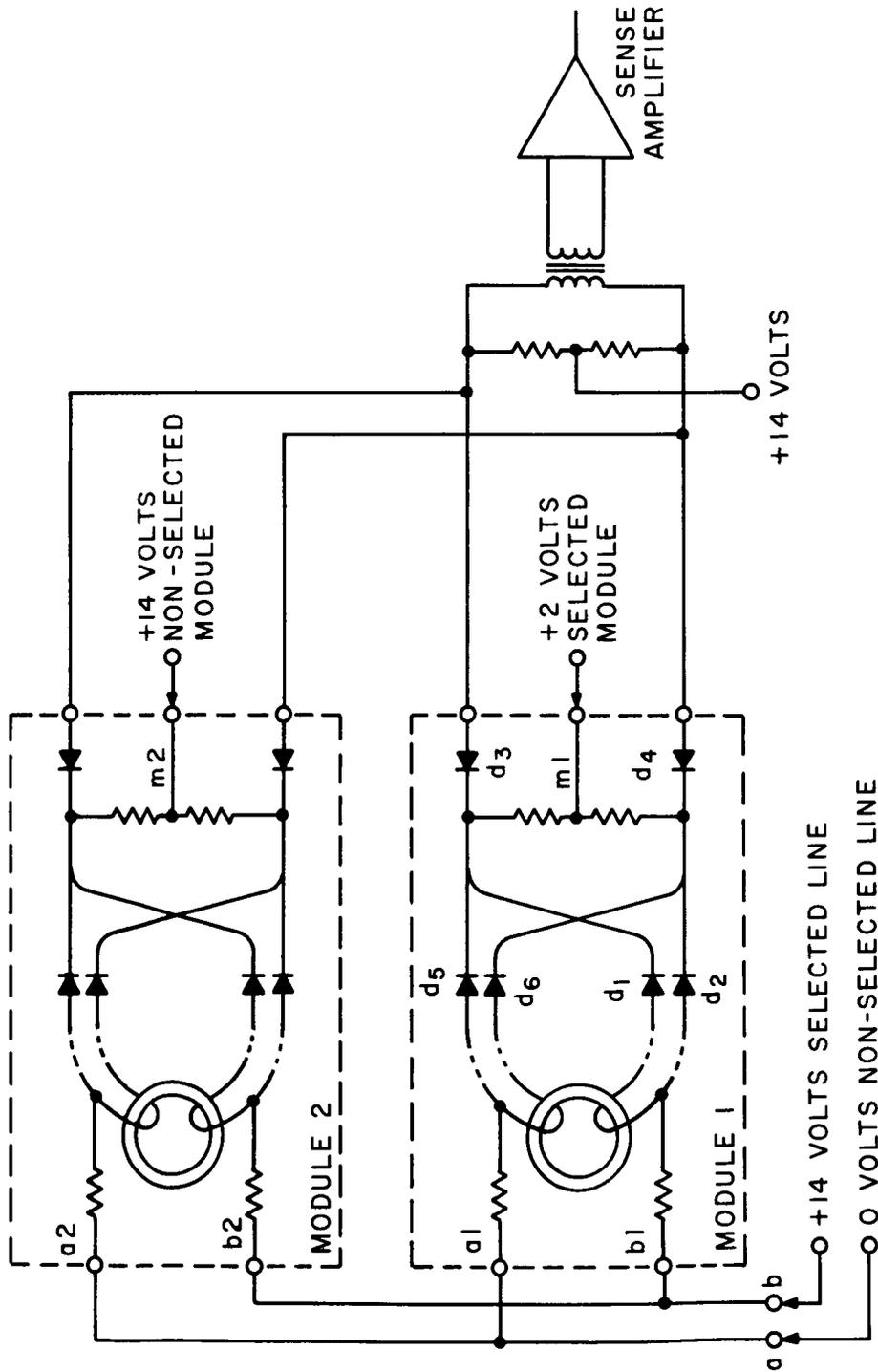
Fig. VI-17 Simplified Rope Sense Line Switching Diagram
