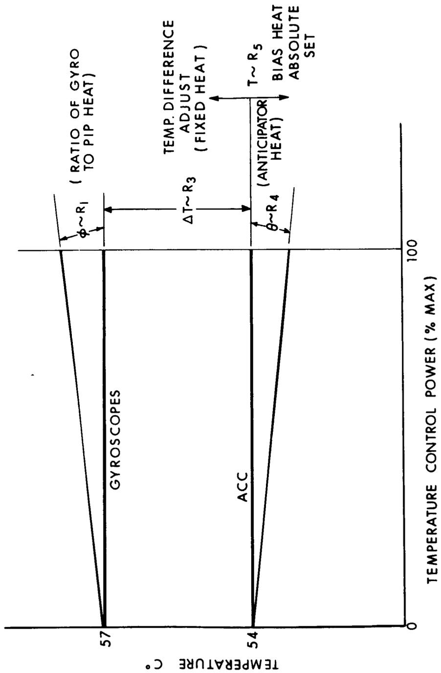
Fig. IV-4 IMU Temperature Control Trimming Resistor Functions
