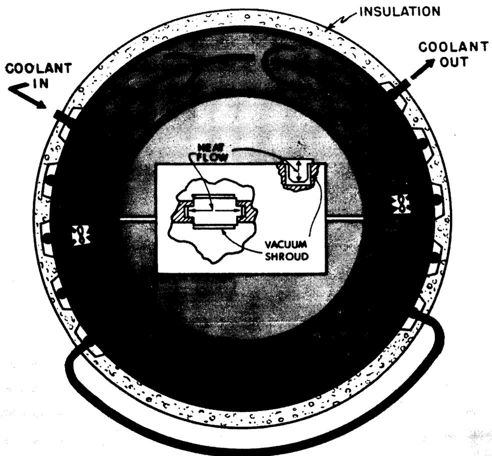
Fig. IV-2 IMU Heat Transfer Diagram
