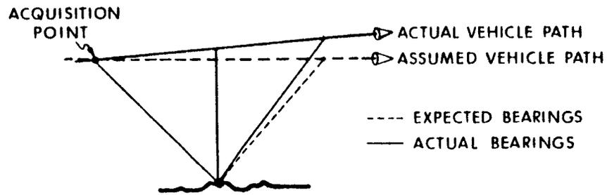
Fig. V-11 Tracking with an Erroneous Vertical Velocity
