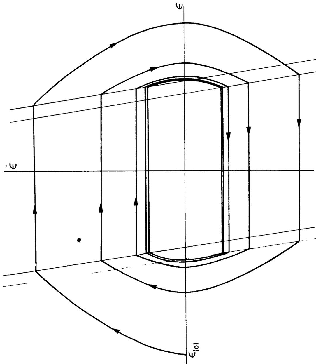
Fig. VII-14 Step Response with Small Rate Gain
