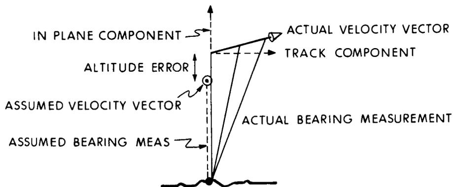
Fig. V-15 Tracking with Erroneous Track Velocity, Altitude, Error, and Vertical Velocity Error
