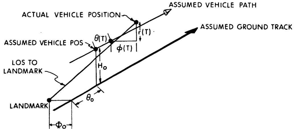
Fig. V-4 Known Landmark Measurement Geometry
