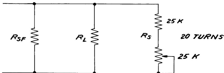
With this method precision adjustment is possible by the use of the potentiometer. Resistance stability is generally better than 3 ppm/year with temperature coefficients of less than 3 ppm/ $C^{\circ}$  deviation. The Precision Voltage Reference
