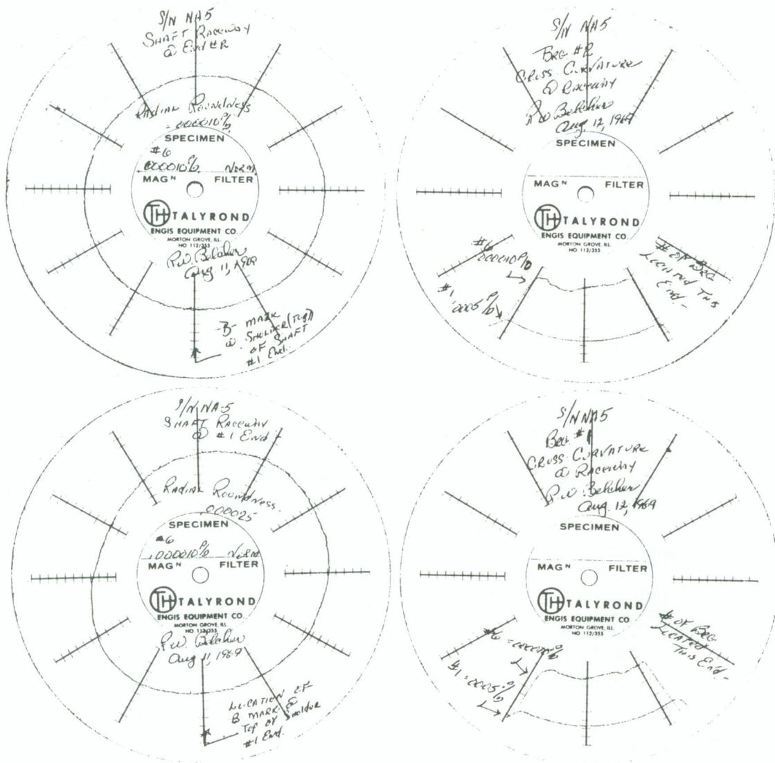
Fig. A-16 Roundness and cross race curvatures of inner races assembled to shaft (Wheel R-2B).
