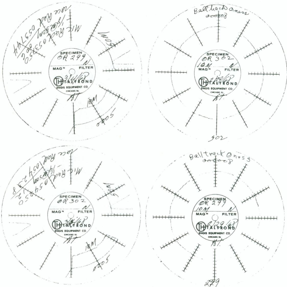
Fig. A-2 Roundness and cross race curvatures of outer races (Wheel R-2)
