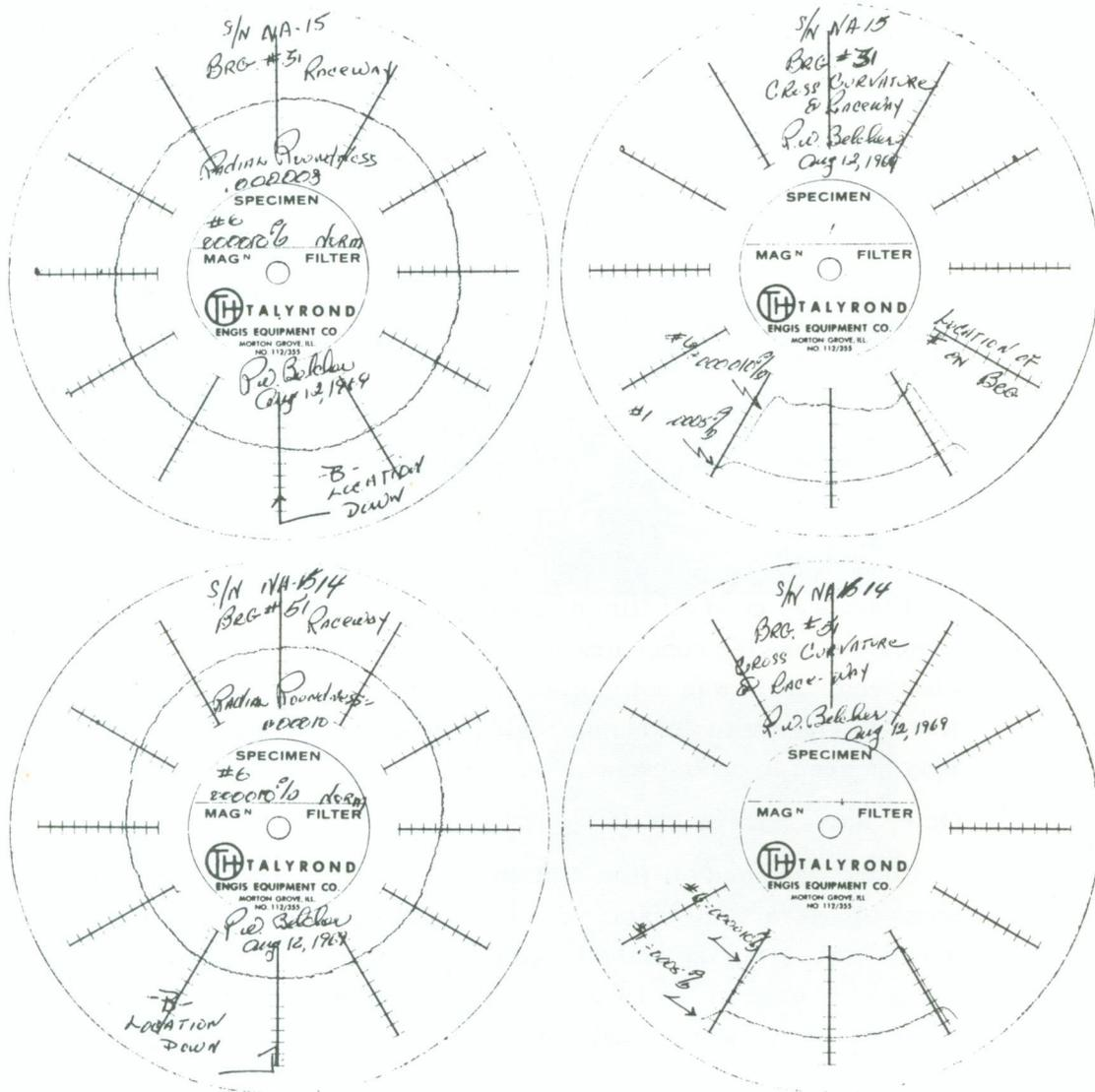
Fig. A-12 Roundness and cross race curvatures of outer races (Wheel R-2A).
