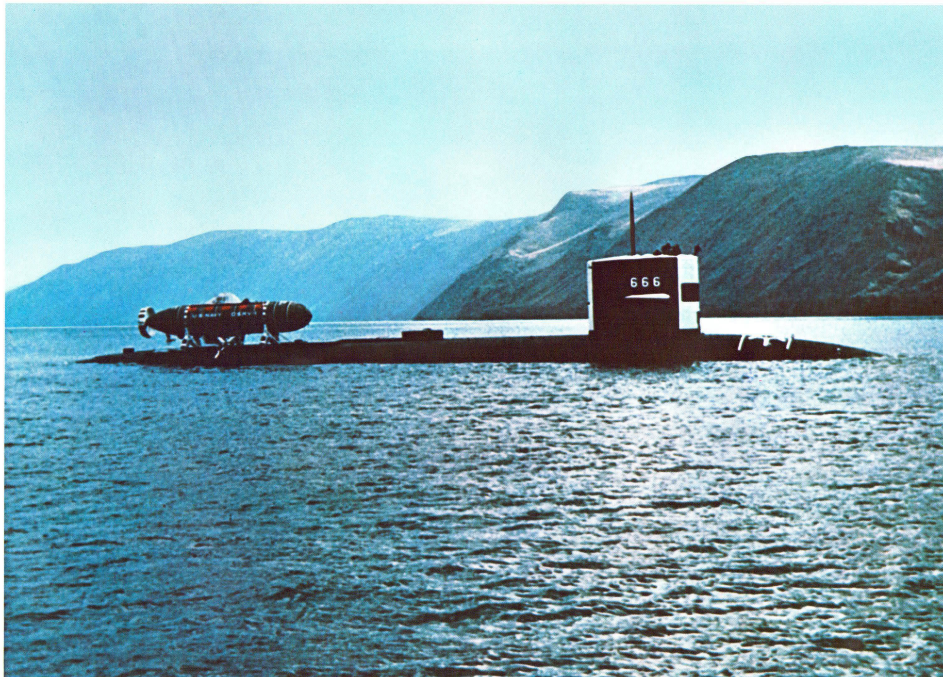
Deep Submergence Rescue Vehicle riding "piggyback" on mother submarine
