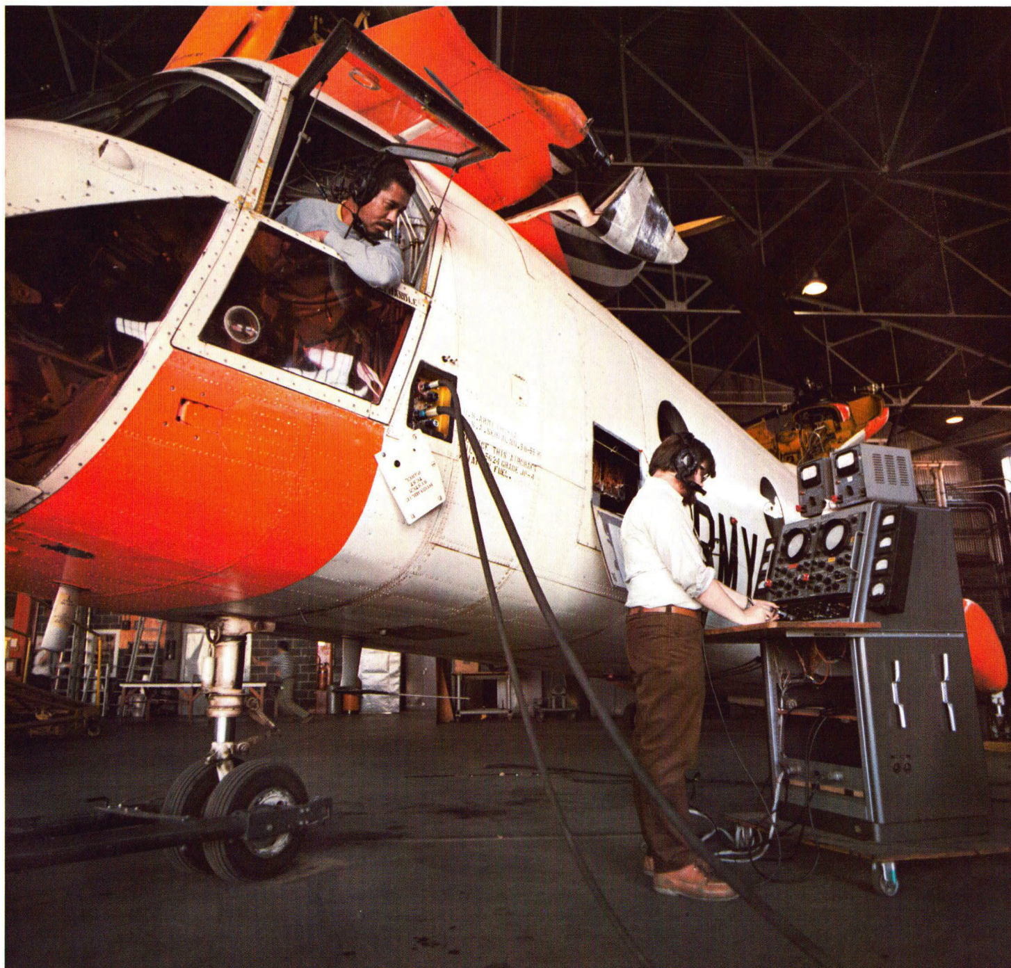
Pre-flight checkout of VTOL experimental control system
