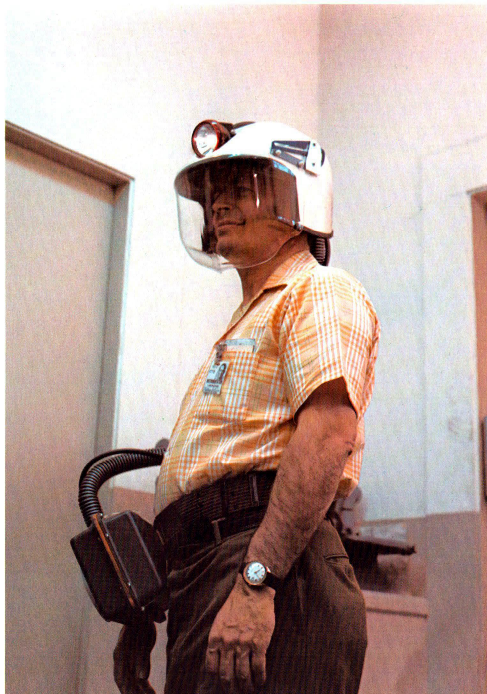
Miner's helmet with a self-contained air supply, developed to reduce the hazards of mining
