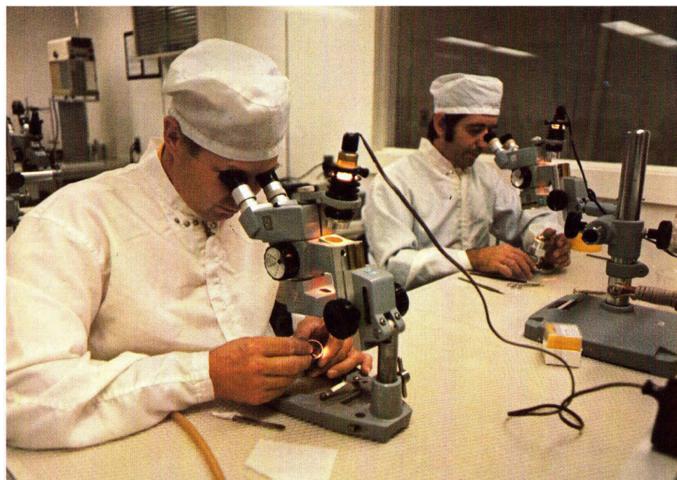
Inertial component assembly in a laboratory clean room
