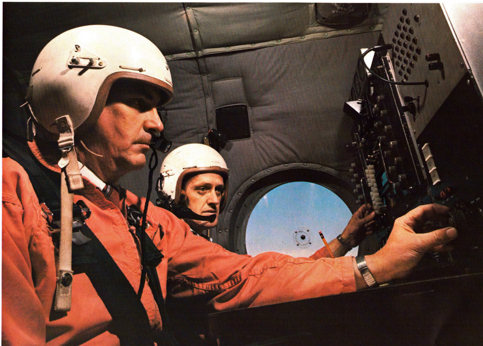
In-flight checkout of VTOL experimental control system
