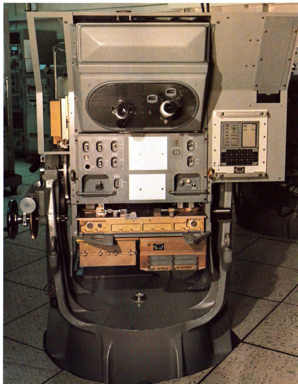
Apollo, Command Module primary Guidance and Navigation system
