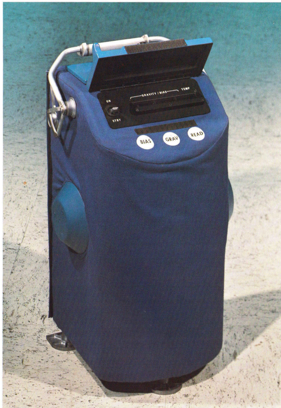
Exterior view of Lunar Gravimeter, an Apollo 17 experiment
