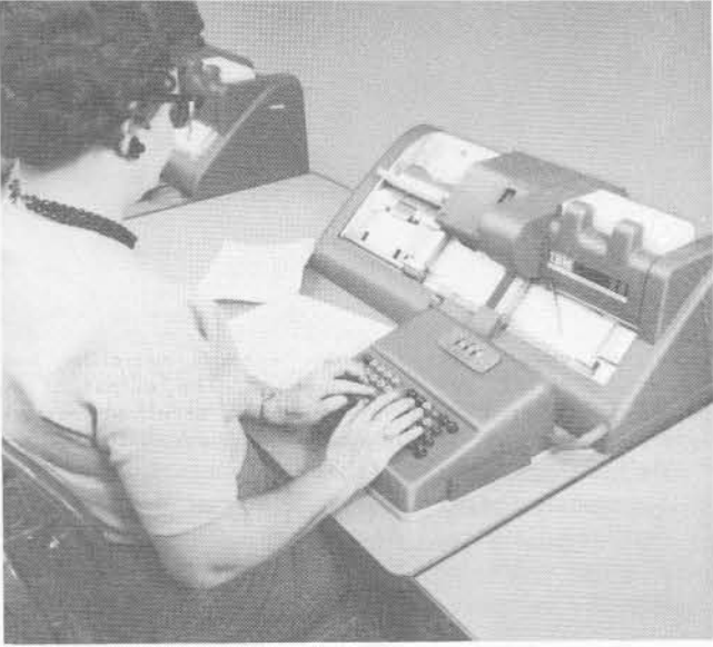
Model 26 printing card punch machines are used to key punch microfilm system cards and master file cards.
