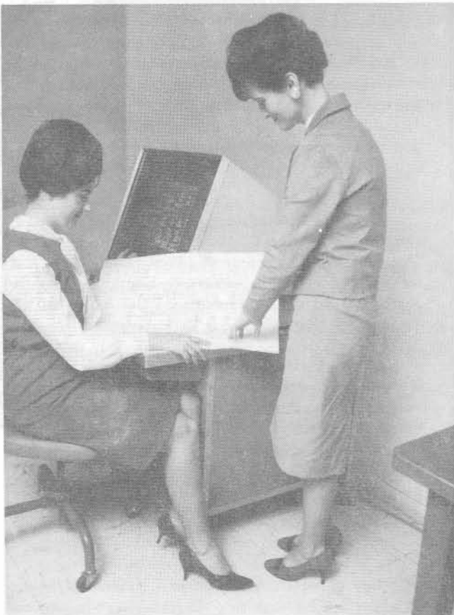
Reader-printers are provided for viewing and making prints of individual microfilm aperture cards.
