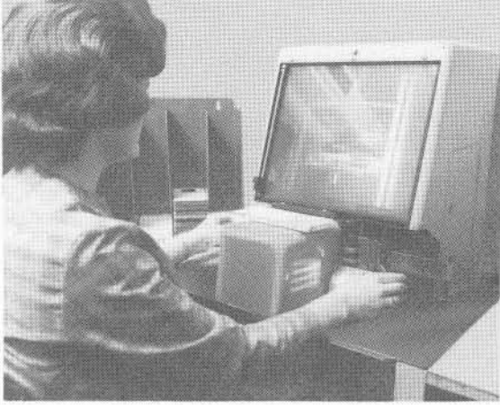
This semi-automatic mounter is used to mount up to 3000 silver microfilm images into aperture cards daily.
