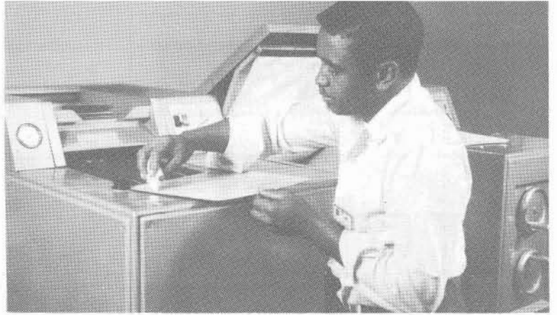
The Model II is used to make offset masters from hard copy. Up to 180 masters can be produced per hour.
