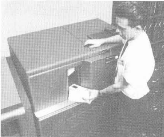
Model 557 card interpreters are used to interpret the punches in the microfilm aperture cards at the rate of 6000 cards per hour.
