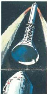
*LES Separation.* Approximately three minutes after launch, the Launch Escape System engine will ignite, carrying the Boost Protective Cover away with it. This will be the first test of the system under actual lunar-mission flight conditions.
