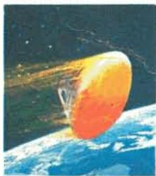
Until now, spacecraft have re-entered from the normal earth-orbiting speed of 17,500 mph. Because of this dramatic difference in re-entry speeds, Apollo's CM heat shield has been designed to weather twice as much heat as Gemini and Mercury did.
