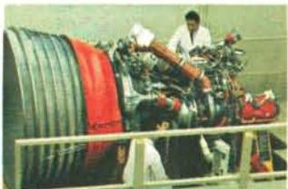
landing mission, it will have to re-ignite. Apollo 4 will be the first test, in space, of firing the J-2 engine, shutting down, then re-igniting.
