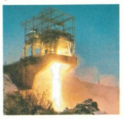
The photo shows a single F-1 engine firing during a captive test.
