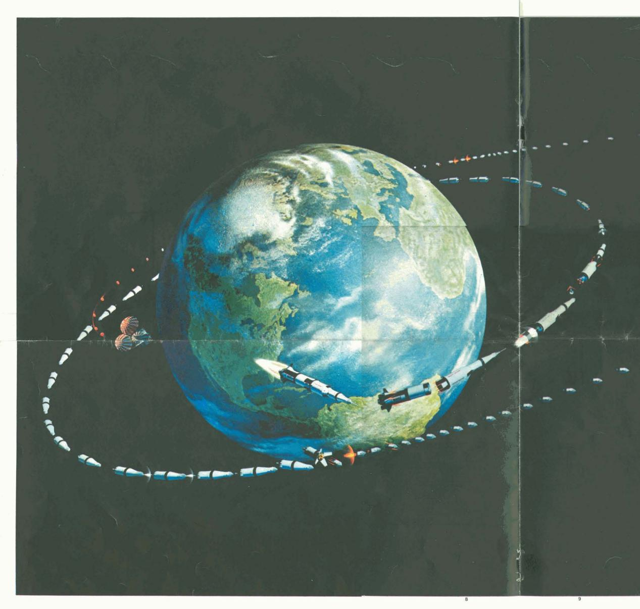
Here – at a glance – is the plan for Apollo 4. Lift-off at Kennedy Space Center...earth orbit and translunar injection...apogee at 11,400 miles...the plummet back to earth and re-entry at almost 25,000 mph...finally, splashdown in the Pacific. (This photograph of the mission was made on a single negative with 89 exposures using a 1/100th-scale model of the Apollo/Saturn V vehicle.)
