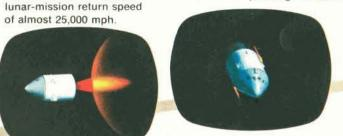
0:11:10 - Third-stage cutoff. Apollo is now in a circular parking orbit around the earth, about 117 miles high at a speed of 17,500 mph. The spacecraft is coasting, without propulsion.
