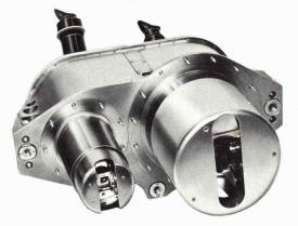
The OUA, a sextant-telescope package, is used to sight on known reference stars and landmarks for the fine angle measurements needed in navigational checks. In most operations, the Command Module pilot will use the telescope to locate a target star, then sight the selected star in the magnified field of view of the sextant to make precise measurements.
