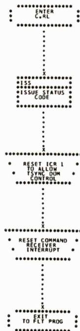
Figure 3-25. Command Receiver Linkage Routine
