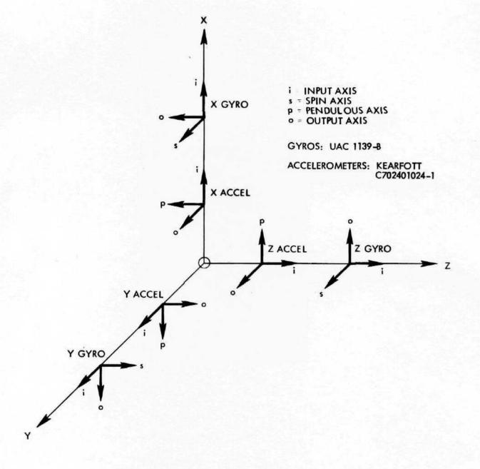
Figure 2-1. ASA Sensor Triad Configuration
