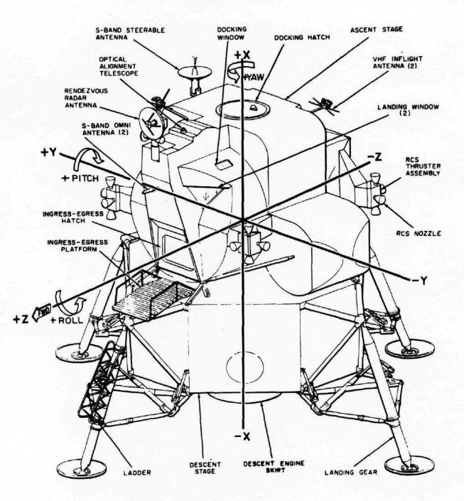
Figure 2-2. LM Body Axis Coordinate System
