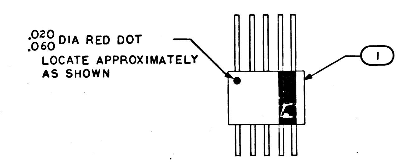
GENERAL REQUIREMENT UPON COMPLETION OF ALL REQUIREMENTS AS SPECIFIED IN ND 1002248, THE NOR GATES WHICH QUALIFY FOR FLIGHT HARDWARE UNDER THE PROVISIONS OF ND 1002248 SHALL BE MARKED IN RED AS INDICATED IN THIS DOCUMENT.
