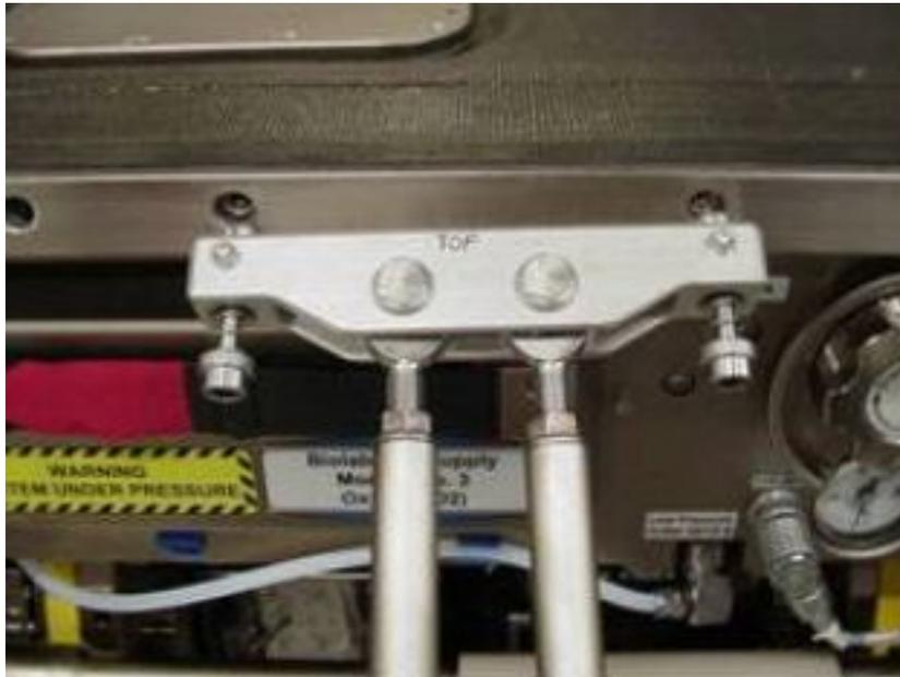
Figure 6. Detail of Upper Jig Strut (bracing rod) fixation
