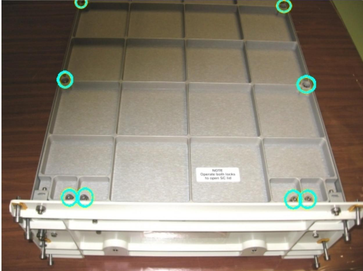
Figure 3. Captive launch fixation bolts on the Stowage Container Lid
