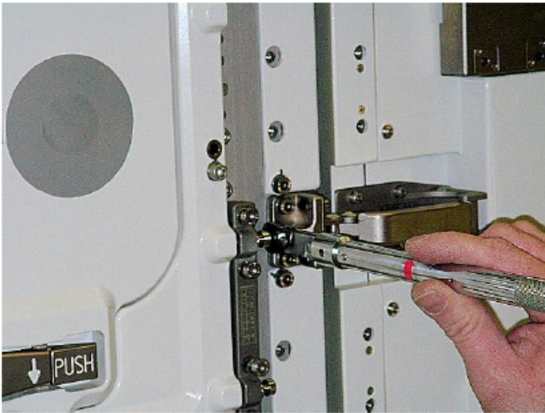
**Figure 2. Details of unscrewing bracket 4 (with tool Biolab incubator wrench tool)**
