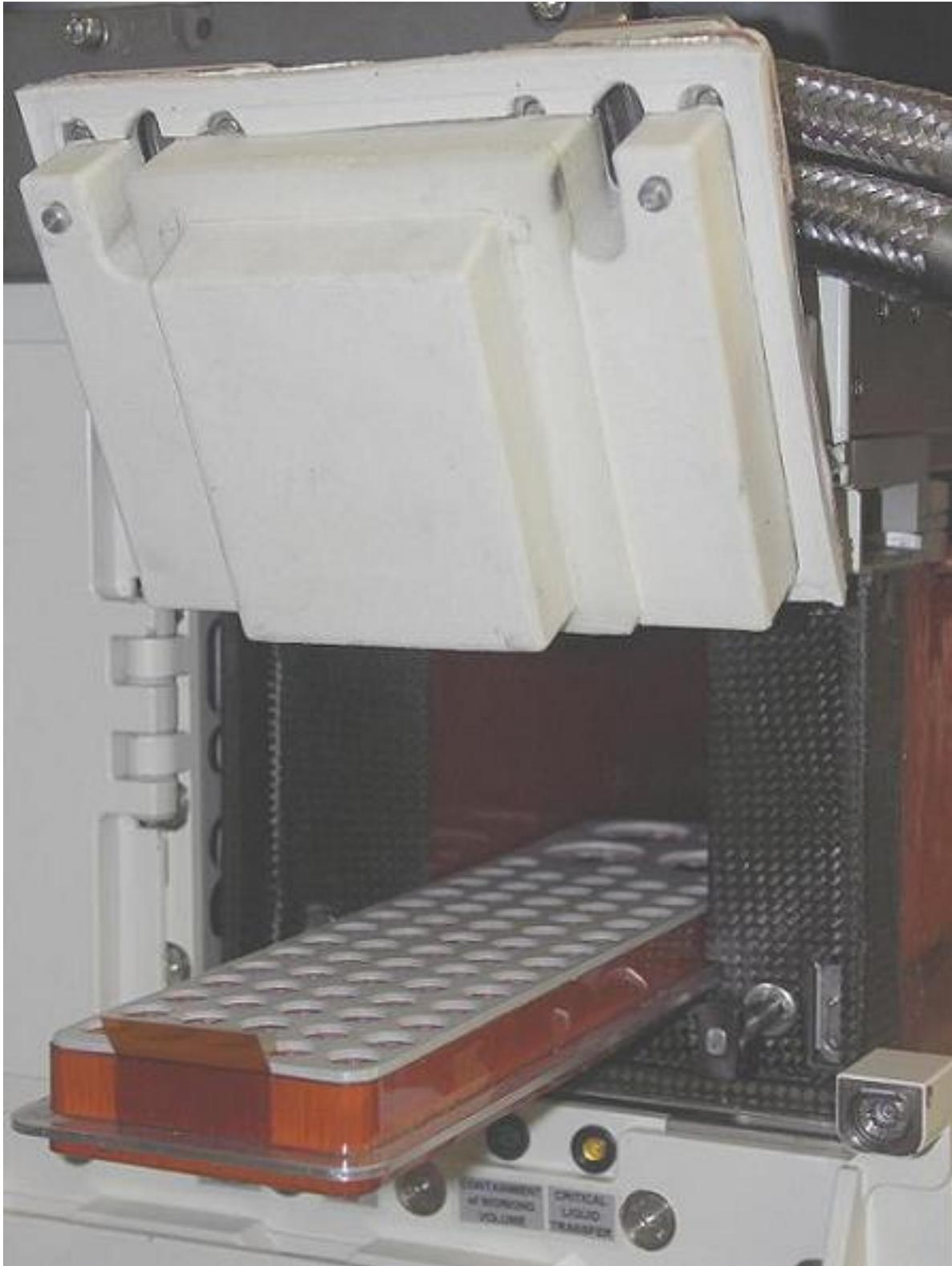
Figure 2. Automatic Temperature Controlled Storage Lower Insulation
