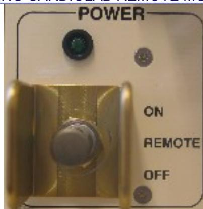
Figure 1. CARDIOLAB POWER switch and POWER LED
