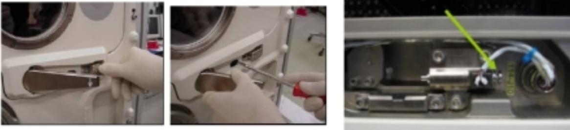
Figure 2. Details of EC Door Manual Override (right picture shows mechanism covered in hole)
