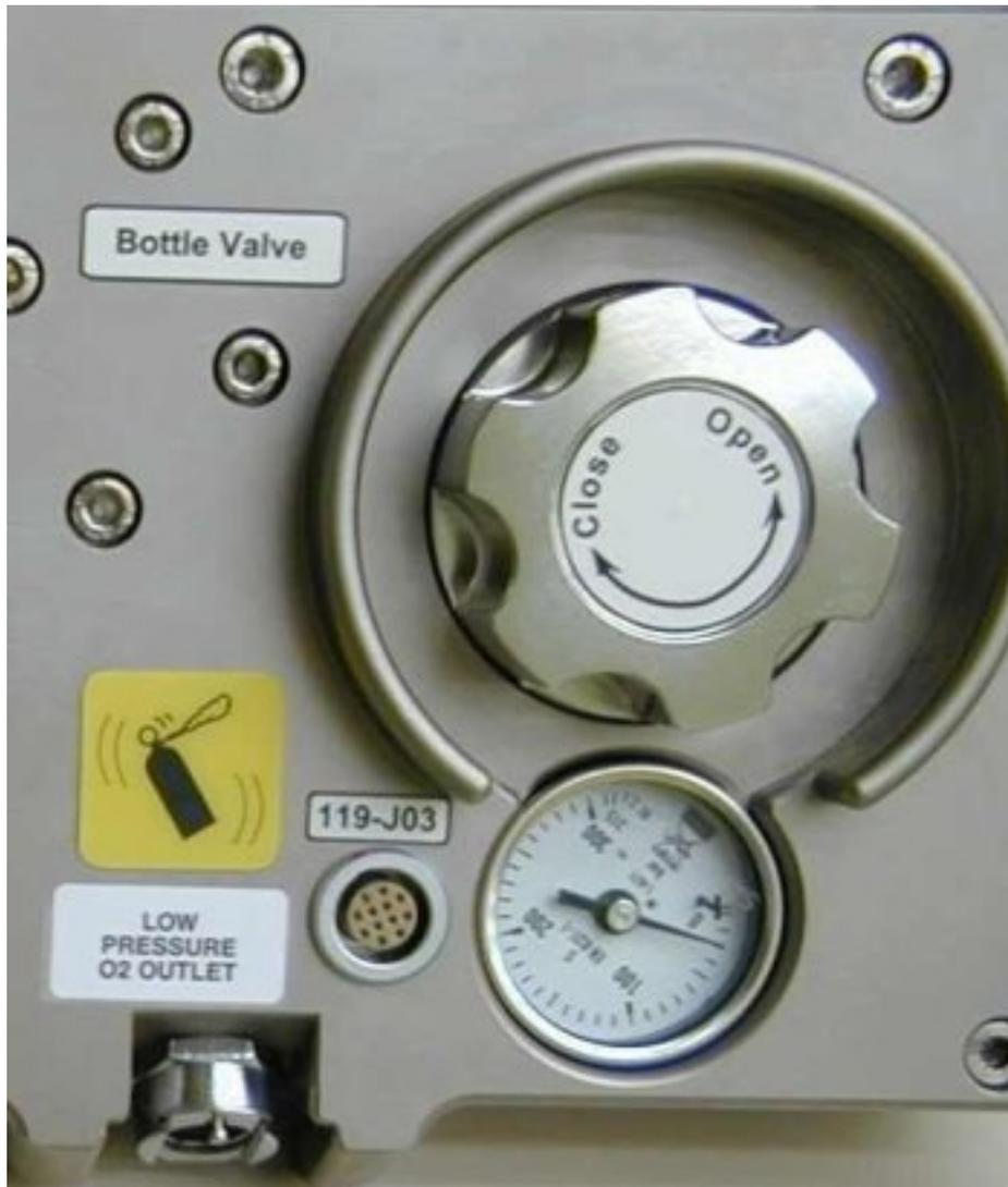
Figure 1. View on O2 pressure gauge (LSM, 3)
