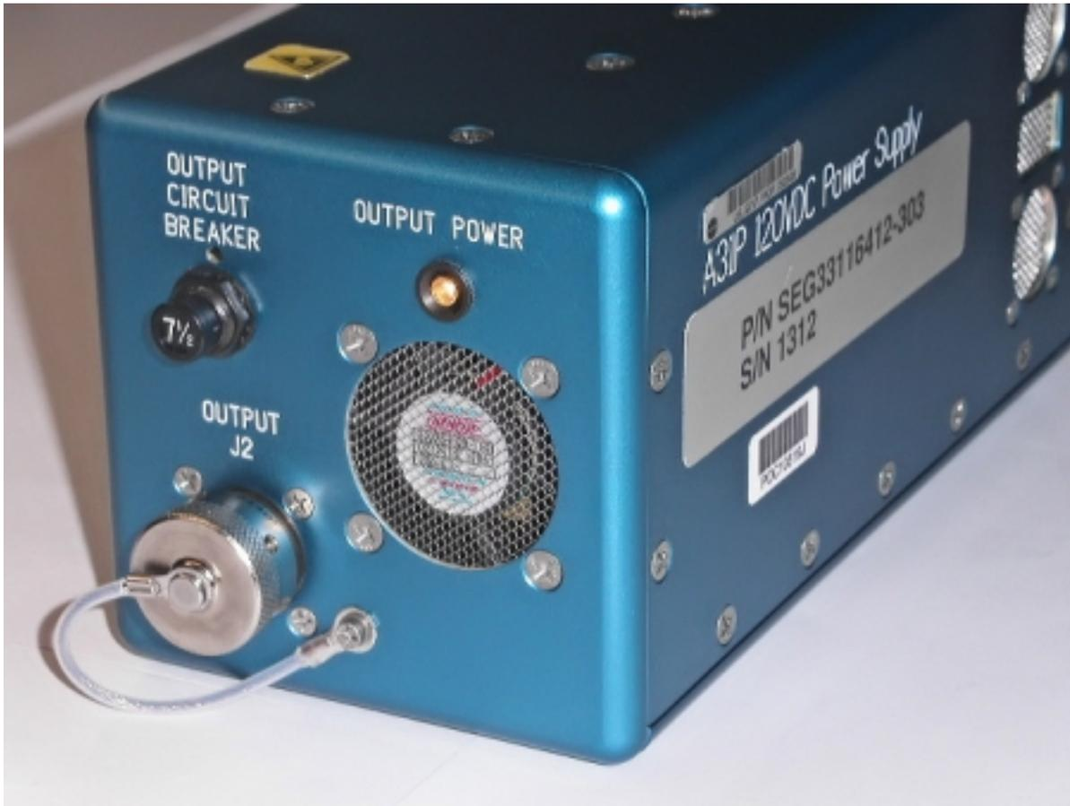
Figure 2. Location of 16 V outlet on DC/DC converter (OUTPUT J2)
