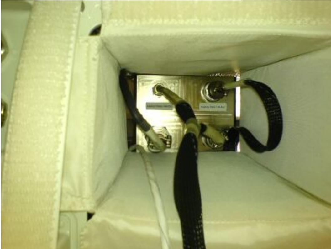
Figure 5. Details of LAN/video cables (one connected harness) and data cable and Nomex cover
