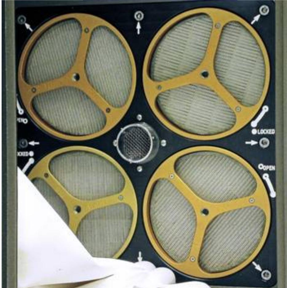
Figure 6. Glovebox Front Filter Plate (for launch the four Glovebox Front Filters will be removed)
