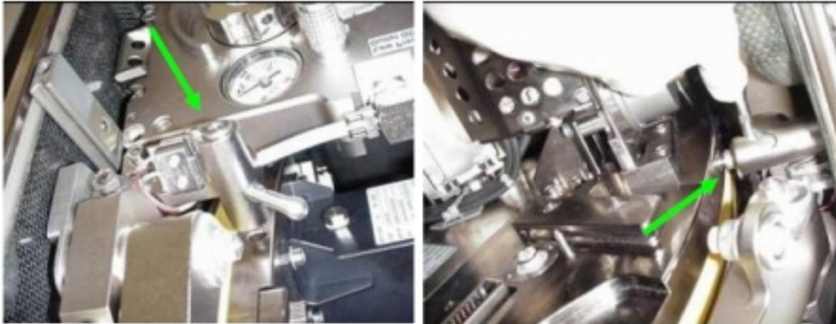
**Figure 3. Details of Rotor Manual Lock (green arrow)**
