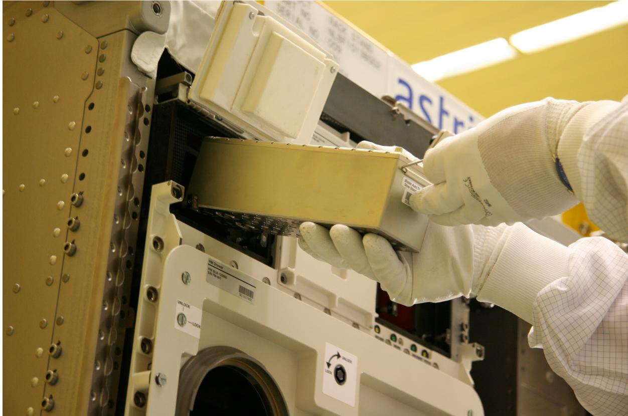
**Figure 3. Auto Temp Cntl Stow Test Insert Installation**
