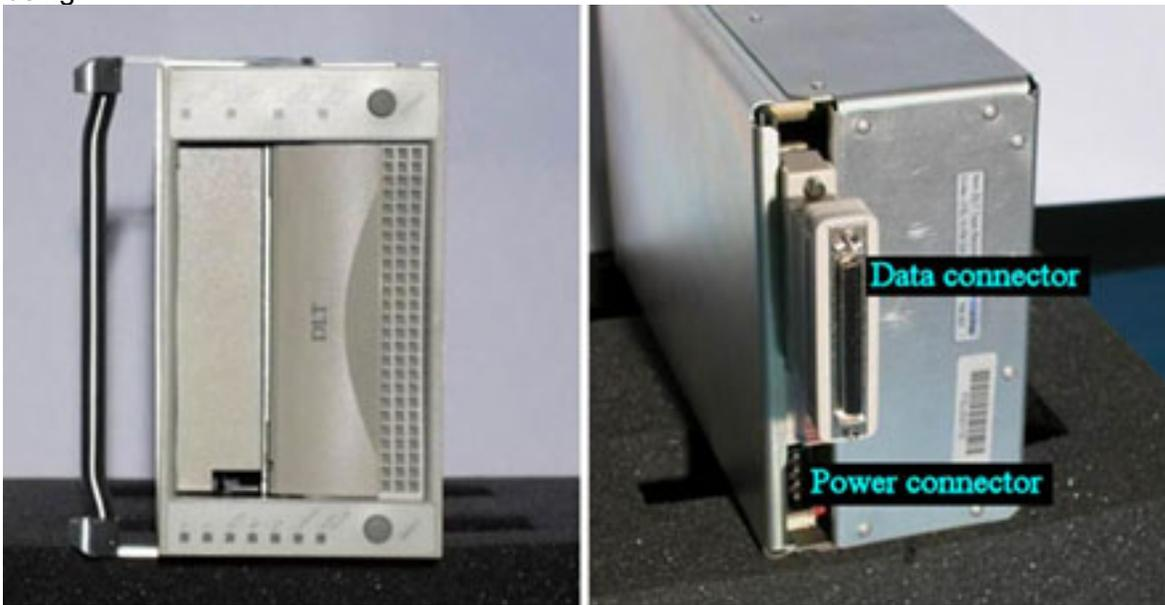
Figure 4. FSL VMU DLT Recorder (front and rear view)
