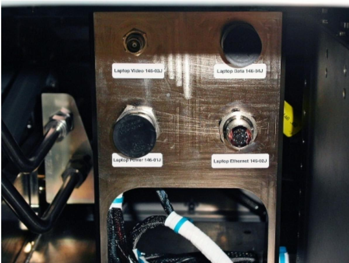
Figure 1. Laptop bracket with connectors
