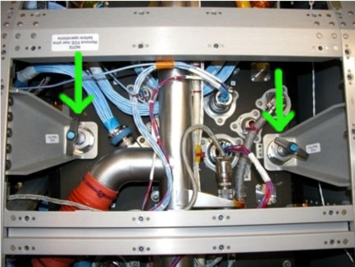
Figure 4. Facility Core Element Rear Pins (indicated by the green arrows, frame corresponding to the L2 panel)
