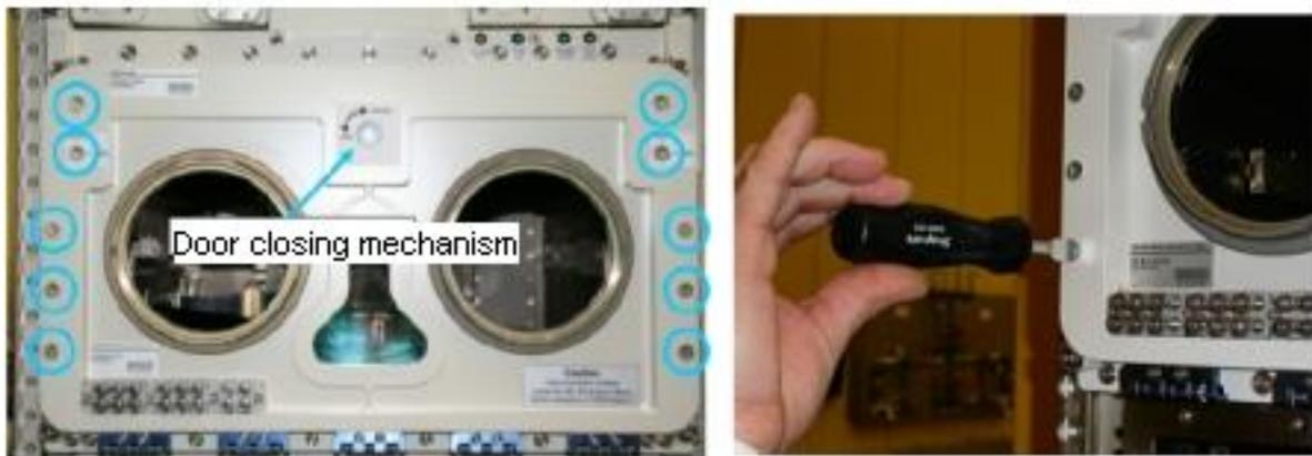
Figure 1. Location of HM door screws and locking mechanism (blue circles)
