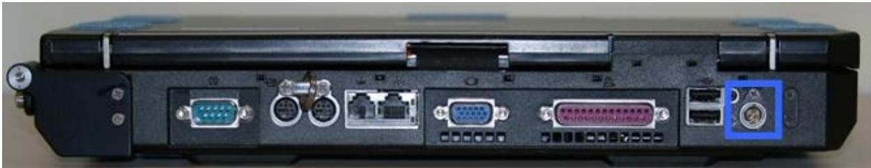
Figure 6. EPM Laptop Power socket
