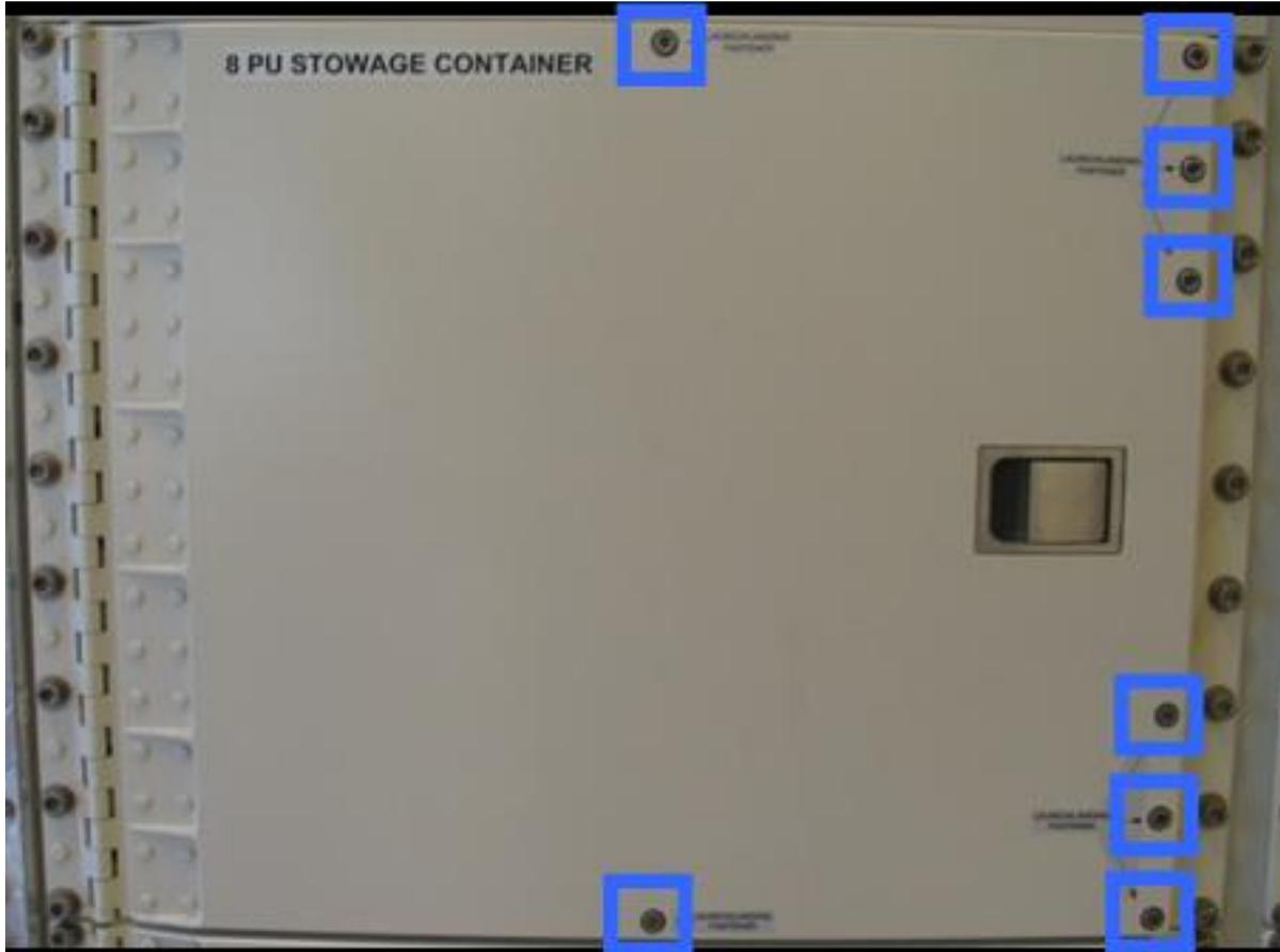
Figure 3. EPM 8-PU Stowage Container Launch and Landing Fasteners
