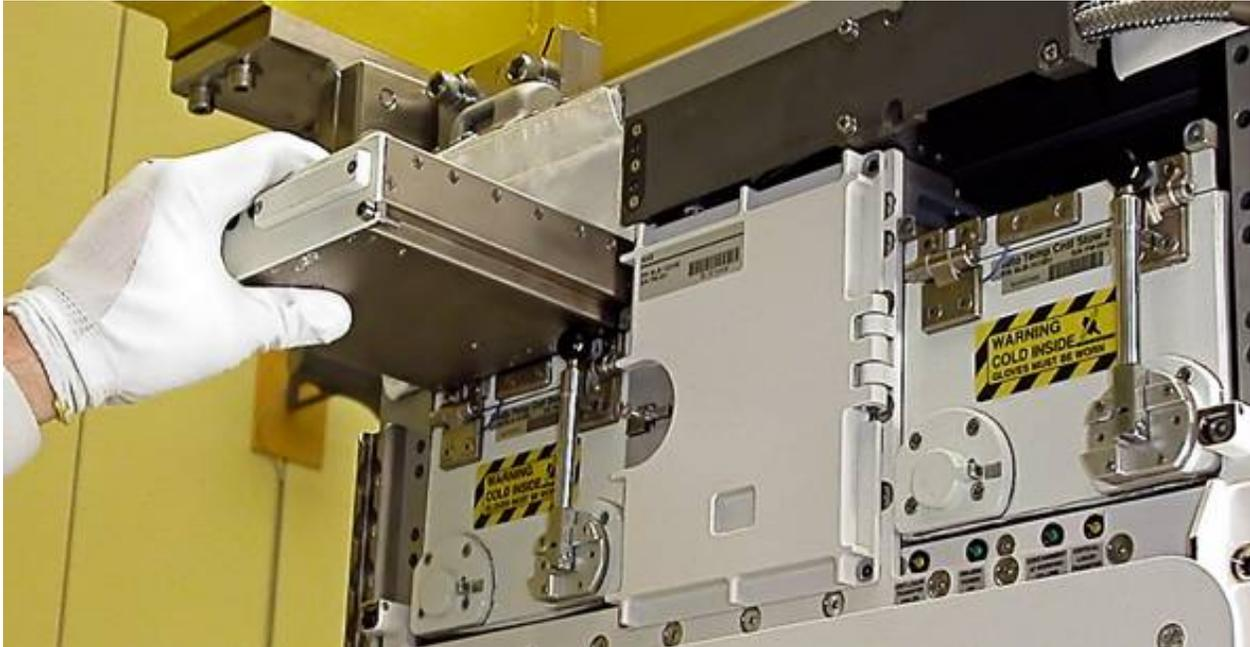
Figure 2. Automatic Temperature Controlled Stowage E-Box insertion
