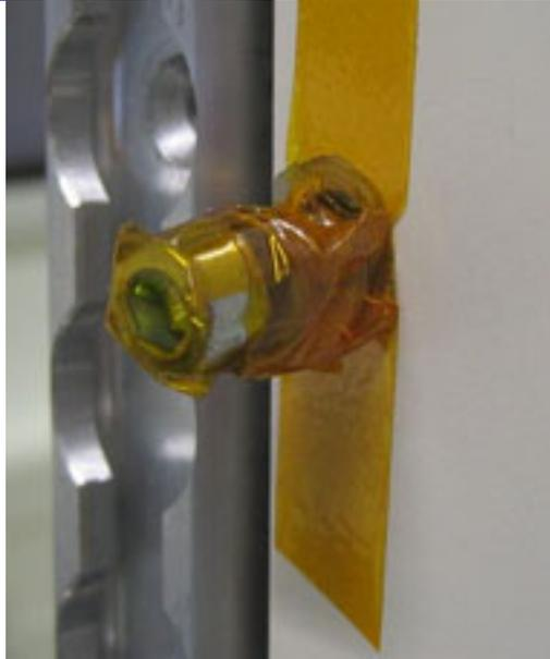
**Figure 4. Loose Bolt with Kapton Tape**
