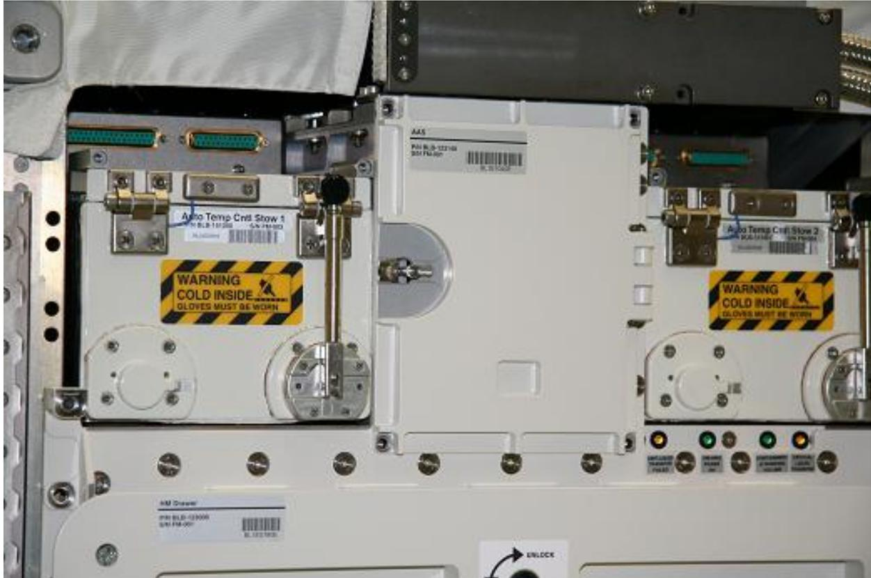
Figure 1. Biolab Auto Temperature Control Stowage 1 and 2 without E-box
