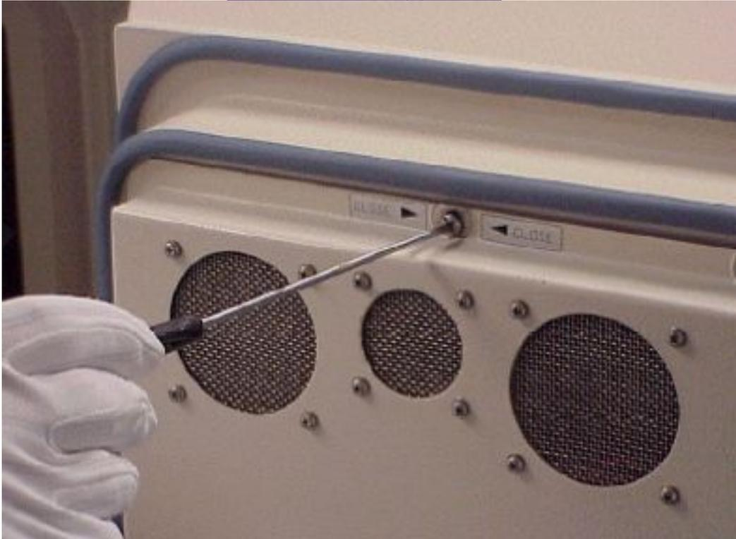
**Figure 4. Removal of TCU Fan Lid**
