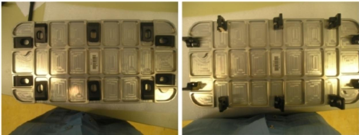
Figure 1. AAS lid, left: brackets in closed position, right: brackets prepared for lid opening
