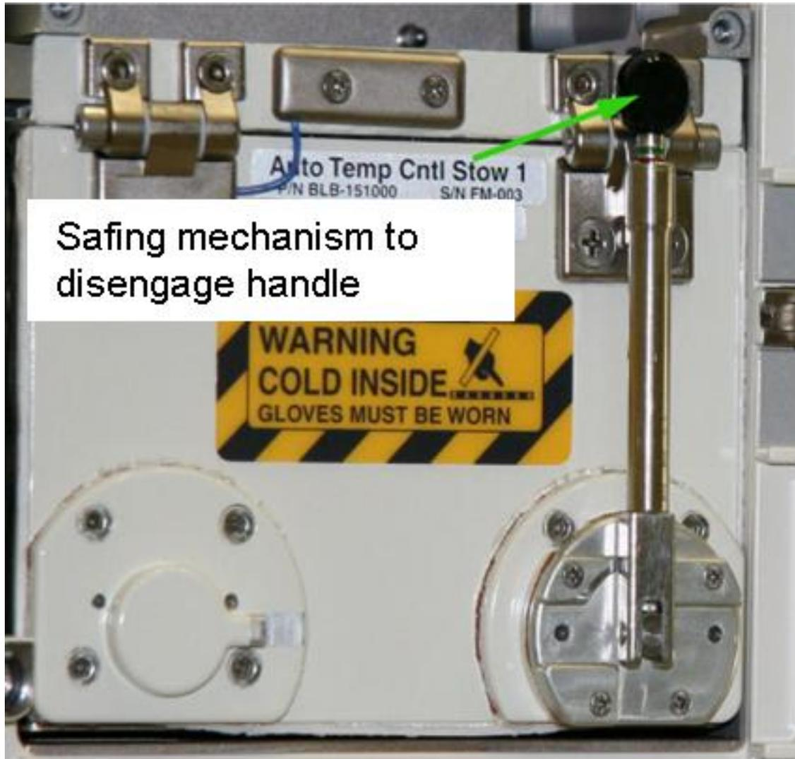
Figure 1. Automatic Temperature Controlled Stowage 1
