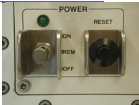
**Figure 1. MEEMM POWER switch and POWER LED**
