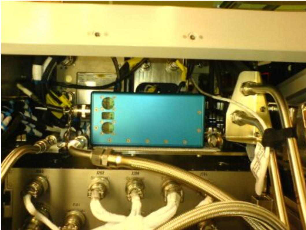
Figure 3. Positioning of DC/DC converter on RIC coldplate
