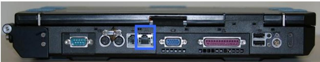
**Figure 5. EPM Laptop Ethernet socket**
