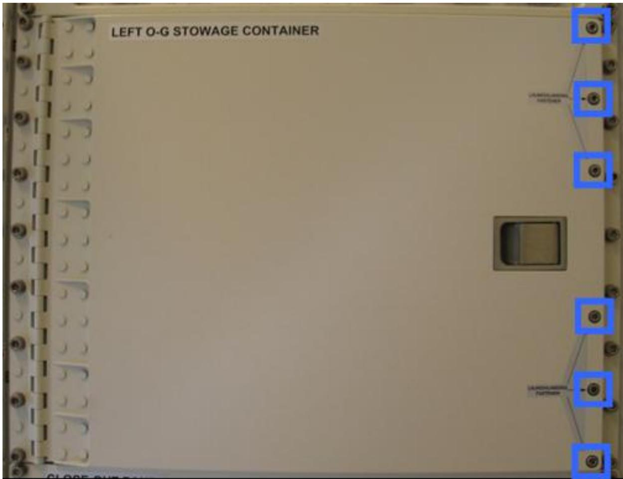
Figure 4. Left 0-G Stowage Container Launch and Landing Fasteners
