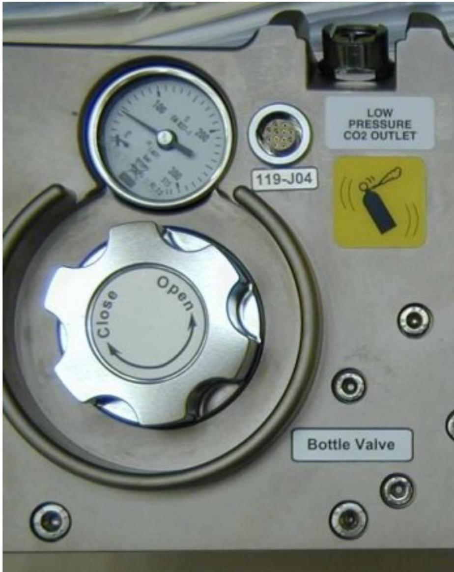
Figure 2. View on CO2 pressure gauge (LSM, 4)
