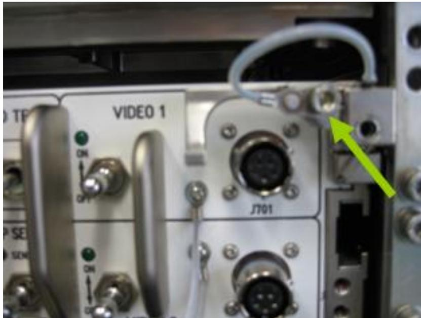
Figure 4. Launch position of captive bolt on the locking mechanism
