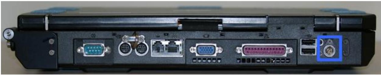
**Figure 3. EPM Laptop Power socket**
