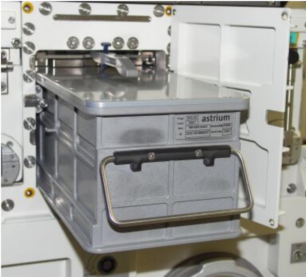
**Figure 3. AAS insert insertion into AAS housing**
