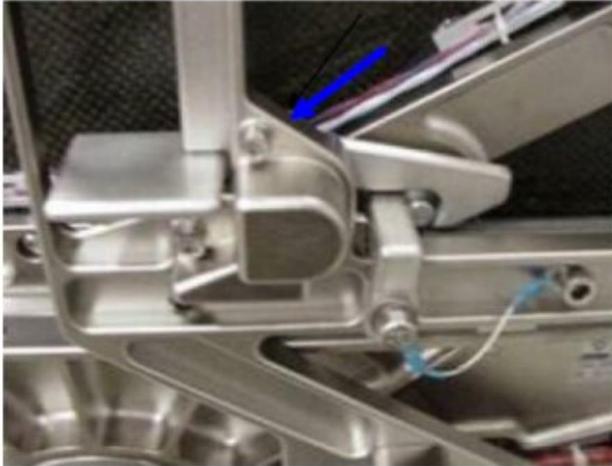
**Figure 14. Detail of jig locking mechanism (blue arrow)**
