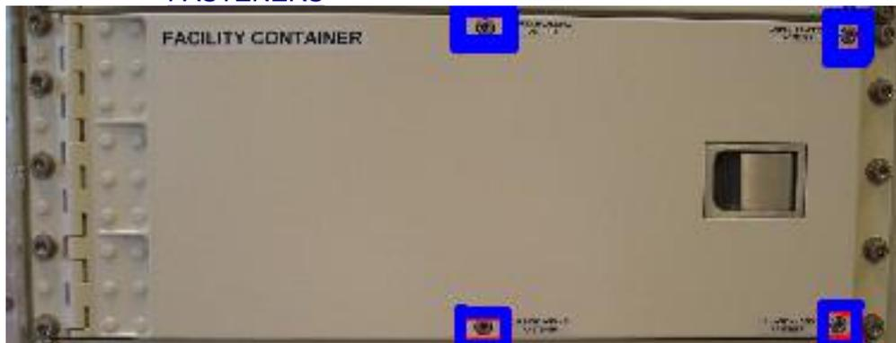
Figure 1. EPM Facility Container Launch And Landing Fasteners
