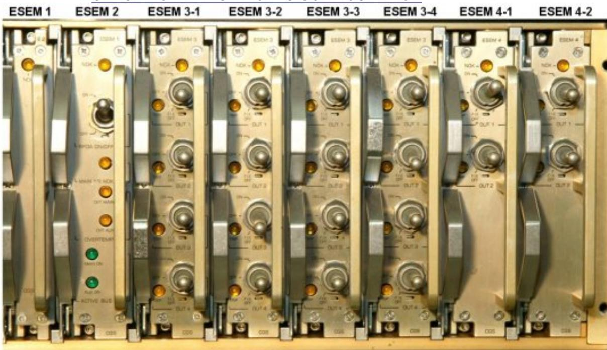
Figure 1. Biolab RPDA ESEM boards
