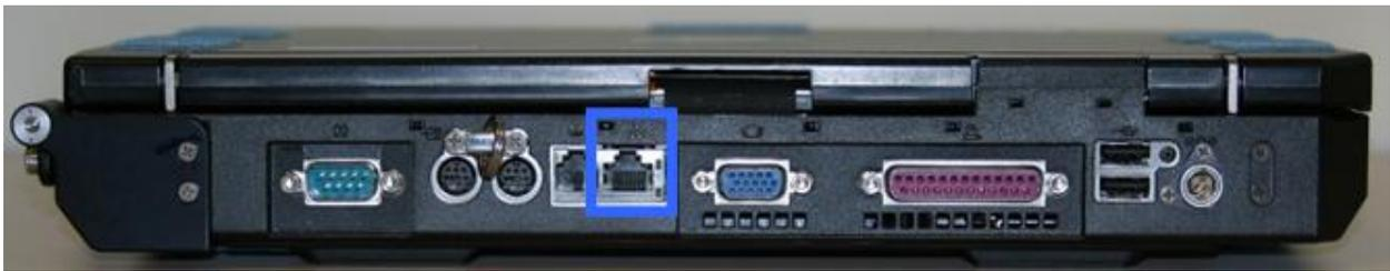
Figure 3. EPM Laptop Ethernet socket
