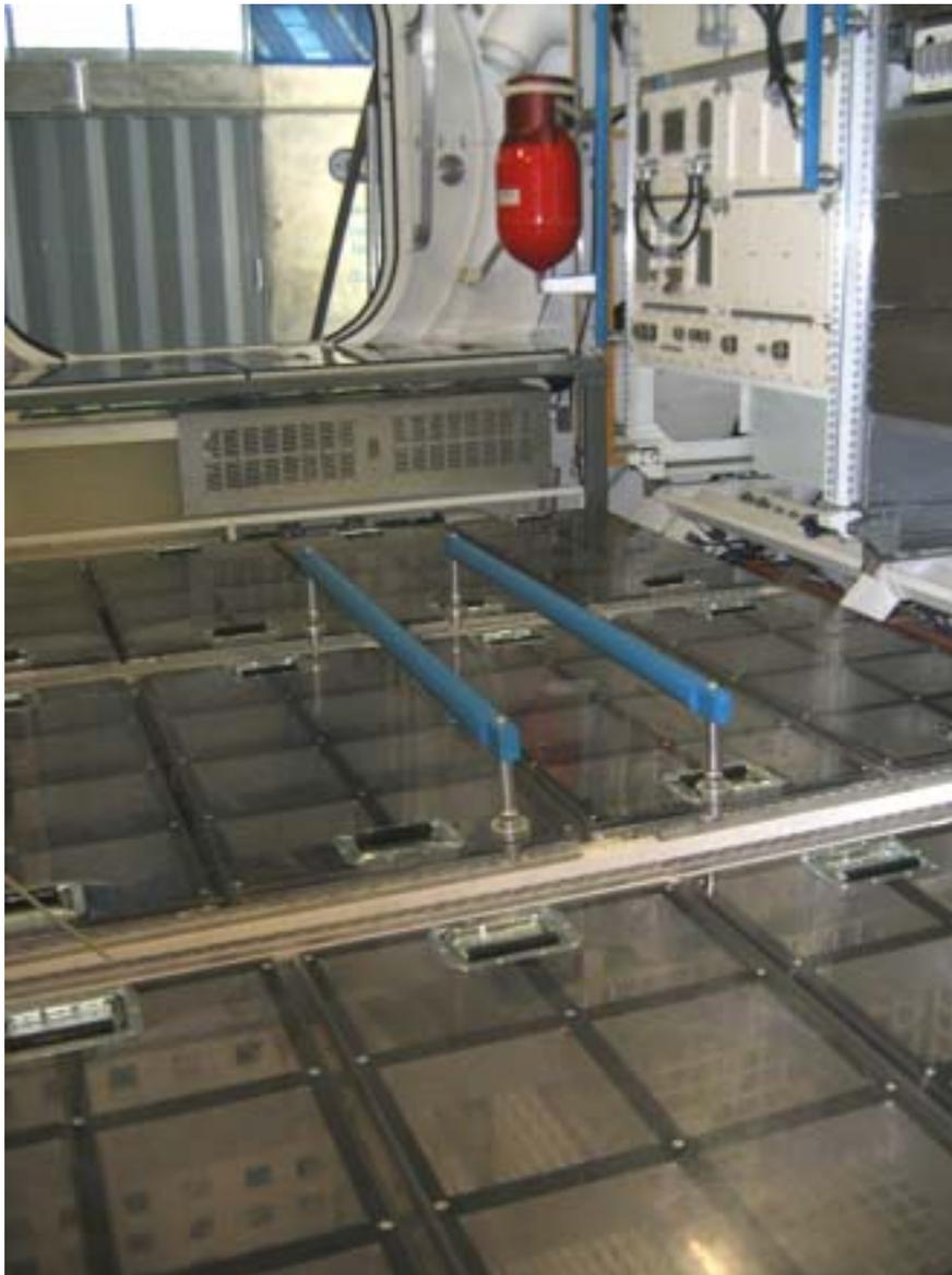
Figure 2. Banisters Mounted on Columbus Mockup Seat Tracks
