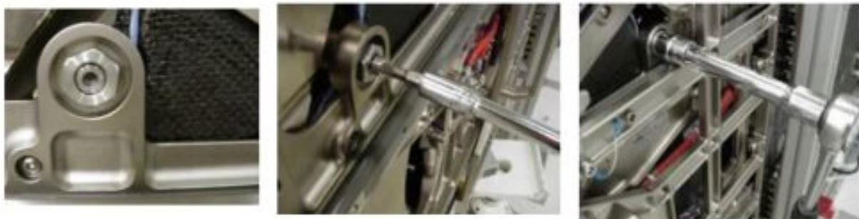
Figure 11. Details of complete rotor spacer-screw unit (left), internal fixation screw (middle) and spacer (right)
