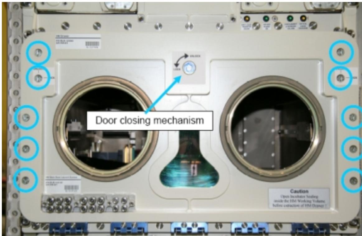
Figure 1. HM Door Locking Screws (blue circles) and Door Closing Mechanism (blue arrow)
