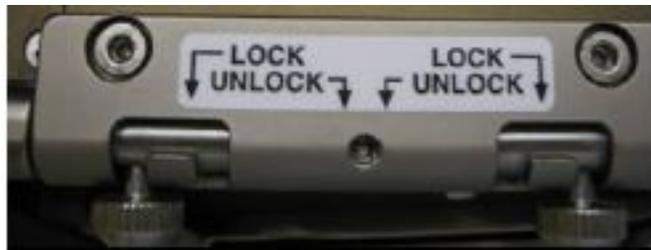
Figure 7. Glovebox Glove Door locking pins
