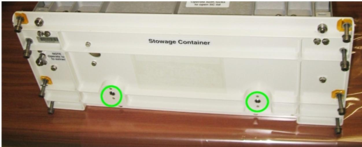
Figure 5. Stowage Container - Handle position
