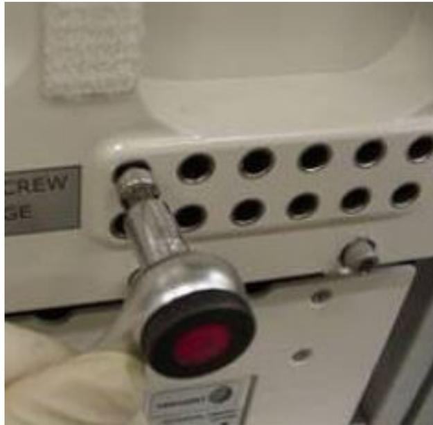
Figure 4. Stowage provision for launch/landing screws on Inc main door
