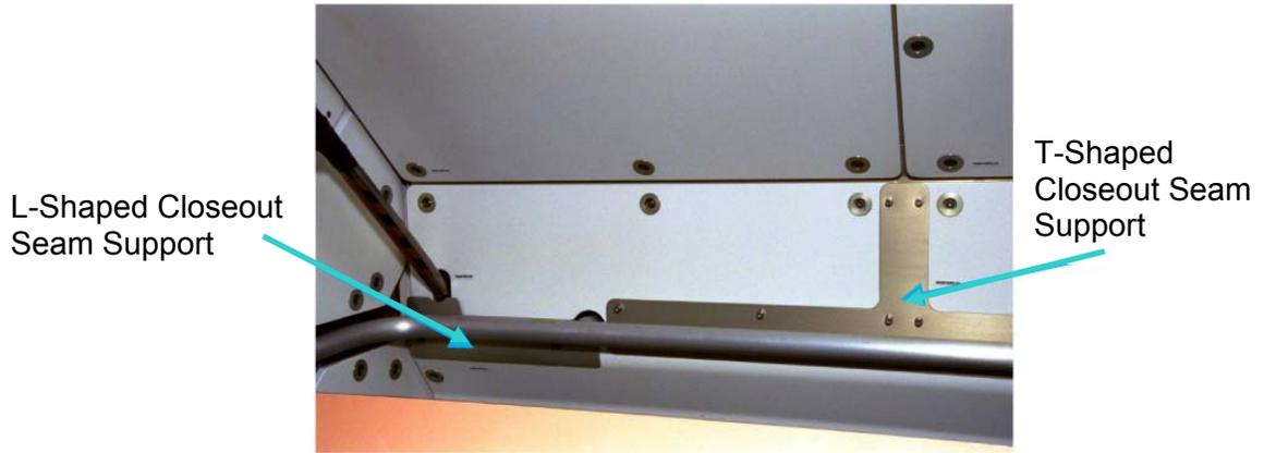
Figure 4.- Closeout Seam Supports.
