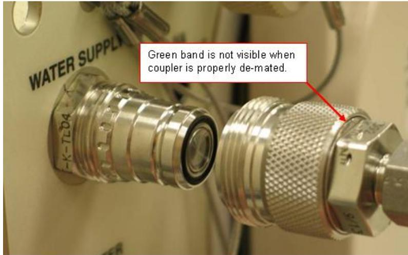
Figure 5. Properly de-mated small QD coupler.
