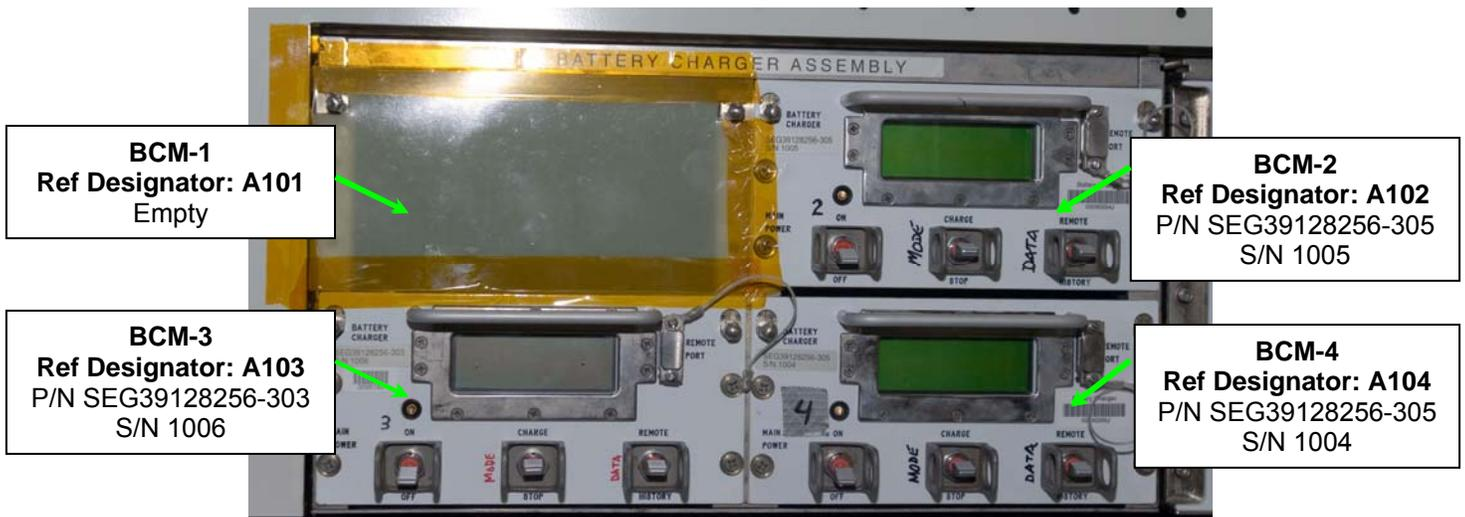
Figure 1.- Battery Charger Module Reference Designations and Current Configuration.
