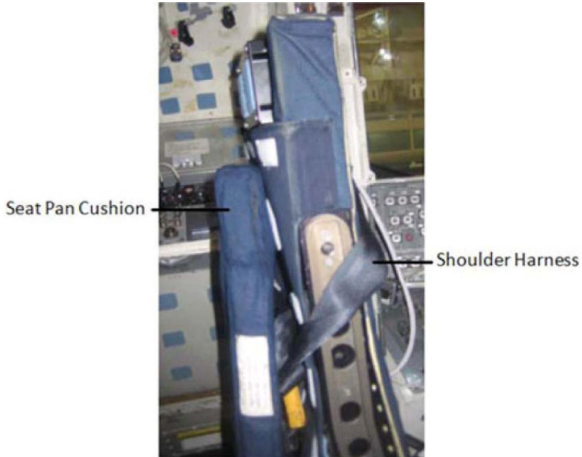
Figure 1. Shoulder Harness Wrapped Around CDR Seat Back.
