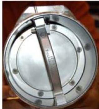
Figure 8.- Example of Closed IMV Valve.
