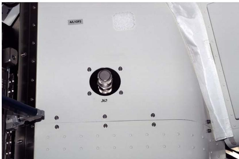
Figure 2.- J62 Connector Mounted to A/L1OF2 Closeout Panel.
