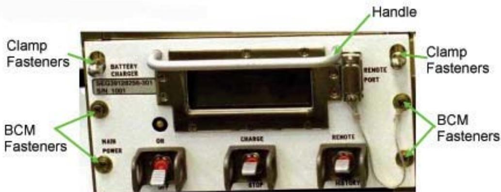
Figure 7.- BCM Housing Assembly Captive Fasteners.
