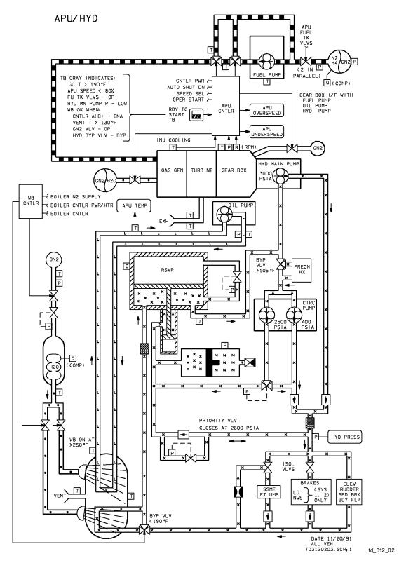
Figure 2-3. APU/HYD/WBS schematics
