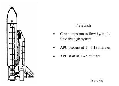
Figure 5-2. APU/HYD/WSB system use prior to launch
