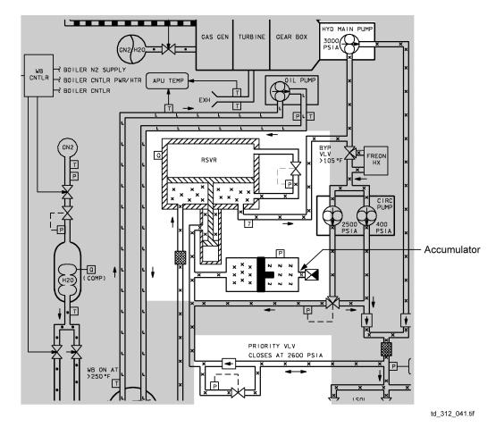
Figure 3-3. Reservoir/accumulator package
