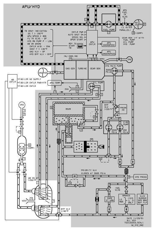
Figure 4-1. Water spray boiler system
