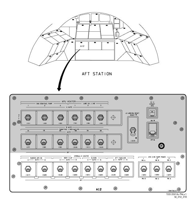
Figure 3-10. Panel A12 and its location
