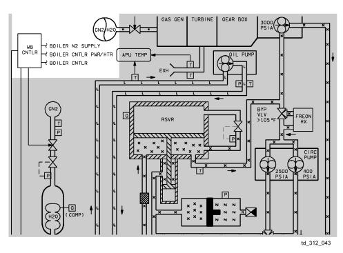
Figure 4-2. WSB electronic controller
