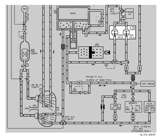
Figure 3-4. Hydraulic circulation pumps
