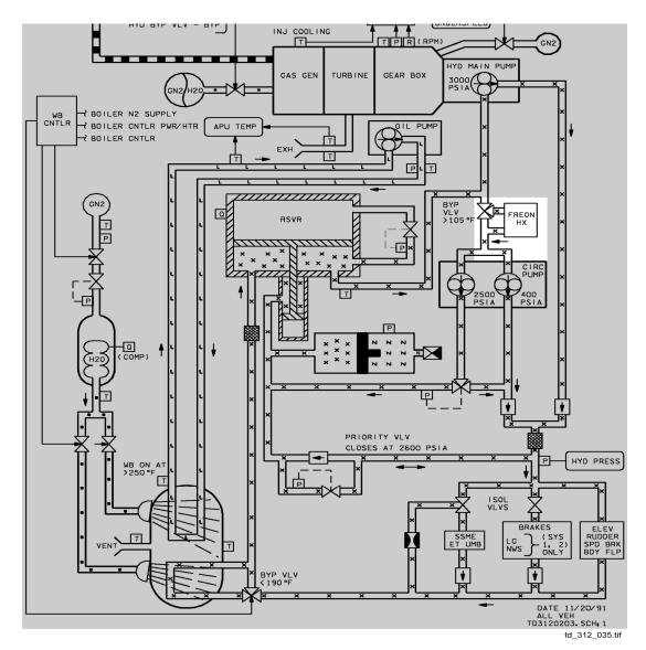
Figure 3-5. Hydraulic/freon heat exchanger
