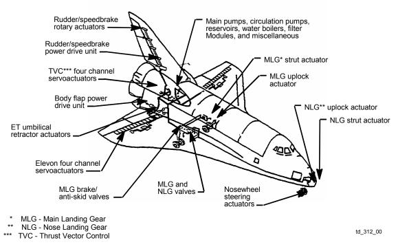
Figure 3-1. Hydraulic system location
