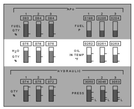
Figure 4-9. HYD/APU Subsystem Status Display meters
