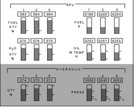
Figure 2-17. HYD/APU Subsystem Status Display meters
