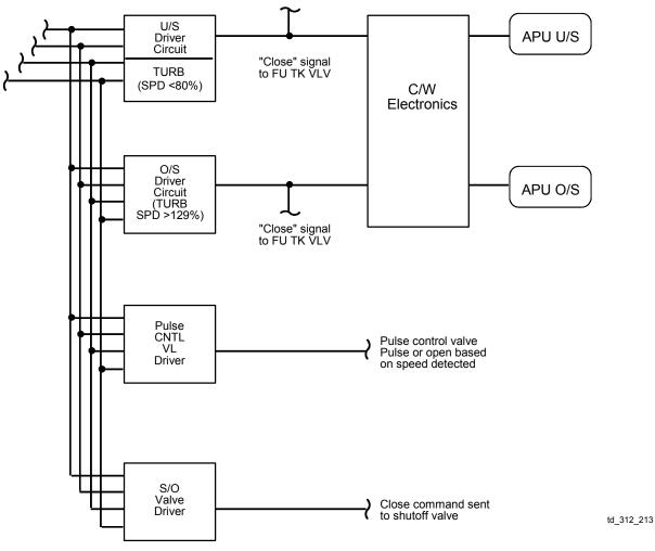
Figure 2-12. APU overspeed/underspeed detection
