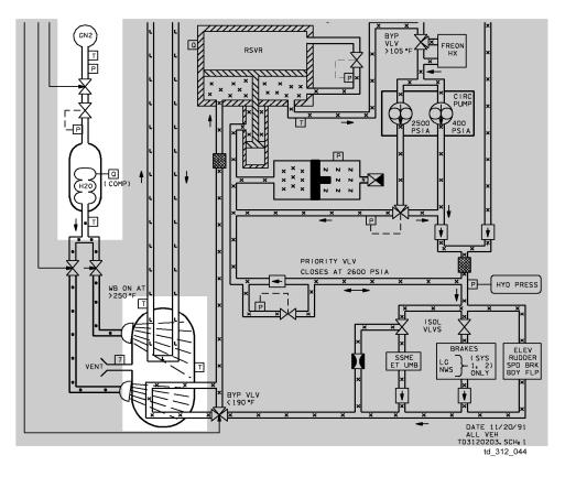
Figure 4-3. Water tank and boiler
