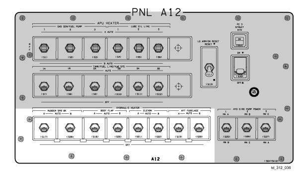
Figure 3-6. Heater switches on panel A12
