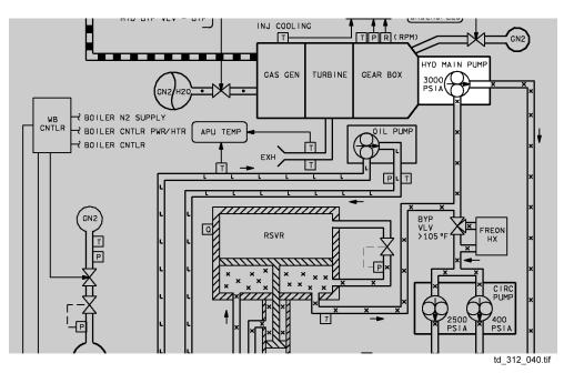
Figure 3-2. Hydraulic main pump
