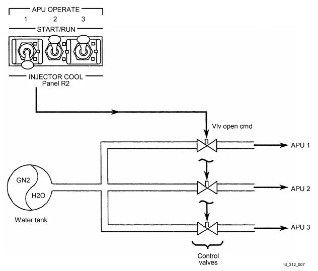
Figure 2-13. APU injector cooling
