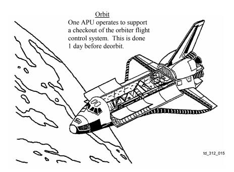
Figure 5-4. APU/HYD/WSB system use on orbit
