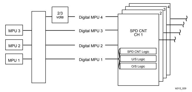
Figure 2-7. Speed control channels
