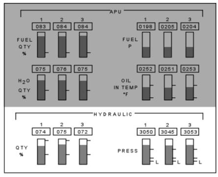
Figure 3-13. HYD/APU Subsystem Status Display meters
