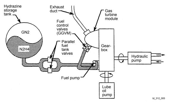
Figure 2-2. APU system layout
