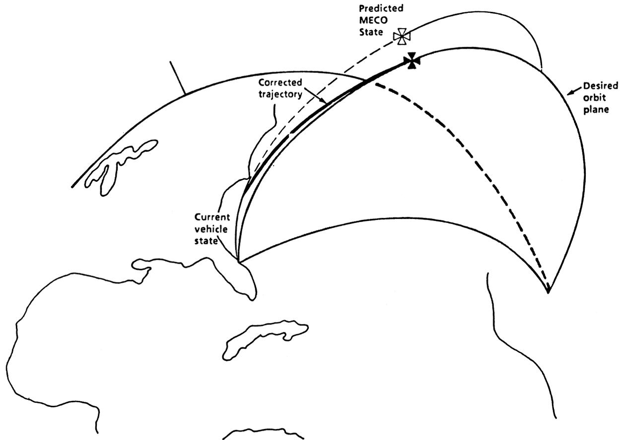
**Figure 3-15.— Orbit plane correction.**
