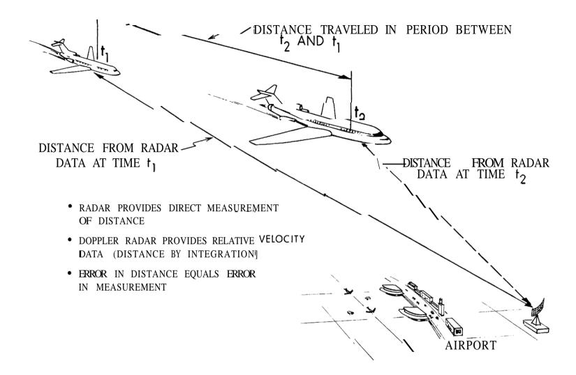
Fig. 1-4 Position Change Information from Radiation Contact Measurements
