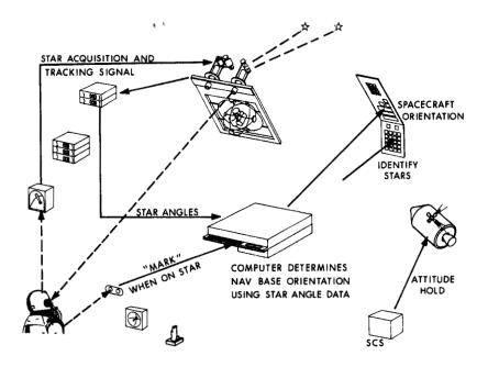
Fig. 11-50 IMU Coarse Alignment Step 1
