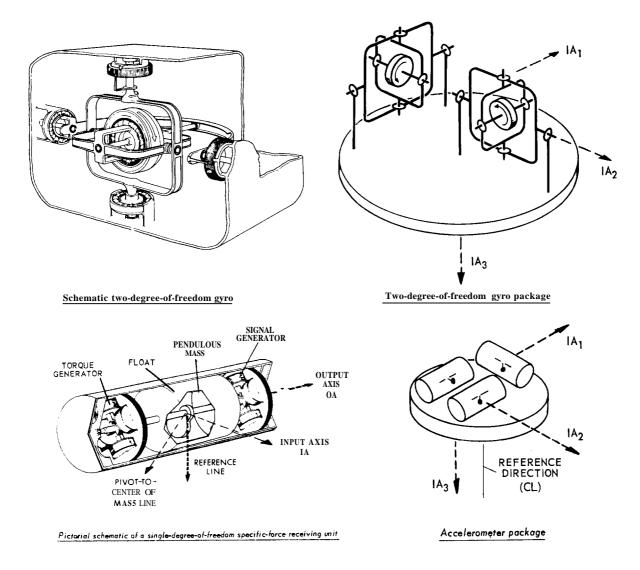
Fig. 1-40 Basic Elements of Typical Geometrical Reference Packages
