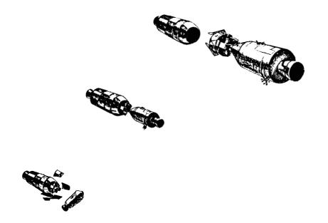
Fig. 11-14 Phase 7 - Transposition and Docking
