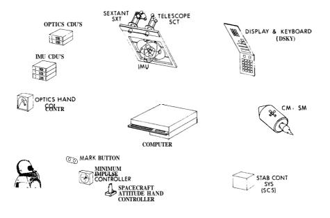
Fig. 11-48 Subsystem Identification
