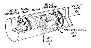
Schematic drawing of single-degree-of-freedom gyro unit
