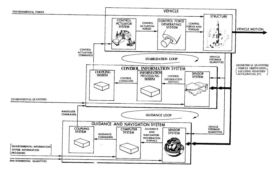
Fig. I-19 Guidance and Control System - Automatic Operator
