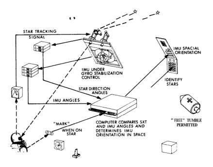
Fig. 11-52 Manual IMU Fine Alignment Step 1
