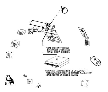
Fig. 11-60 Star Occultation by Moon - Automatic Navigation Measurement
