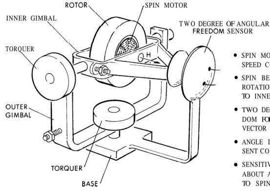
NOTE: ROTOR AND ITS BEARINGS MAY BE ENCLOSED IN A HERMETICALLY SEALED CAN AND SUBSTANTIALLY SUPPORTED BY FLOTATION IN A FLUID CONTAINED WITHIN AN OUTER CASE NSOR FEATURES
