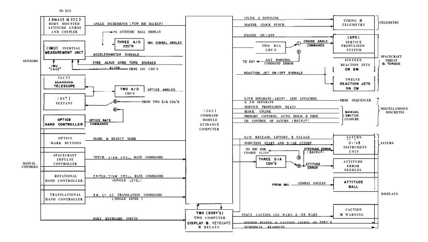
11-44 Guidance, Navigation, & Control Interconnections in Command Module
