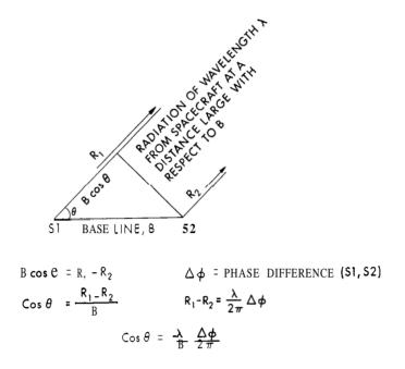
II-1 Short Base Line Interferometric Direction Measurement
