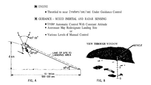
Fig. 11-22 Phase 15 - LEM Powered Descent Final Approach 6/14/65 34213
