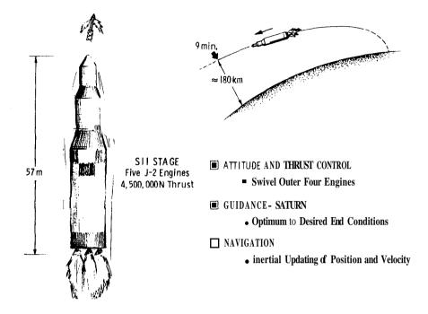
Fig, 11-10 Phase 3 - Earth Launch Second Stage
