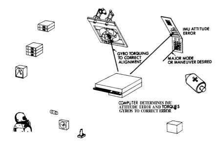
Fig. 11-53 Manual IMU Fine Alignment Step 2
