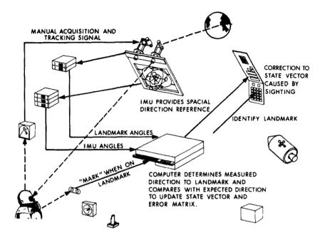
Fig. 11-54 Low Orbit Navigation - Landmark Tracking
