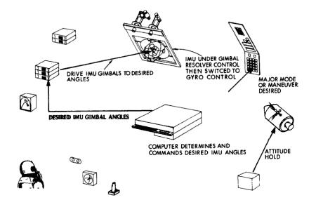
Fig. 11-51 IMU Coarse Alignment Step 2
