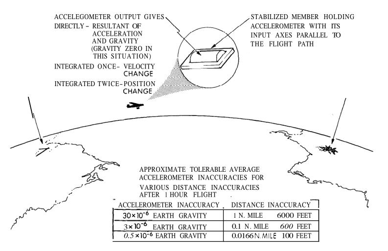
Fig. 1-6 Position and Velocity Changes from Integration of Accelerometer Measurements Taken along Flight Paths
