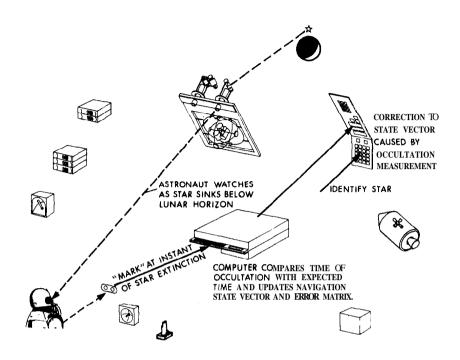
Fig. 11-61 Star Occultation by Moon - Manual Navigation Measurement
