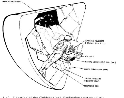
11-42 Location of the Guidance and Navigation System in the Command Module
