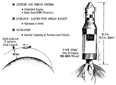
Fig. 11-11 Phase 4 - Earth Launch Third Stage
