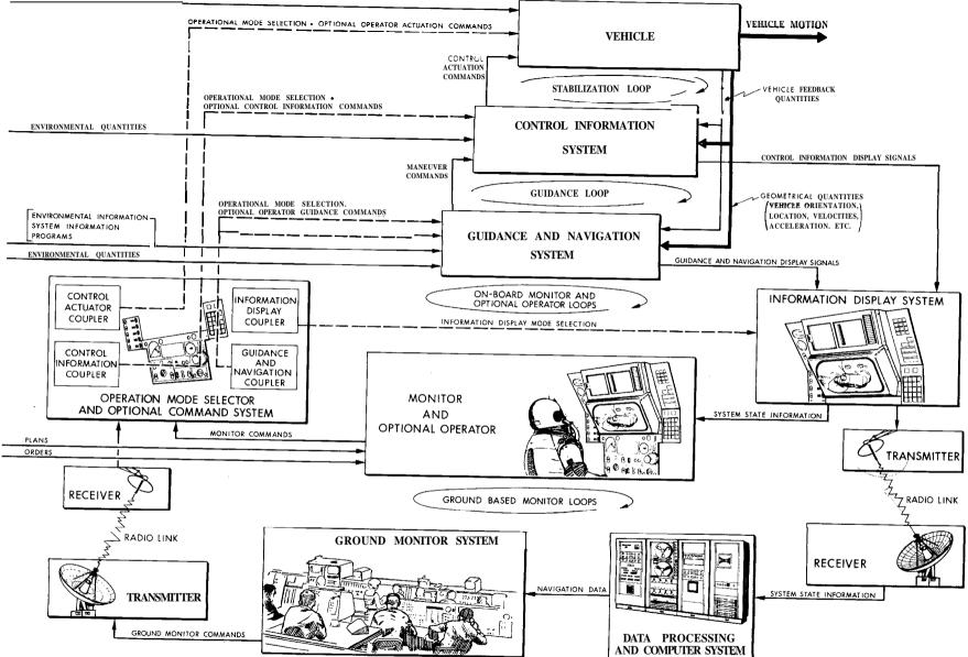
Fig. 1-23 Control and Guidance System with Ground Based Monitor
