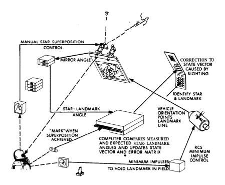
Fig. 11-55 Midcourse Navigation - Manual Star-Landmark Measurement
