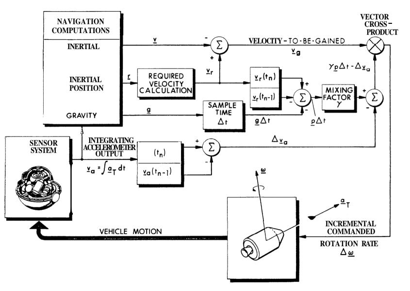
Fig. 111-8 Velocity-to-beGained Steering
