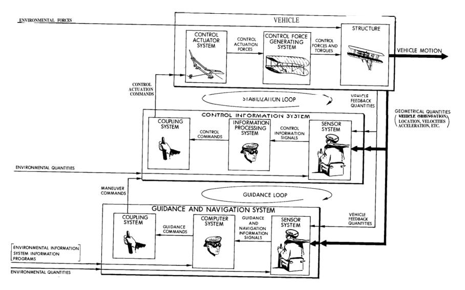
Fig. I-15 Guidance and Control System - Human Operator
