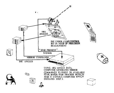
Fig. 11-58 Automatic IMU Fine Alignment - Step 1
