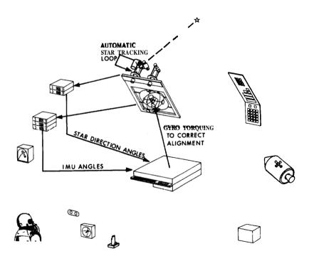
Fig. 11-59 Automatic IMU Fine Alignment - Step 2
