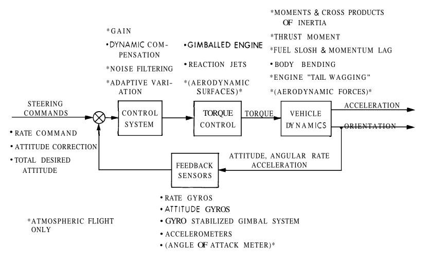
11-4 Generalization of Thrust Vector Stabilization and Control
