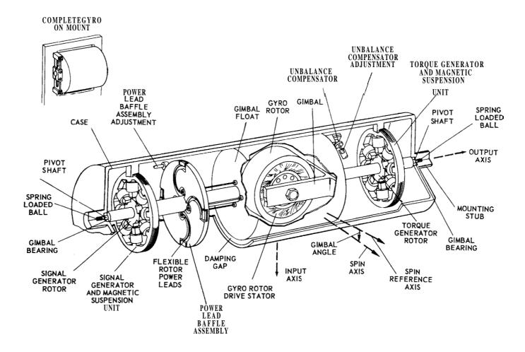
Fig. 1-34 Basic Features of Single-Degree-of-Freedom Floated Integrating Gyro Unit
