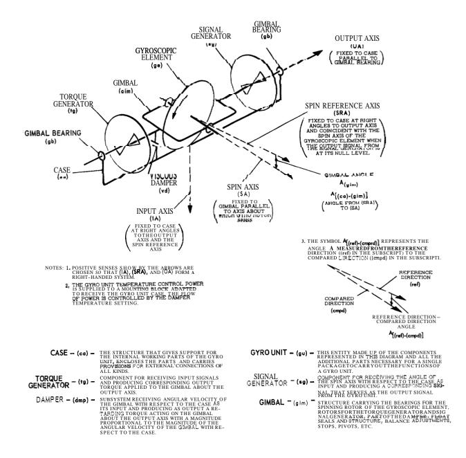
Fig, I-35 Line Schematic Diagram of Single-Degree-of-Freedom Floated Integrating Gyro Unit
