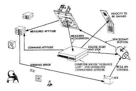
Fig, 11-49 Guidance Steering Control
