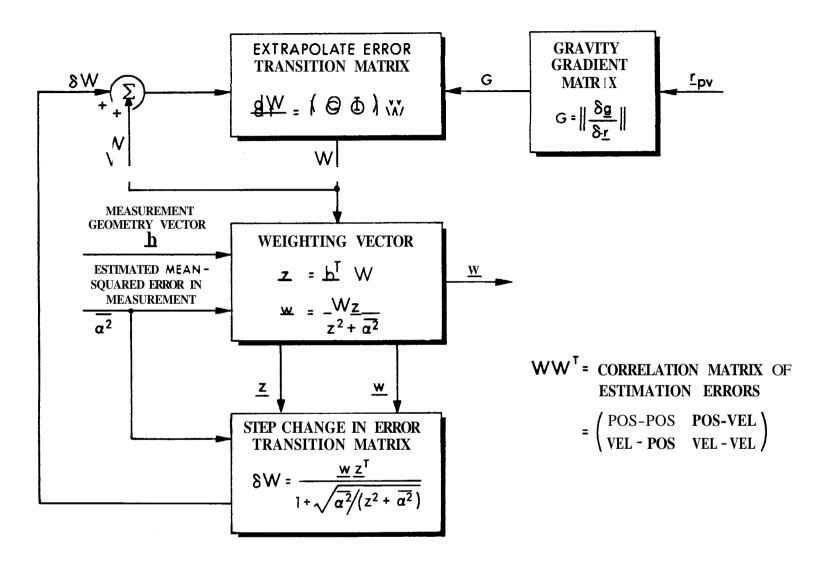
Fig. 111-5 Weighting Vector Calculation
