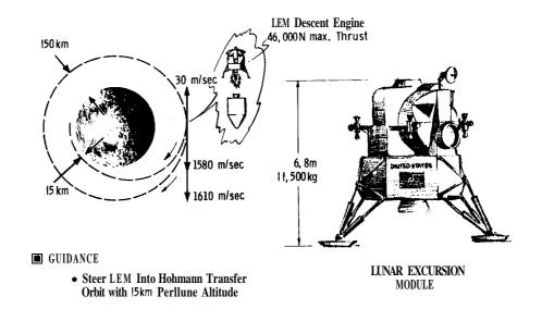
Fig. II-19 Phase 12 - LEM Descent Orbit Injection 4/19/65 36360
