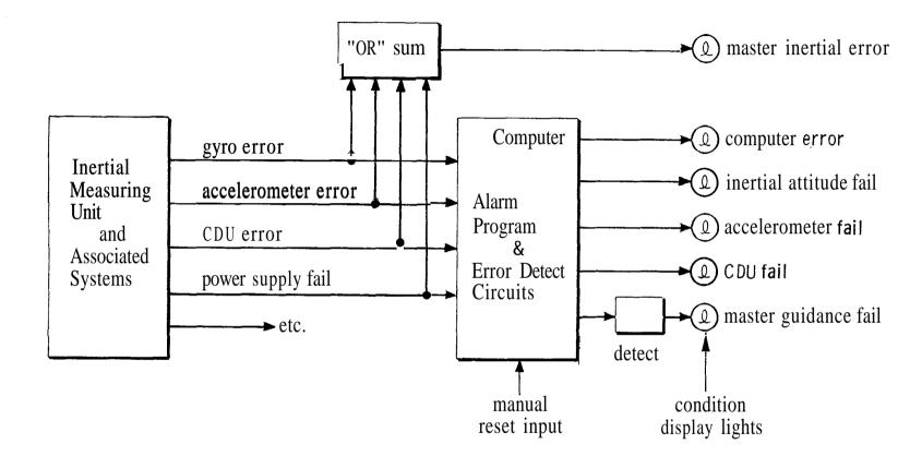
11-66 Failure Detection - Command Module Primary Guidance System
