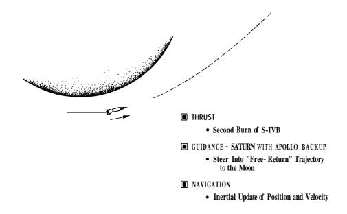
Fig. 11-13 Phase 6 - Translunar Injection
