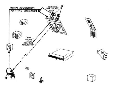
Fig. 11-56 Illuminated Horizon Manual Navigation Measurement - Step 1
