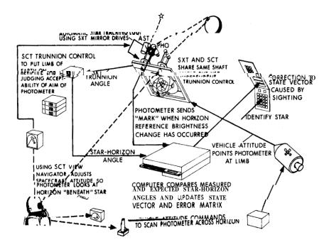
Fig. 11-57 Illuminated Horizon Manual Navigation Measurement - Step 2
