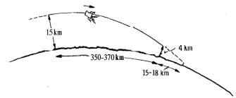
Fig. 11-21 Phase 14 - LEM Powered Descent Braking Phase
