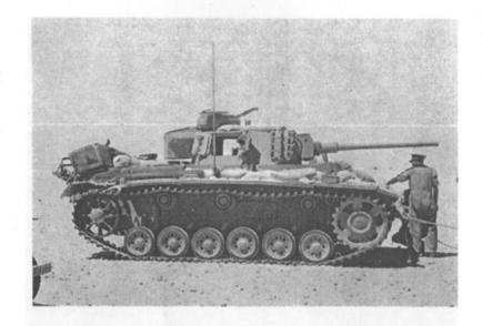
16. Pzkw III Model H with short 5-cm gun and extra plate on the front super-structure; the first of such tanks to be captured being dismantled for examination, May 1941.
