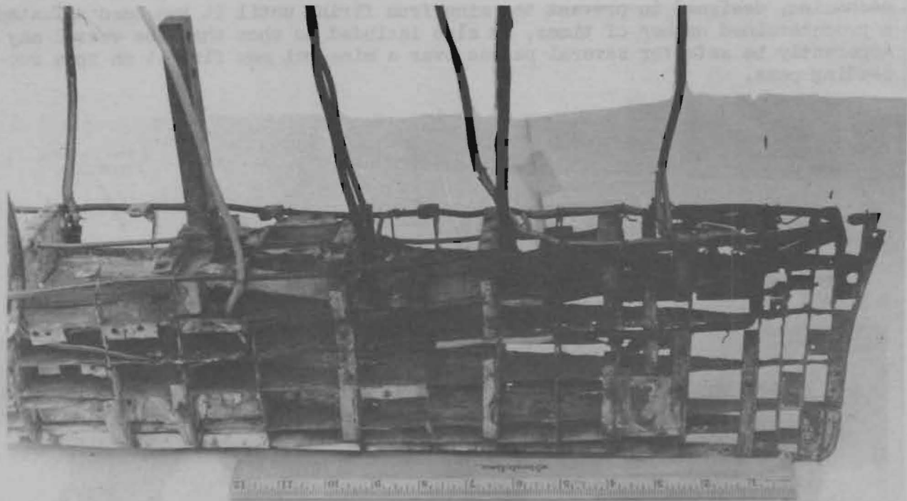
ASSEMBLED MAGNETIC SHIP MODEL SHOWING LEADS FROM EXPERIMENTAL COILS PROTRUDING THROUGH MAIN DECK
