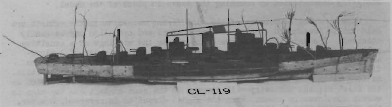
ASSEMBLED MAGNETIC SHIP MODEL SHOWING LEADS FROM EXPERIMENTAL COILS PROTRUDING THROUGH MAIN DECK
