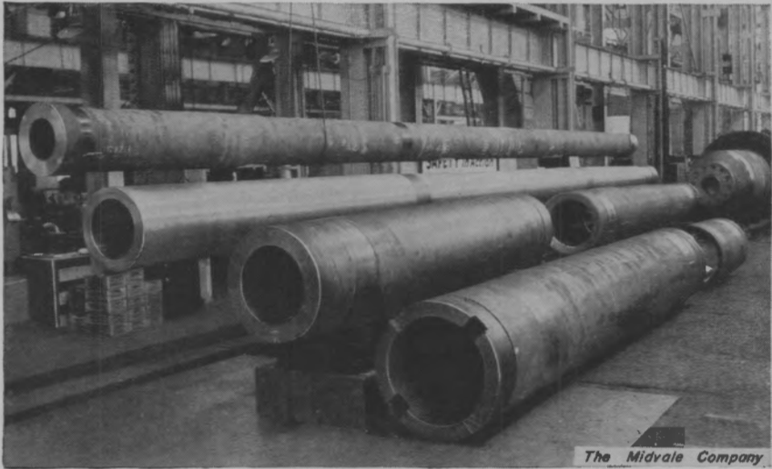
16-inch guns are constructed of layers on metal—liner, tube, jacket, and hoops.
