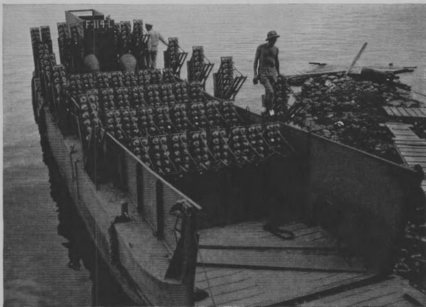
The "Woofus", or Rocket Launcher Mark 24, installed in the well of an LCM.
