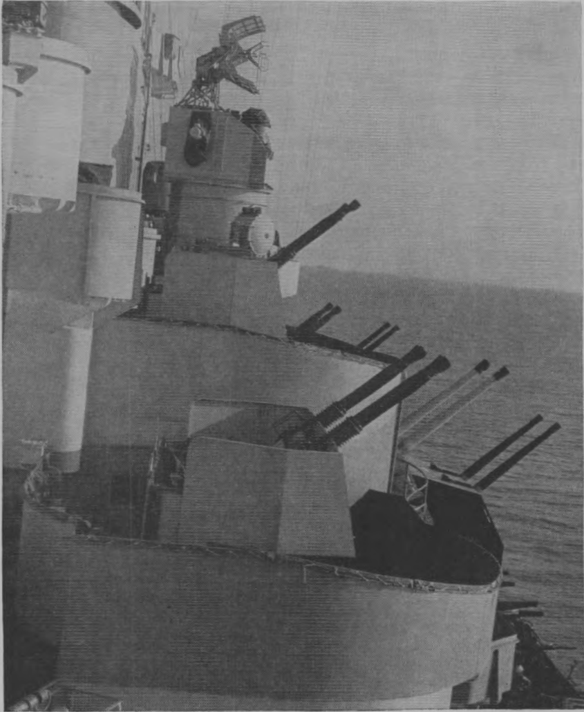
40 mm and 5"/38 guns on U. S. S. Missouri. Naval vessels were literally studded with protective anti-aircraft armament.
