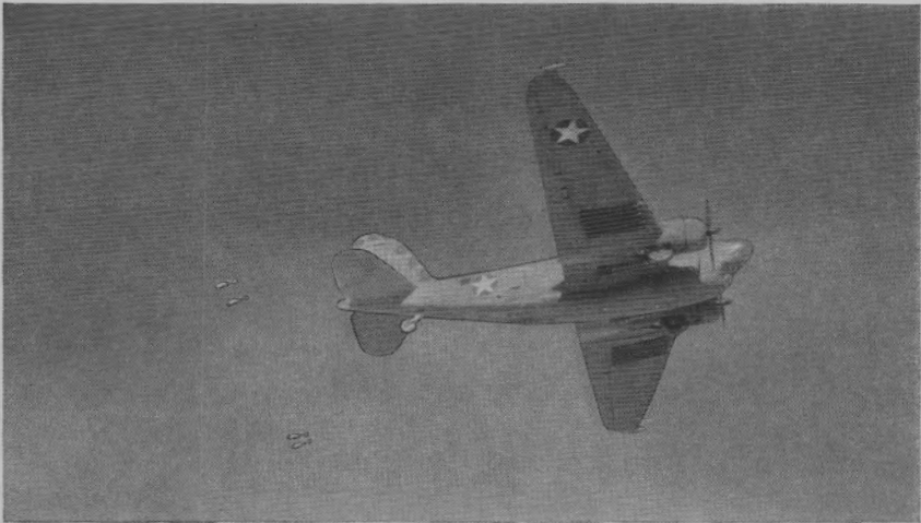
The retrobomb, a product of the desperate days when any antisubmarine armament was worth a try.
