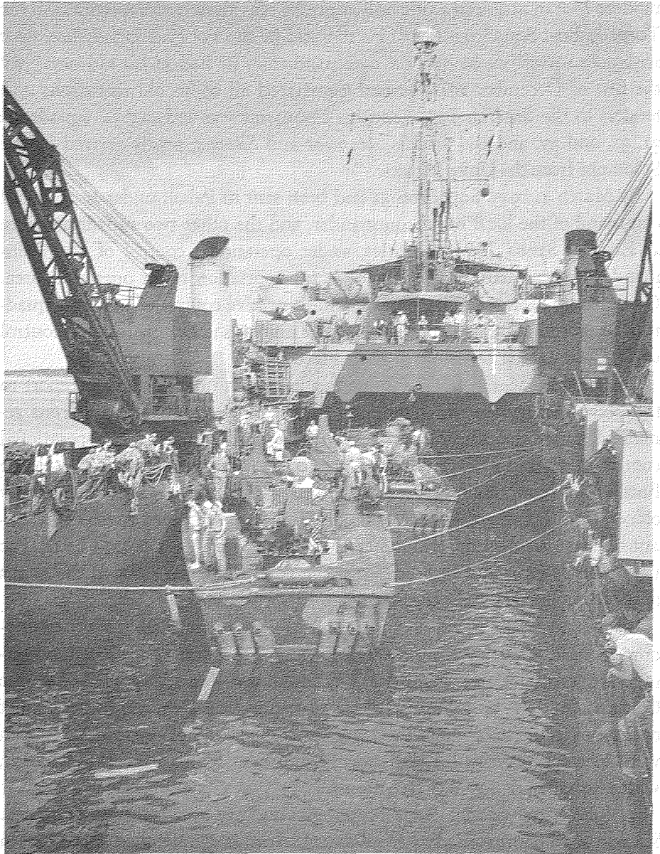
PT's of Squadron 37 being eased into their cradles in Oak Hill (LSD 7) at Espiritu Santo on July 24, 1945, for shipment to Okinawa. The LSD submerges to let the PT's enter her well deck. When six PT's are safely aboard in their cradles, the LSD refloats herself and is ready to get underway.
