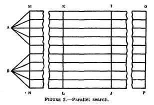
area from which objectives on or near the coast could be attacked is outlined in figure 2. The area to be searched is determined by the extent of the coast line which is to be defended against surprise attack. The extent of the area which can be searched simultaneously is limited by the number of aircraft available. The coverage of only a narrow front is shown in figure 2; the method is the same for any practicable width of front.
