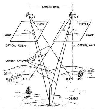
FIGURE 7.—Diagram of stereoscopic pair of aerial photographs.
