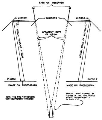
FIGURE 8.—Diagram showing stereoscopic perception.
