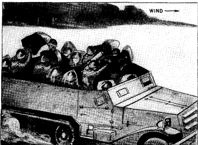
FIGURE 22.—Do not remove cellophane covers while vehicle is in motion or disregard direction of wind. Men on down wind side who first remove covers will be contaminated by the covers of the men on up wind side.
