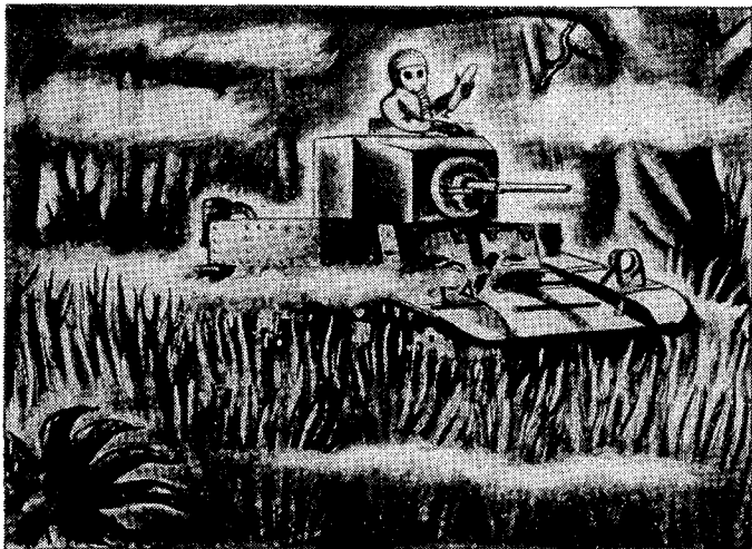
FIGURE 6.—Do not stop the tank as soon as it is contaminated. Continue until out of the contaminated area. If you decontaminate while in the area, tank will be recontaminated from vegetation when you start.
