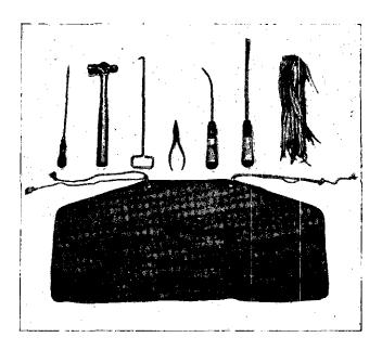
FIGURE 4. Tool roll, Phillips pack saddle.
