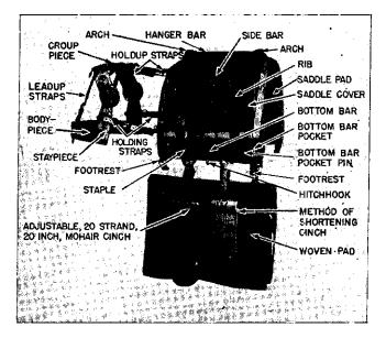
FIGURE 2. Phillips pack saddle, cargo, assembled.
