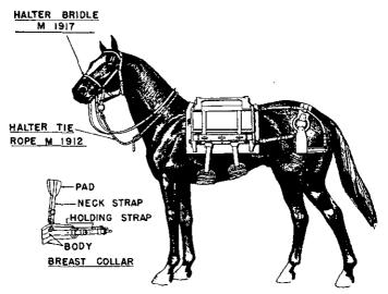
FIGURE 1. Phillips pack saddle, cavalry.
