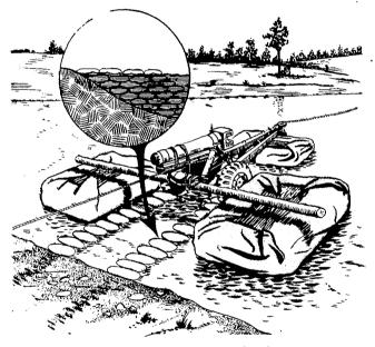
Figure 11. Flotation of howitzer.
