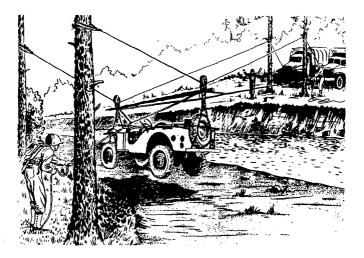
Figure 15. Aerial cableway showing movement of 4-ton truck by double-cable crossing.
