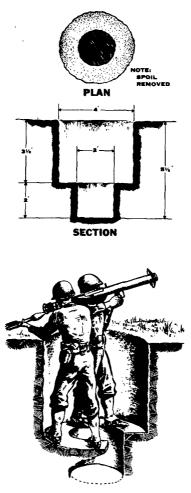
Figure 6. Pit-type emplacement for rocket launcher.
