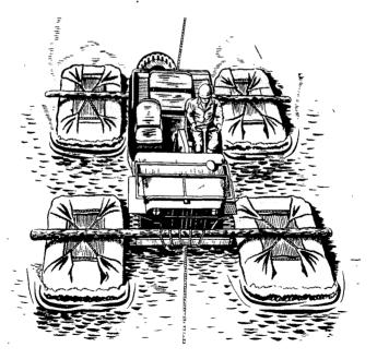
Figure 12. Flotation of <sup>1</sup>/<sub>4</sub>-ton truck on brush raft.
