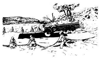
Figure 13. Flotation of 11/2-ton truck with tarpaulin.
