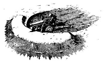
Figure 4. Development of circular emplacement for howitzer.
