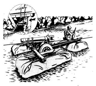
Figure 10. Flotation of howitzer.
