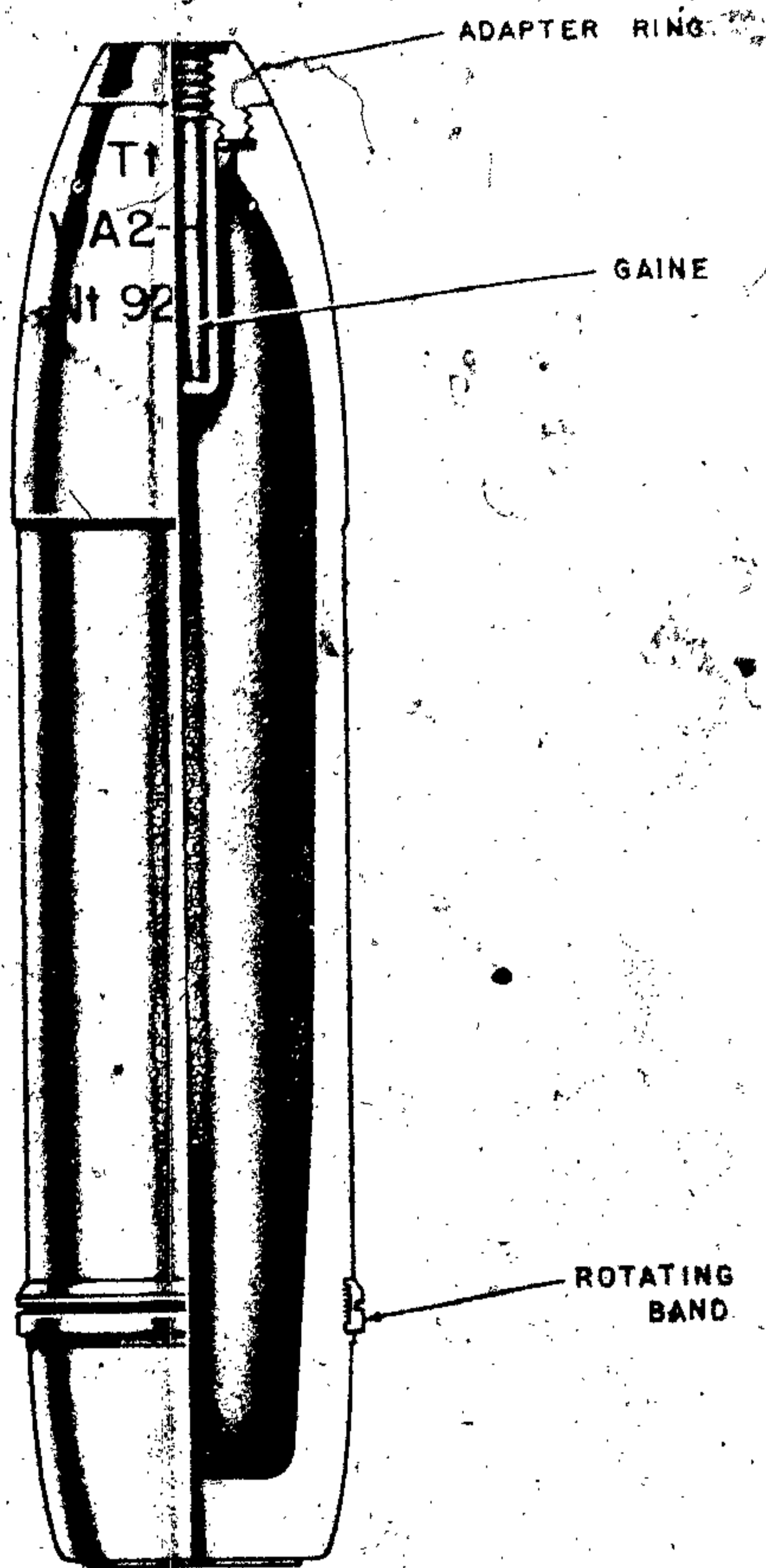
Figure 447—H. E. Projectile for 100-mm Howitzer, 10-cm Stg. Gr. (p)
