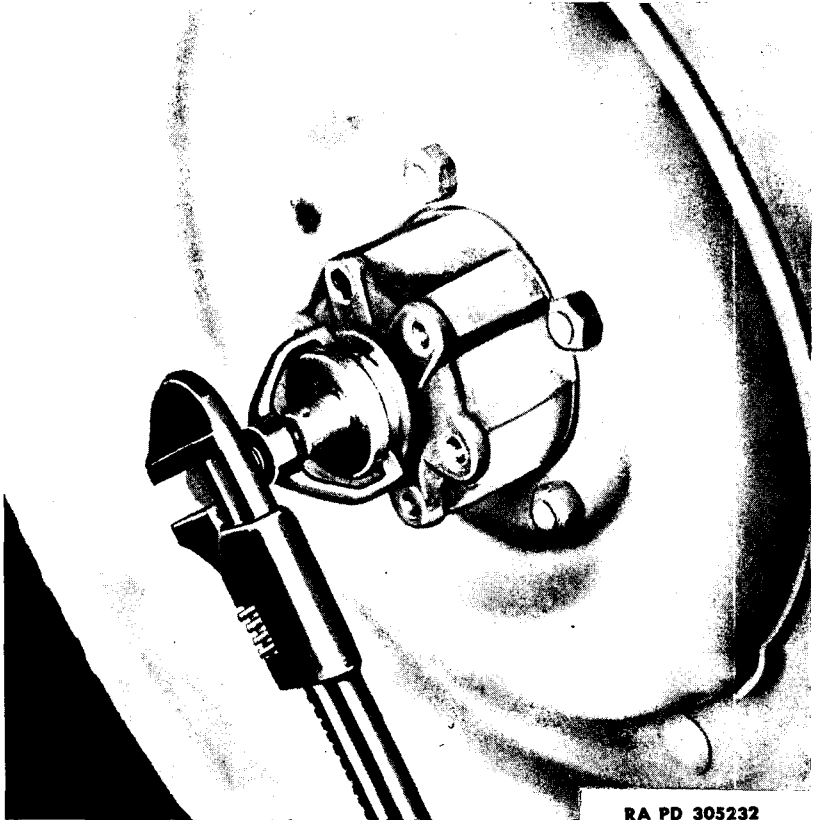
Figure 77—Removing Driving Flange, Using Puller (41-P-2905-60)
