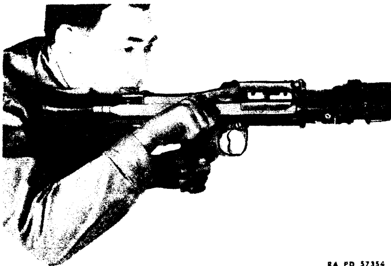
Figure 30 — Cocking Handle in Forward Position — Gun Cocked
