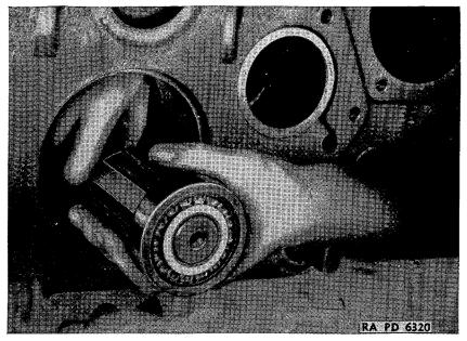
FIGURE 123.—Transfer case mainshaft removal.
