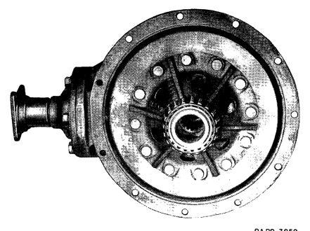
RAPD 3859 FIGURE 27.—Front axle differential assembly, installed.
