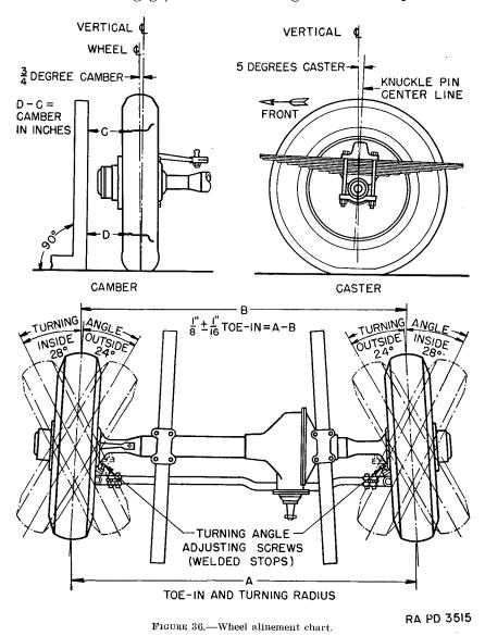
less than 0° reverse, it is an indication that some part has been bent or excessively worn and should be replaced. (2) Caster.—This is the amount in degrees that steering knuckle pins are tilted toward rear or front of vehicles. Positive caster is inclination of top of knuckle pin toward rear of vehicle; zero caster is vertical position of pins; and negative or reverse caster is an inclination of top of pins toward front of vehicle.
