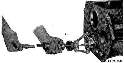
FIGURE 105.--Transmission countershaft rear bearing removal.
