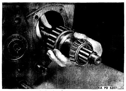
FIGURE 115.-Transfer case front-drive shaft removal.
