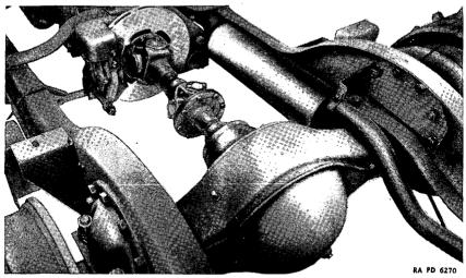
FIGURE 43.-Rear axle (jackshaft) assembly, installed.
