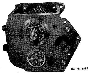
FIGURE 100.-Transmission rear bearings, installed.
