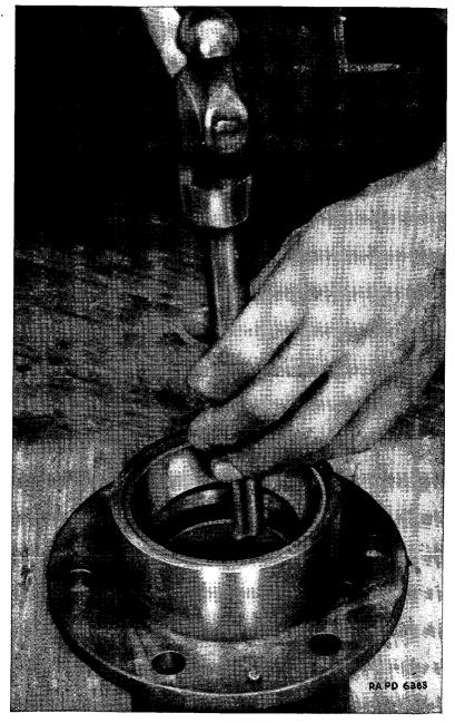
FIGURE 24 .- Front axle drive pinion bearing cup removal.
