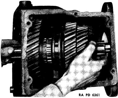
FIGURE 102.-Transmission mainshaft removal.
