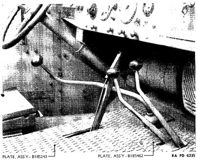
FIGURE 80.-Transmission shift levers and floor plates, installed.
