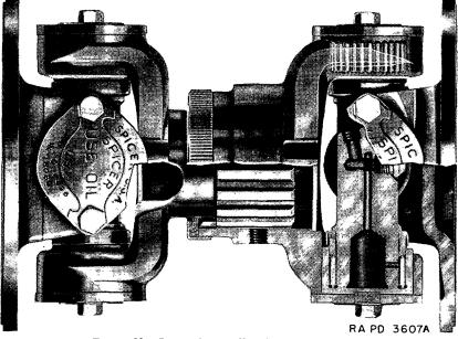
FIGURE 69.-Rear axle propeller shaft, sectionalized.
