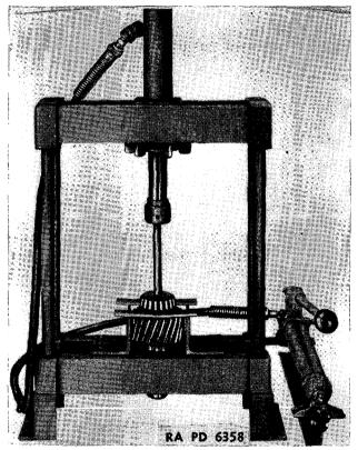
FIGURE 129.—Pressing rear bearing off intermediate shaft.
