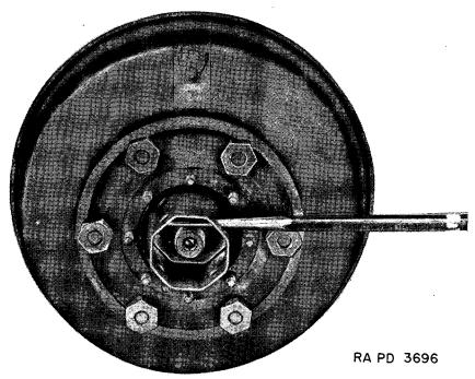
FIGURE 12.—Front axle wheel bearing nut removal.
