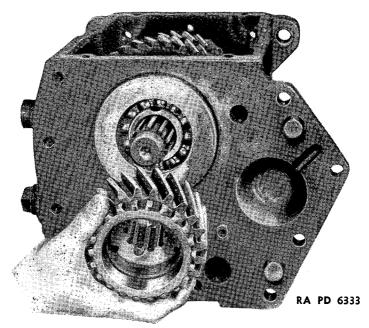
FIGURE 99.—Transmission drive gear removal.
