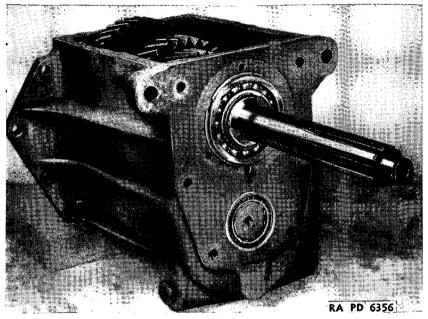
FIGURE 94.-Transmission main drive gear, installed.
