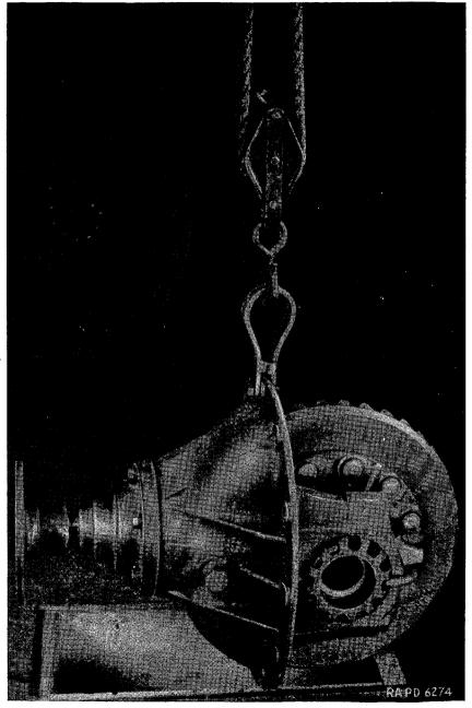
FIGURE 50.-Differential assembly removal using special fixture.
