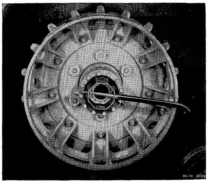
FIGURE 48.-Rear axle drive sprocket bearing nut removal.
