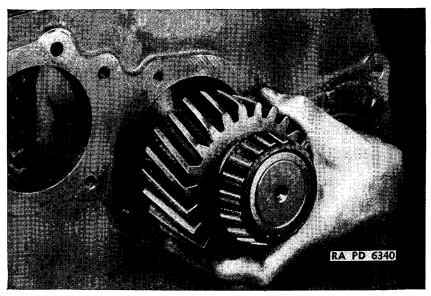
FIGURE 119.-Transfer case intermediate shaft removal.
