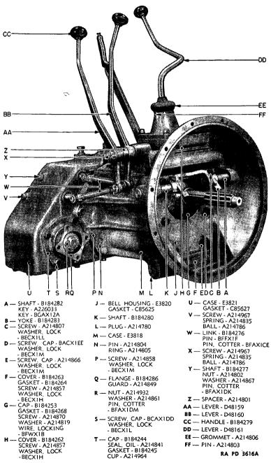
FIGURE 77.-Transmission assembly, right side.
