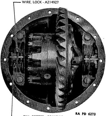
PIN. COTTER - BFAX2AK FIGURE 56.—Rear axle differential and ring gear dismounted, top view.
