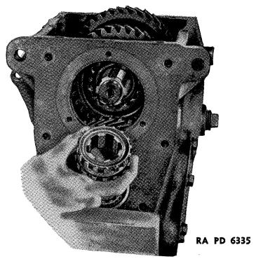
FIGURE 97.-Transmission third and fourth speed clutch gear removal.
