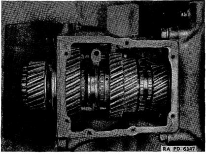
FIGURE 92.-Transmission gears installed.
