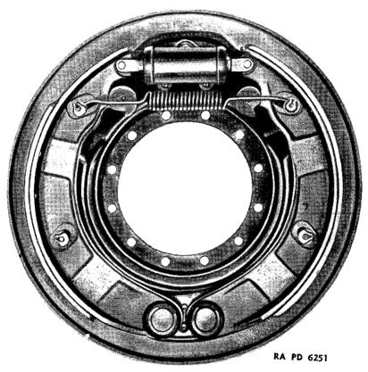
FIGURE 16.-Front wheel brake assembly.
