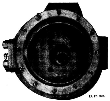
FIGURE 18 .- Front axle Rzeppa universal joint housing.
