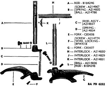
FIGURE 125.-Transfer case shifting mechanism, exploded.
