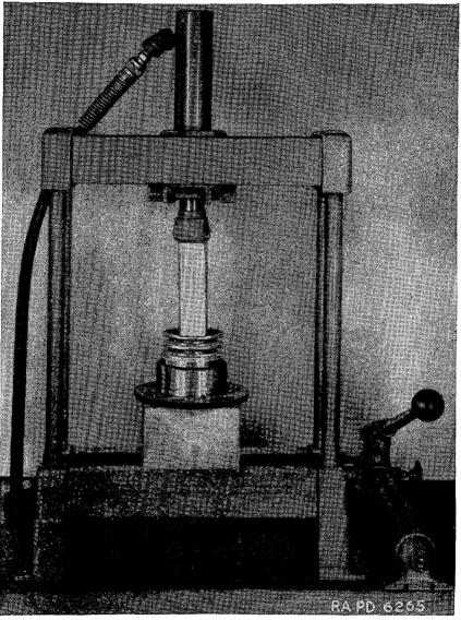
FIGURE 41.-Front axle drive pinion bearing cup replacement.
