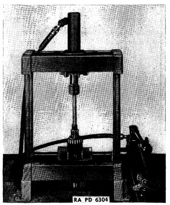
FIGURE 128 --- Pressing front bearing off front-drive shaft.
