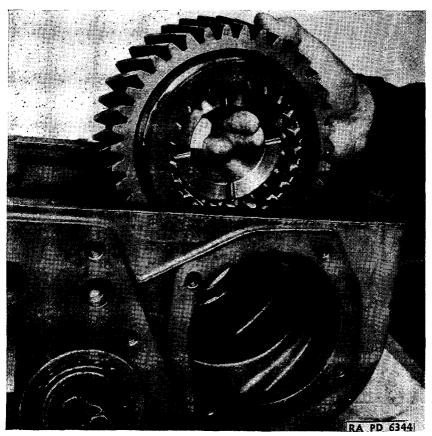
FIGURE 116.-Transfer case front-drive shaft gear removal.
