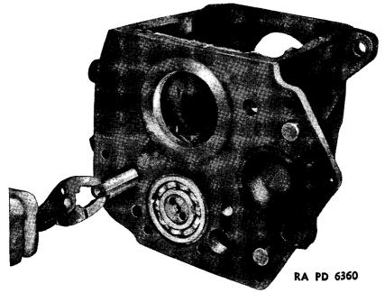
FIGURE 103.---Transmission reverse idler gear shaft removal.
