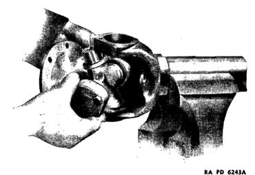
FIGURE 73.—Propeller shaft universal joint journal removal.
