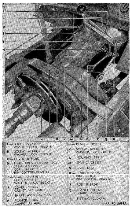
FIGURE 83.-Transmission assembly, installed.
