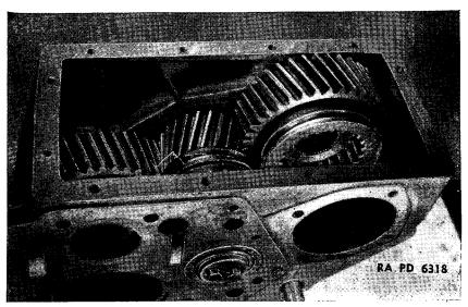
FIGURE 135. Transfer case front-drive shaft gear replacement.
