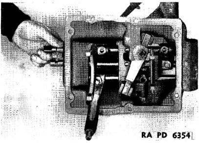
FIGURE 91.- Transmission reverse shift rod removal.
