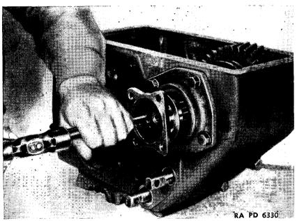
FIGURE 141.—Transfer case front-drive shaft companion flange replacement.
