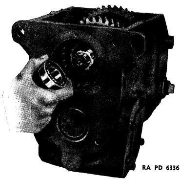
FIGURE 96. -Transmission mainshaft pilot bearing removal.
