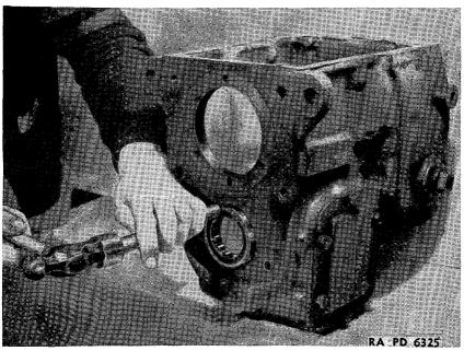
FIGURE 148.-Transmission countershaft front bearing replacement.
