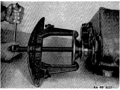
FIGURE 122.—Transfer case mainshaft companion flange removal.
