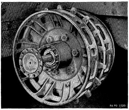
FIGURE 47.---Rear axle drive shaft removal.
