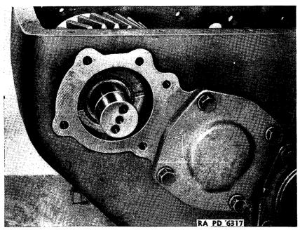
FIGURE 136.-Transfer case front-drive shaft, installed.
