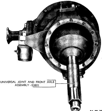
FIGURE 17.-Front axle Rzeppa universal joint removal.
