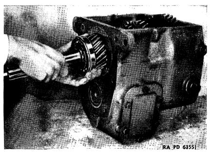
FIGURE 95.-Transmission main drive gear removal.
