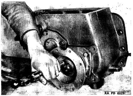
FIGURE 142.-Transfer case mainshaft companion flange replacement.
