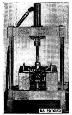
FIGURE 108.-Pressing off countershaft power take-off gear.
