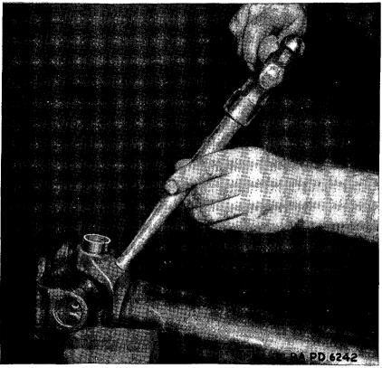
FIGURE 72.—Propeller shaft universal joint needle bearing removal.
