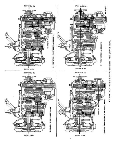
manually shifted by the operator. When shifting, the poppet springs are depressed and the balls slip from one recess to another as required. The eight interlock balls between the shift rods lock either one, or two, of the three shift rods in their neutral position
