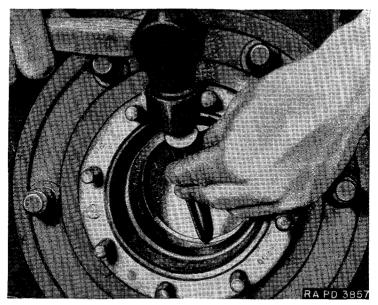
FIGURE 14.—Front axle wheel bearing inner cup removal.
