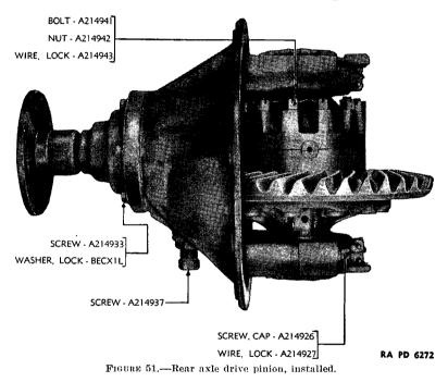
moved from carrier without disassembling carrier from axle. However, since it is usually necessary to remove differential at same time, the drive pinion is usually removed as a unit with the carrier.
