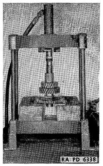
FIGURE 145.--Pressing on transmission countershaft power take-off gear.
