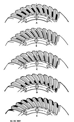
FIGURE 35.—Gear tooth bearing surface contact adjustment.
