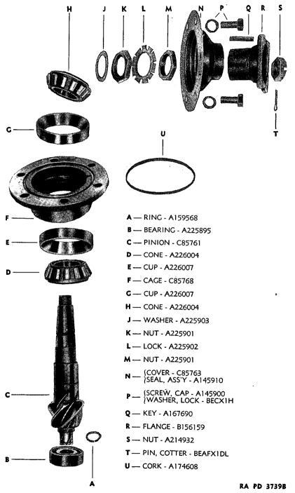
FIGURE 39.-Front axle drive pinion, exploded.
