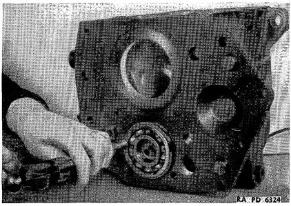
FIGURE 149.-Transmission countershaft rear bearing replacement.
