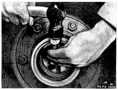
FIGURE 15.—Front axle wheel bearing outer cup removal.
