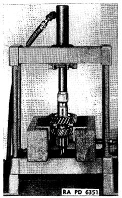
FIGURE 109 .--- Pressing off countershaft third speed gear.
