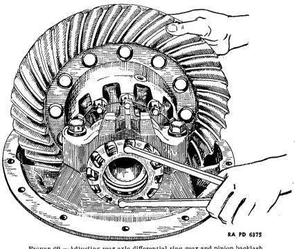
FIGURE 60.-Adjusting rear axle differential ring gear and pinion backlash.
