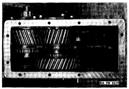
FIGURE 134.-Transfer case mainshaft and intermediate shaft, installed.
