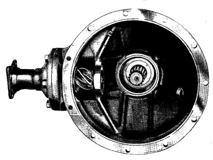
FIGURE 28.—Front axle drive pinion, installed.
