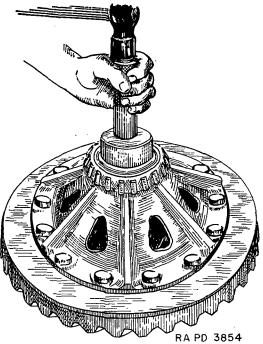
FIGURE 38.—Front axle differential bearing cone replacement.
