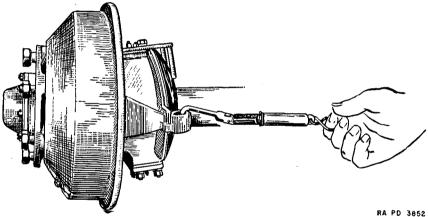
FIGURE 34.—Checking front axle steering knuckle drag.
