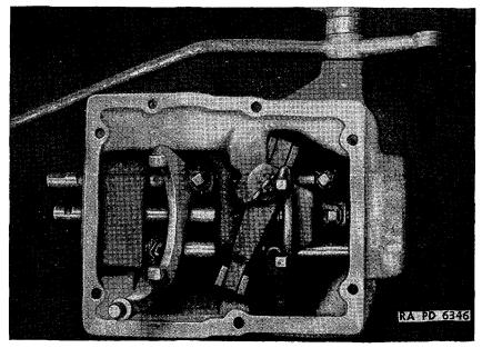
FIGURE 87.-Transmission shifter mechanism, bottom view.
