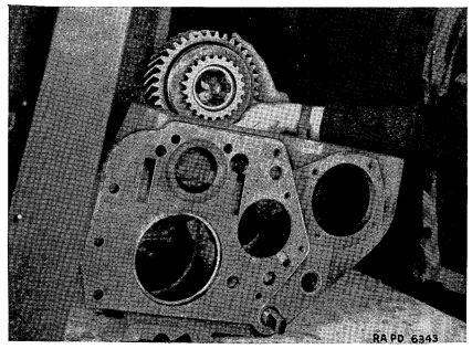
FIGURE 124.-Transfer case mainshaft underdrive gear removal.
