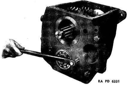
FIGURE 101.-Transmission lower shift fork guide rod removal.
