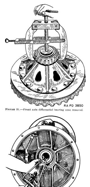
FIGURE 32.—Front axle tube oil seal removal.
