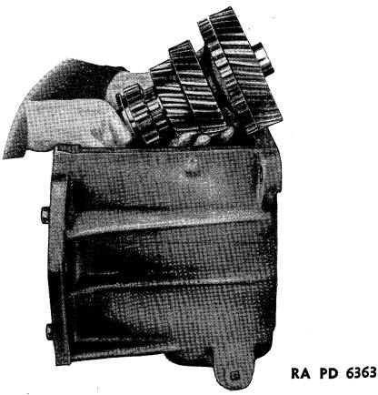
FIGURE 106.-Transmission countershaft removal.
