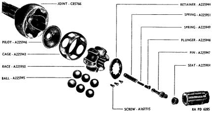
FIGURE 19.-Front axle Rzeppa universal joint, exploded.
