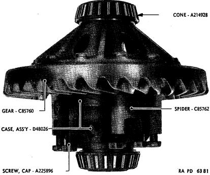
FIGURE 29.--Front axle differential case cap screw removal.
