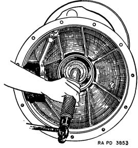
FIGURE 37.-Front axle tube oil seal replacement.
