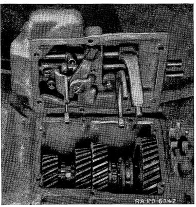
FIGURE 85.—Transmission shifter mechanism removal.
