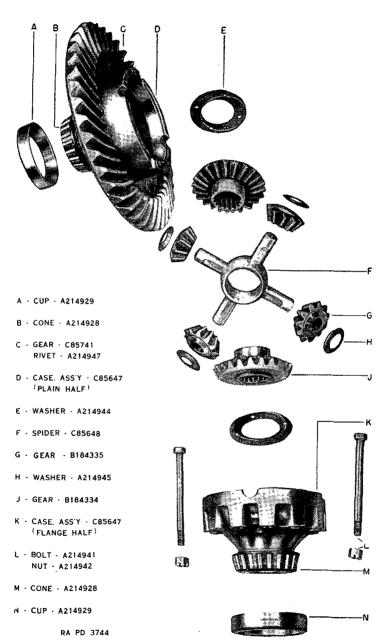
FIGURE 58.-Rear axle differential case assembly, partially exploded.
