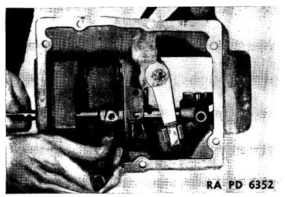
FIGURE 89 .--- Transmission first and second speed shift rod removal.
