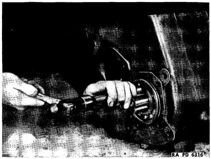
FIGURE 132.—Transfer case mainshaft rear bearing replacement.
