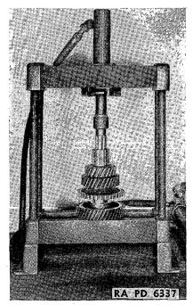
FIGURE 146.-Pressing on transmission countershaft drive gear.
