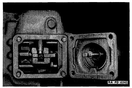
FIGURE 86.-Transmission shifter mechanism, top view.
