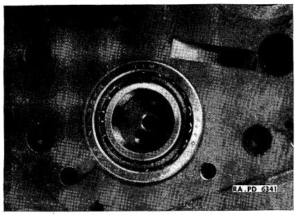
FIGURE 118.—Transfer case intermediate shaft in front bearing.
