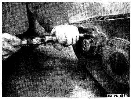
FIGURE 138.-Transfer case front-drive shaft rear bearing cup replacement.
