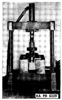
FIGURE 144 .- Pressing on transmission countershaft third speed gear.
