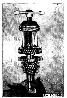
FIGURE 107 .- Pulling transmission countershaft drive gear.
