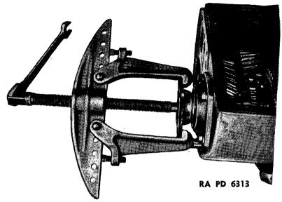
FIGURE 112.-Transfer case front-drive shaft companion flange removal.
