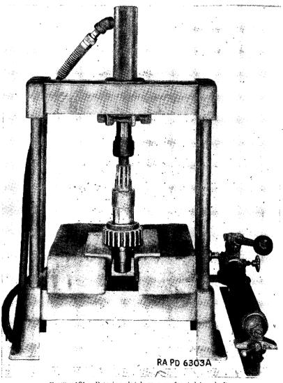
FIGURE 131.-Pressing clutch gear on front drive shaft.
