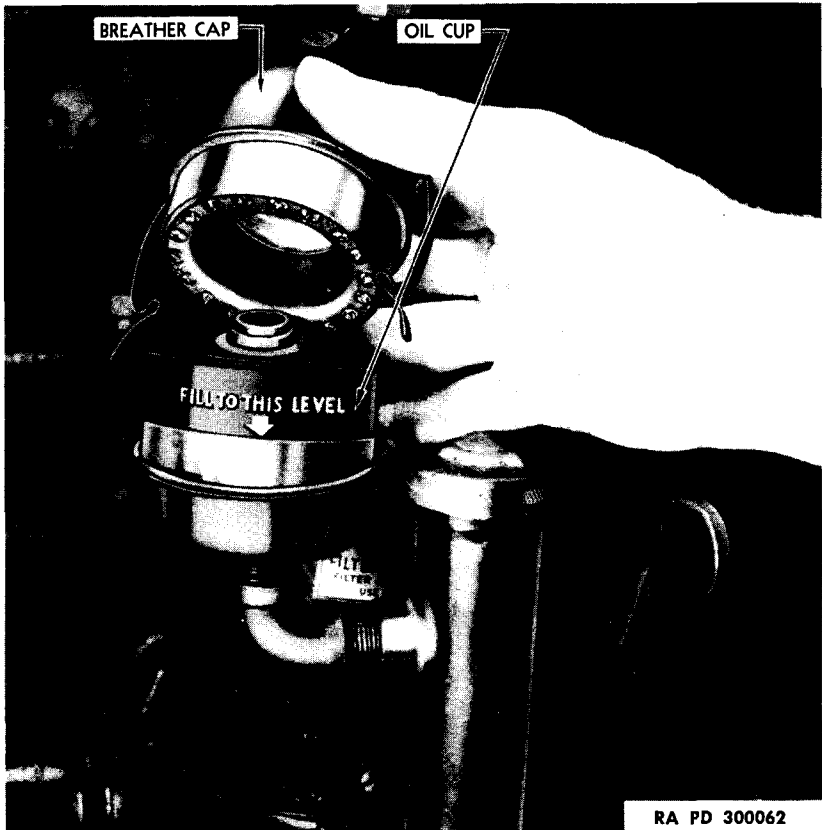
Figure 29—Crankcase Ventilator and Air Cleaner
