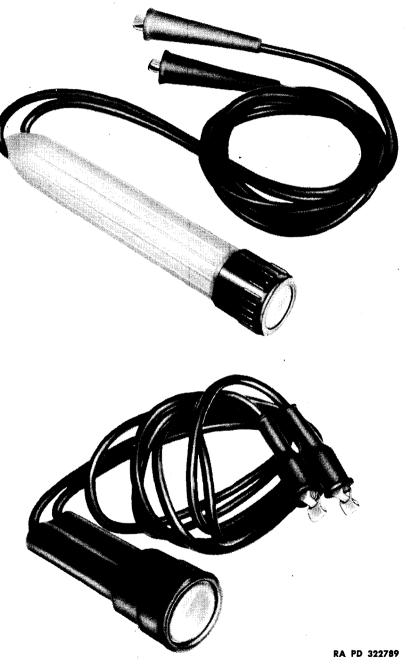
Figure 8—Neon Timing Lights
