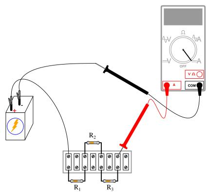
If your resistor values are indeed between  $1 \ k\Omega$  and  $100 \ k\Omega$ , and the battery voltage approximately 6 volts, the current should be a very small value, in the milliamp (mA) or microamp ( $\mu$ A) range. When you measure current with a digital meter, the meter may show the appropriate metric prefix symbol (m or  $\mu$ ) in some corner of the display. These metric prefix telltales are easy to overlook when reading the display of a digital meter, so pay close attention!
