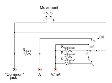
$\ensuremath{^{\text{"}}} R_{\text{multiplier}}\ensuremath{^{\text{"}}}$  resistors are actually rheostat networks
