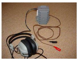
As you can see, I built my detector using scrap parts (household electrical switch/receptacle box for the enclosure, section of brown lamp cord for the test leads). Even some of the internal components were salvaged from scrap (the step-down transformer and headphone jack were
