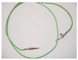
The home-made jumper wires with large, uninsulated (bare metal) alligator clips are okay
