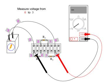
Using the voltmeter to "step" around the circuit in this manner yields three positive voltage figures and one negative:  $\frac{1}{2}$
