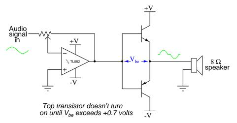
Bottom transistor doesn't turn on until V<sub>be</sub> drops below -0.7 volts
