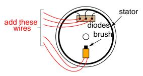
I recommend that you solder ring-lug terminals to your wires, and attach them underneath the terminal nuts along with the stator wire ends, so that each diode block terminal is securing two ring lugs.
