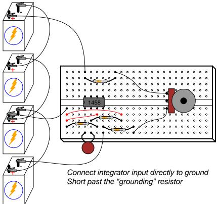
As soon as the "grounding" resistor is shorted with a jumper wire, the op-amp's output voltage will start to change, or drift. Ideally, this should not happen, because the integrator
