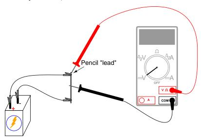
Move the black test probe position along the length of the rod, noting the voltmeter indica-
