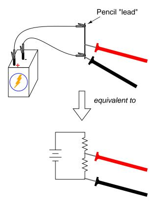
Now, change the voltmeter connection to the circuit so as to measure voltage across the "upper resistor" of the pencil lead, like this:
