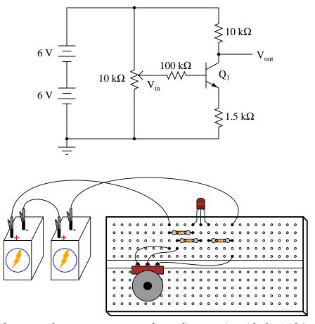
Repeat the same voltage measurement and recording exercise with the 1.5 k $\Omega$  resistor installed, calculating the new (reduced) voltage gain. Try altering the transistor's temperature again and noting the output voltage for a steady input voltage. Does it change more or less than without the 1.5 k $\Omega$  resistor?
