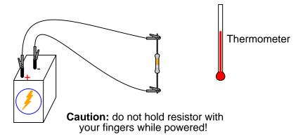
Measure each resistor's resistance with your ohmmeter, noting the exact values on a piece of paper for later reference.
