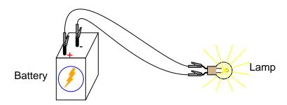
This is the simplest complete circuit in this collection of experiments: a battery and an incandescent lamp. Connect the lamp to the battery as shown in the illustration, and the lamp should light, assuming the battery and lamp are both in good condition and they are matched to one another in terms of voltage.
