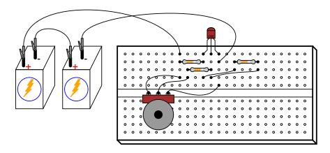
Although this different method of feedback accomplishes the same goal of increased stability by diminishing gain, the two feedback circuits will not behave identically. Note the range of possible output voltages with each feedback scheme (the low and high voltage values obtained with a full sweep of the input voltage potentiometer), and how this differs between the two circuits.
