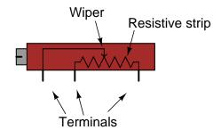
It should be noted that not all linear potentiometers have the same pin assignments. On some, the middle pin is the wiper.
