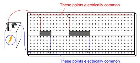
With so many of these integrated circuits having "reset," "enable," and "disable" terminals needing to be maintained in a "high" or "low" state, not to mention the  $V_{\rm DD}$  (or  $V_{\rm CC}$ ) and ground power terminals which require connection to the power supply, having both terminals of the power supply readily available for connection at any point along the board's length is very useful.
