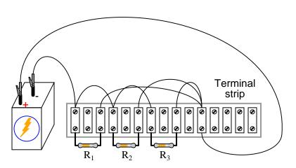
Normally, it is considered improper to secure more than two wires under a single terminal strip screw. In this illustration, I show three wires joining at the top screw of the rightmost lug used on this strip. This is done for the ease of proving a concept (of current *summing* at a circuit node), and does not represent professional assembly technique.
