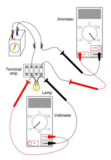
Measure the resistance of the lamp with your multimeter. This resistance figure is due to the thin metal "filament" inside the lamp. It has substantially more resistance than a jumper wire, but less than any of the resistors from the last experiment. Record this resistance value for future use.
