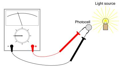
Experiment with measuring the resistance of several different types of materials, just be sure not to try measure anything that produces substantial voltage, like a battery. Suggestions for materials to measure are: fabric, plastic, wood, metal, clean water, dirty water, salt water, glass, diamond (on a diamond ring or other piece of jewelry), paper, rubber, and oil.
