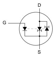
In the case of the JFET, it is the *voltage* across the reverse-biased gate-source diode which sets the current regulation point for the pair of constant-current diodes. A pair of opposing constant-current diodes is included in the model to facilitate current in either direction be-
