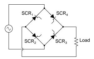
Figure 7.35: Controlled bridge rectifier
