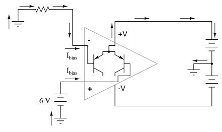
Without a ground reference on the power supply, the bias currents will have no complete path for a circuit, and they will halt. Since bipolar junction transistors are current-controlled devices, this renders the input stage of the op-amp useless as well, as both input transistors will be forced into cutoff by the complete lack of base current.
