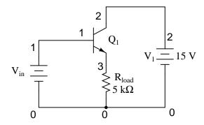
Figure 4.41: Common collector amplifier for SPICE.
