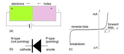
Figure 2.30: (a) Forward biased PN junction, (b) Corresponding diode schematic symbol (c) Silicon Diode I vs V characteristic curve.
