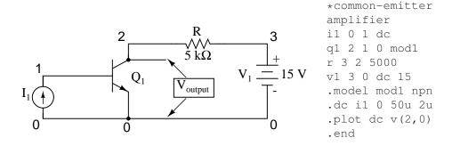
Figure 4.25: Common emitter schematic with node numbers and corresponding SPICE netlist.
