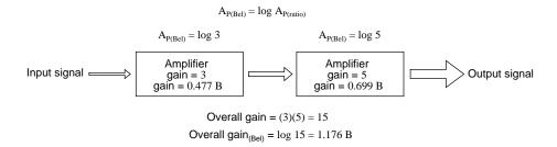
Figure 1.7: Power gain in bels is additive: 0.477 B + 0.699 B = 1.176 B.
