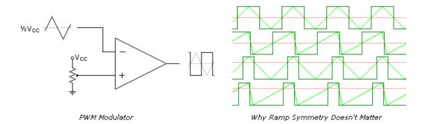
If there isn't any computation involved PWM can be fast. The limiting factor is the comparators frequency response. This may not be an issue since quite a few of the uses are fairly low speed. Some microcontrollers have PWM built in, and can record or create signals on demand.
