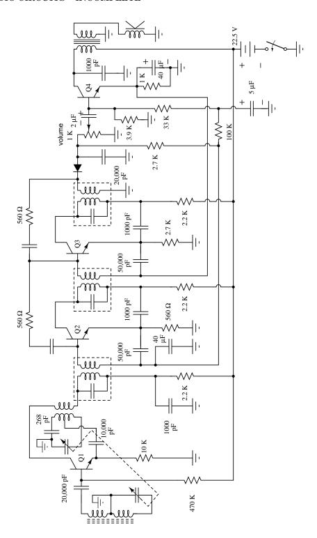
Figure 9.14: Regency TR1: First mass produced transistor radio, 1954.
