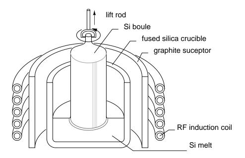
Figure 2.51: Czochralski monocrystalline silicon growth.
