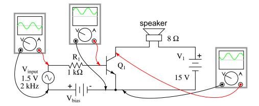
Figure 4.34: Input is biased upward at base. Output is inverted.
