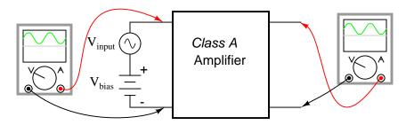
Figure 4.65: Class A: The amplifier output is a faithful reproduction of the input.
