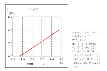
Figure 4.42: Common collector: Output equals input less a 0.7 V  $V_{BE}$  drop.
