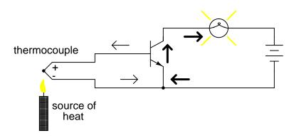
Figure 4.6: A single thermocouple provides less than 40 mV. Many in series could produce in excess of the 0.7 V transistor  $V_{\rm BE}$  to cause base current flow and consequent collector current to the lamp.
