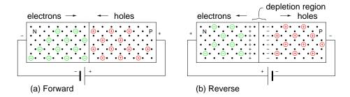
Figure 2.29: (a) Forward battery bias repels carriers toward junction, where recombination results in battery current. (b) Reverse battery bias attracts carriers toward battery terminals, away from junction. Depletion region thickness increases. No sustained battery current flows.
