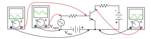
Figure 4.38: PNP version of common emitter amplifier.
