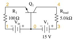
Figure 4.54: Common-base circuit for DC SPICE analysis.
