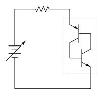
Figure 7.8: Powered Shockley diode equivalent circuit.
