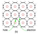
Figure 2.23: (a) Intrinsic semiconductor is an insulator having a complete electron shell. (b) However, thermal energy can create few electron hole pairs resulting in weak conduction.
