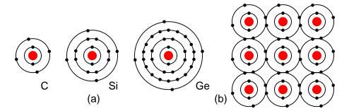
Figure 2.14: (a) Group IVA elements: C, Si, Ge having 4 electrons in the valence shell, (b) complete the valence shell by sharing electrons with other elements.
