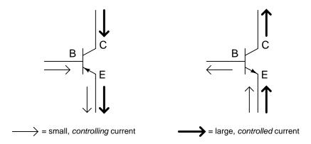
Figure 4.2: Small Base-Emitter current controls large Collector-Emitter current flowing against emitter arrow.
