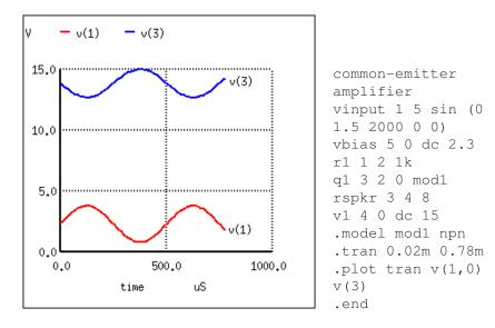
Figure 4.35: V(3), the output voltage across  $r_{spkr}$ , compared to the input.
