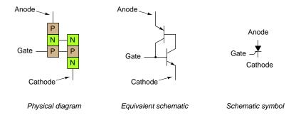
Figure 7.19: The Silicon-Controlled Rectifier (SCR)
