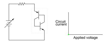
Figure 7.9: Zero applied voltage; zero current
