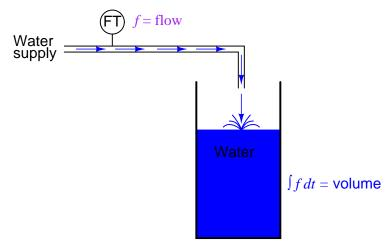
If we were to use a "Flow Transmitter" device to measure water flow, then by time-integration we could calculate the volume of water accumulated in the tank over time. Although it is theoretically possible to use a capacitive op-amp integrator circuit to derive a volume signal from a flow signal, mechanical and digital electronic "integrator" devices are more suitable for integration over long periods of time, and find frequent use in the water treatment and distribution industries.
