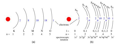
Figure 2.8: (a) Bohr representation of Silver atom, (b) Subshell representation of Ag with division of shells into subshells (angular quantum number l). This diagram implies nothing about the actual position of electrons, but represents energy levels.
