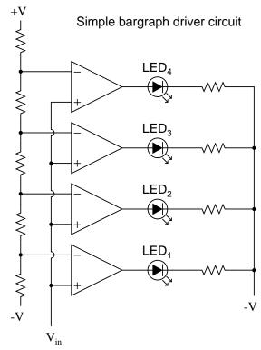
In the circuit shown above,  $LED_1$  would be the first to light up as the input voltage increased in a positive direction. As the input voltage continued to increase, the other LED's would illuminate in succession, until all were lit.
