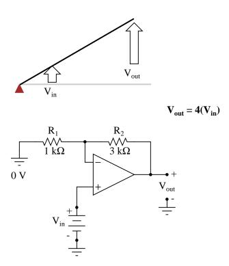
Inverting op-amp circuits may be modeled using the lever analogy as well. With the inverting configuration, the ground point of the feedback voltage divider is the op-amp's inverting input with the input to the left and the output to the right. This is mechanically equivalent to a *first-class* lever, where the input force (effort) is on the opposite side of the fulcrum from the output (load):
