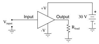
Without having to analyze the actual transistor design of the amplifier, you can readily discern the whole circuit's function: to take an input signal  $(V_{in})$ , amplify it, and drive a load
