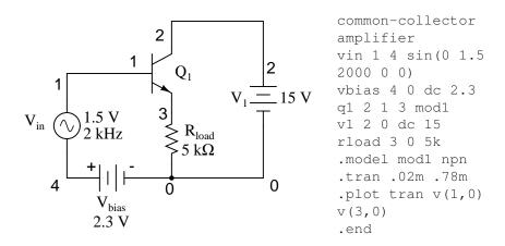
Figure 4.44: Common collector (emitter-follower) amplifier.
