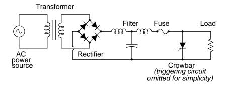
Figure 7.25: Crowbar circuit used in DC power supply
