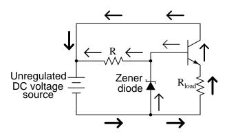
Figure 4.49: Common collector application: voltage regulator.
