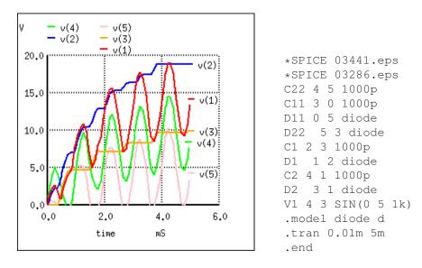
Figure 3.47: Voltage quadrupler: DC voltage available at v(3) and v(2). Intermediate waveforms: Clampers: v(5), v(4), v(1).
