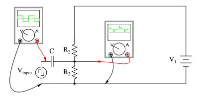
Figure 4.95: Capacitively coupled low frequency square-wave shows distortion.
