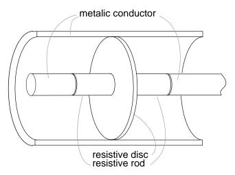
Coaxial T-attenuator for radio frequency work
