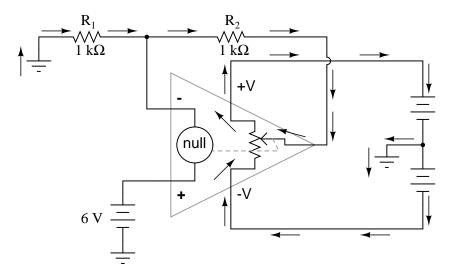
The 6 volt signal source does not have to supply any current for the circuit: it merely commands the op-amp to balance voltage between the inverting (-) and noninverting (+) input pins, and in so doing produce an output voltage that is twice the input due to the dividing effect of the two 1  $k\Omega$  resistors.
