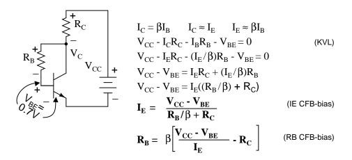
Figure 4.86: Collector-feedback bias.
