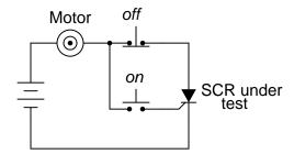
Figure 7.24: DC motor start/stop control circuit
