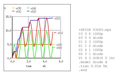
Figure 3.45: Voltage tripler: v(3) half-wave rectifier, v(4) input+ 5 V, v(1) clamper, v(2) final output.
