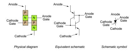
Figure 7.53: The Silicon-Controlled Switch(SCS)
