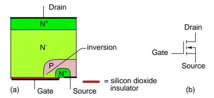
Figure 2.47: N-channel MOSFET (enhancement type): (a) Cross-section, (b) schematic symbol.
