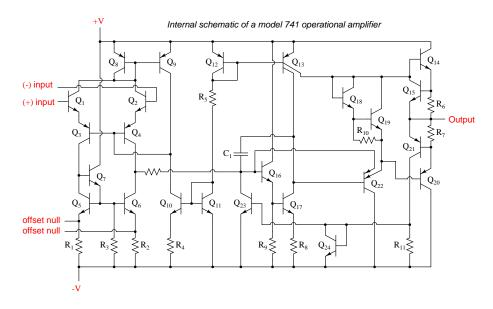
Figure 8.7: Schematic diagram of a model 741 op-amp.
