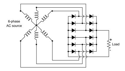
Figure 3.25: Six-phase full-wave bridge rectifier circuit.
