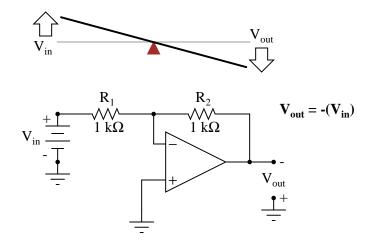
Changing the resistor ratio  $R_2/R_1$  changes the gain of the amplifier circuit, just as changing the fulcrum position on the lever changes its mechanical displacement "gain." Consider the following example, where  $R_2$  is made twice as large as  $R_1$ :
