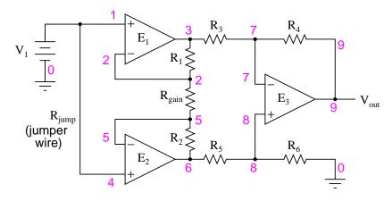
instrumentation amplifier v1 1 0 rin1 1 0 9e12 rjump 1 4 1e-12 9e12 0 0 1 2 999k 0 4 5 999k 9 0 8 7 999k rload 9 0 10k 2 3 10k rgain 2 5 10k r2 5 6 10k 3 7 10k 7 9 10k r5 6 8 10k
