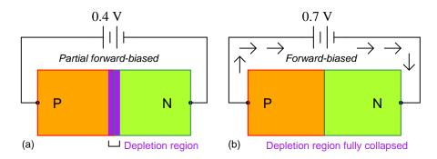
Figure 3.7: Inceasing forward bias from (a) to (b) decreases depletion region thickness.
