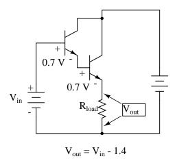
Figure 4.51: Darlington pair based common-collector amplifier loses two  $V_{BE}$  diode drops.
