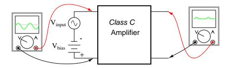
Figure 4.68: Class C: Conduction is for less than a half cycle (< 180°).
