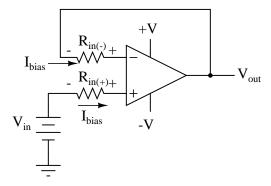
With the additional resistance added to the circuit, the output voltage will be closer to  $V_{in}$  than before, even if there is some offset between the two input currents.
