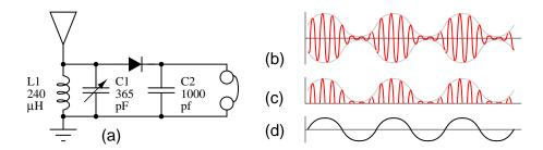
Figure 9.11: (a) Crystal radio. (b) Modulated RF at antenna. (c) Rectified RF at diode cathode, without C2 filter capacitor. (d) Demodualted audio to headphones.
