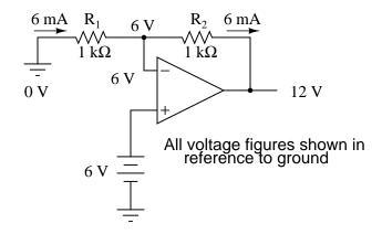
If  $R_1$  and  $R_2$  are both equal and  $V_{in}$  is 6 volts, the op-amp will output whatever voltage is needed to drop 6 volts across  $R_1$  (to make the inverting input voltage equal to 6 volts, as well, keeping the voltage difference between the two inputs equal to zero). With the 2:1 voltage divider of  $R_1$  and  $R_2$ , this will take 12 volts at the output of the op-amp to accomplish.
