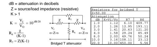
Figure 1.18: Formulas and abbreviated table for bridged-T attenuator section,  $Z = 50 \Omega$ .
