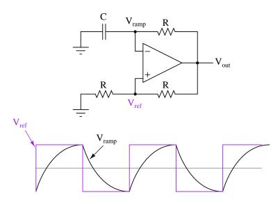
$V_{\text{out}}$  is a square wave just like  $V_{\text{ref}}$ , only taller
