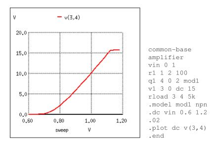
Figure 4.55: Common-base amplifier DC transfer function.
