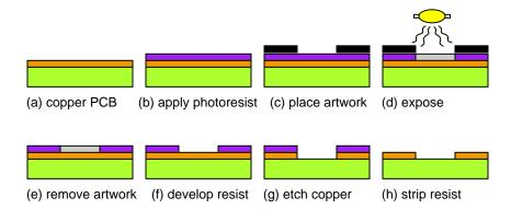
Figure 2.53: Processing of copper printed circuit boards is similar to the photo lithographic steps of semiconductor processing.
