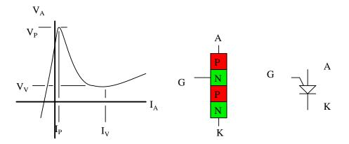
$Figure~7.49: \ Programmable~unijunction~transistor:~Characteristic~curve, internal~construction, schematic~symbol.$
