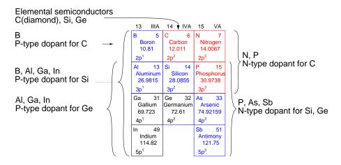
Figure 2.27: Group IIIA P-type dopants, group IV basic semiconductor materials, and group VA N-type dopants.
