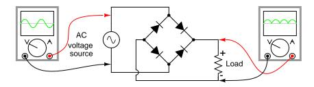
Figure 3.20: Full-wave bridge rectifier.
