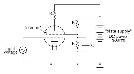
With a constant DC screen voltage, electron flow from cathode to plate became almost exclusively dependent upon grid voltage, meaning the plate voltage could vary over a wide range with little effect on plate current. This made for more stable gains in amplifier circuits, and better linearity for more accurate reproduction of the input signal waveform.
