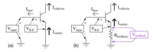
Figure 4.108: (a) No feedback vs (b) emitter feedback. A waveform at the collector is inverted with respect to the base. At (b) the emitter waveform is in-phase (emitter follower) with base, out of phase with collector. Therefore, the emitter signal subtracts from the collector output signal.
