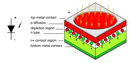
Figure 3.74: Photodiode: Schematic symbol and cross section.
