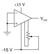
Potentiometer adjusted so that  $V_{out} = 0$  volts with inputs shorted together
