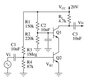
Figure 9.21: Class A cascode small-signal high gain amplifier.
