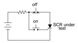
Figure 7.23: SCR testing circuit
