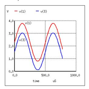
Figure 4.45: Common collector (emitter-follower): Output V3 follows input V1 less a  $0.7 \ VVBE$  drop.
