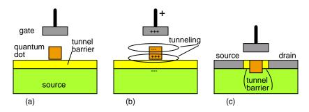
Figure 2.62: (a) Single electron box, an isolated quantum dot separated from an electron source by an insulator. (b) Positive charge on the gate polarizes quantum dot, tunneling an electron from the source to the dot. (c) Quantum transistor: channel is replaced by quantum dot surrounded by tunneling barrier.
