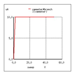
As expected for any transistor, the controlled current holds steady at a regulated value over a wide range of power supply voltages. In this case, that regulated point is 10  $\mu$ A (1.000E-05). Now let's see what happens when we apply a negative voltage to the gate (with reference to the source) and sweep the power supply over the same range of 0 to 50 volts:
