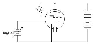
As the signal voltage increases, current through the tube is choked off. This decreases the voltage between the plate and the fluorescent screen, lessening the shadow effect (shadow narrows).
