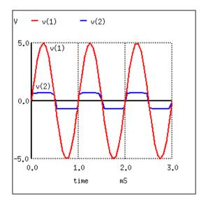
Figure 3.33: Diode D1 clips at -0.7 V as it conducts during negative peaks. D2 conducts for positive peaks, clipping at 0.7V.
