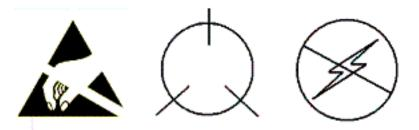
These are some of the more common logos associated with anti-static labels. They are used to inform the user that the contents are static sensitive.
