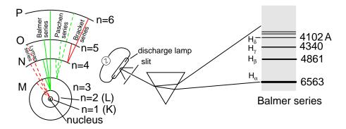
Figure 2.3: Bohr hydrogen atom (with orbits drawn to scale) only allows electrons to inhabit discrete orbitals. Electrons falling from n=3,4,5, or 6 to n=2 accounts for Balmer series of spectral lines.
