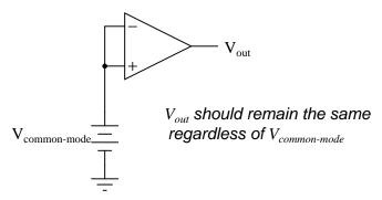
Voltage that is common between either of the inputs and ground, as " $V_{common-mode}$ " is in this case, is called *common-mode voltage*. As we vary this common voltage, the perfect differential amplifier's output voltage should hold absolutely steady (no change in output for any arbitrary change in common-mode input). This translates to a *common-mode voltage gain* of zero.
