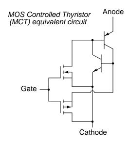
Figure 7.56: MOS-controlled thyristor (MCT) equivalent circuit
