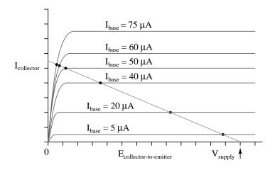
Figure 4.74: More base current curves shows saturation detail.
