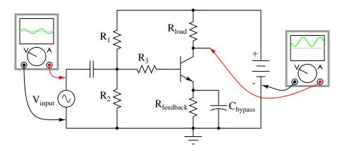
Figure 4.110: High AC voltage gain reestablished by adding  $C_{bupass}$  in parallel with  $R_{feedback}$
