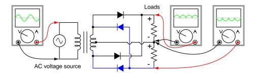
Figure 3.19: Dual polarity full-wave center tap rectifier
