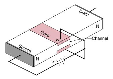
Figure 2.38: Junction field effect transistor cross-section.
