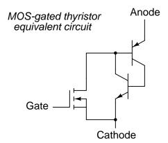
Figure 7.55: MOS-gated thyristor equivalent circuit
