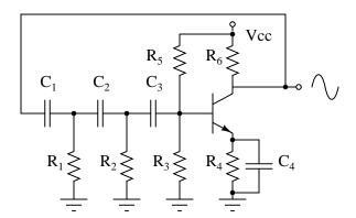
Figure 9.9: Phase shift oscillator.  $R_1C_1$ ,  $R_2C_2$ , and  $R_3C_3$  each provide  $60^\circ$  of phase shift.
