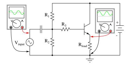
Figure 4.109: Common collector (emitter follower) amplifier.
