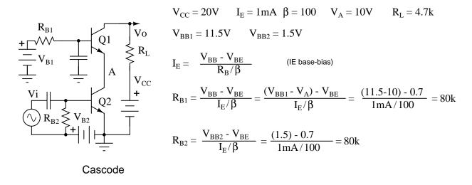
Figure 4.93: Bias for a cascode amplifier.
