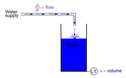
A "Level Transmitter" device mounted on a water storage tank provides a signal directly proportional to water level in the tank, which – if the tank is of constant cross-sectional area throughout its height – directly equates water volume stored. If we were to take this volume signal and differentiate it with respect to time (dv/dt), we would obtain a signal proportional to the water *flow rate* through the pipe carrying water to the tank. A differentiator circuit
