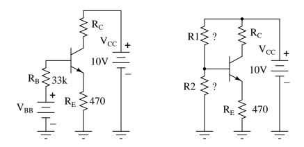
Figure 4.92: Emitter-bias example converted to voltage divider bias.
