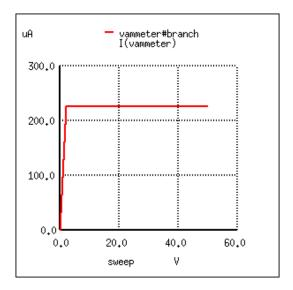
As expected, the drain current is greater now than it was in the previous simulation. With less reverse-bias voltage impressed across the gate-source junction, the depletion region is not as wide as it was before, thus "opening" the channel for charge carriers and increasing the drain current figure.
