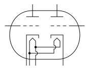
The 12AX7 and 12AU7 models are common examples of dual-triode tubes, both of low-power rating. The 12AX7 is especially common as a preamplifier tube in electric guitar amplifier circuits.
