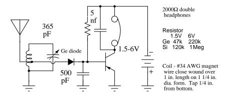
Figure 9.13: Crystal radio with one transistor audio amplifer, base-bias. After Stoner, Figure 4.3A. [8]
