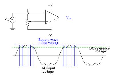
Any time there is a transition through the reference voltage level, no matter how tiny that transition may be, the output of the comparator will switch states, producing a square wave with "glitches."
