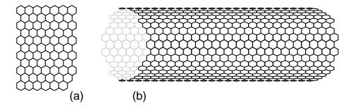
Figure 2.63: (a) Graphene: A single sheet of the graphite allotrope of carbon. The atoms are arranged in a hexagonal pattern with a carbon at each intersection. (b) Carbon nanotube: A rolled-up sheet of graphene.
