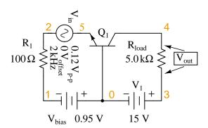
Figure 4.56: Common-base circuit for SPICE AC analysis.
