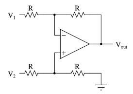
If all the resistor values are equal, this amplifier will have a differential voltage gain of 1. The analysis of this circuit is essentially the same as that of an inverting amplifier, except that the noninverting input (+) of the op-amp is at a voltage equal to a fraction of  $V_2$ , rather than being connected directly to ground. As would stand to reason,  $V_2$  functions as the noninverting input and  $V_1$  functions as the inverting input of the final amplifier circuit. Therefore:
