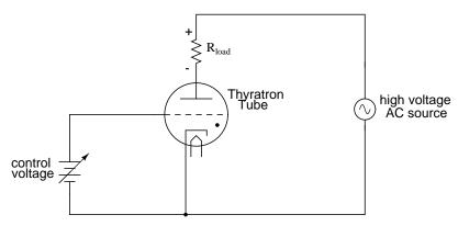
It should be noted that the schematic shown above is greatly simplified for most purposes and thyratron tube designs. Some thyratrons, for instance, required that the grid voltage switch polarity between their "on" and "off" states in order to properly work. Also, some thyratrons had more than one grid!
