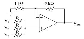
With a voltage divider composed of a  $2 \ k\Omega \ / \ 1 \ k\Omega$  combination, the noninverting amplifier circuit will have a voltage gain of 3. By taking the voltage from the passive averager, which is the sum of  $V_1$ ,  $V_2$ , and  $V_3$  divided by 3, and multiplying that average by 3, we arrive at an output voltage equal to the sum of  $V_1$ ,  $V_2$ , and  $V_3$ :
