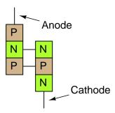
Figure 7.6: Transistor equivalent of Shockley diode
