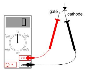
Figure 7.21: Rudimentary test of SCR
