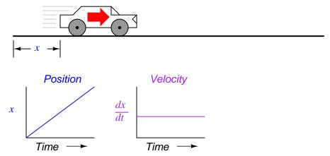
For a linear graph of x over time, the derivate of position (dx/dt), otherwise and more commonly known as *velocity*, will be a flat line, unchanging in value. The derivative of a mathematical function may be graphically understood as its *slope* when plotted on a graph,
