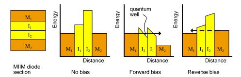
Figure 2.61: Metal insulator insulator metal (MIIM) diode: Cross section of diode. Energy levels for no bias, forward bias, and reverse bias. After Figure 1 [21].
