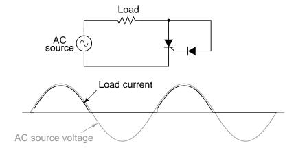
Figure 7.28: Gate connected directly to anode through a diode; nearly complete half-wave current through load.
