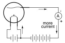
Sure enough, the presence of the battery created a much larger current from the filament to the metal strip. However, when the battery was turned around, there was little to no current at all!
