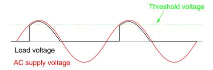
Figure 7.3: Thyratron waveforms
