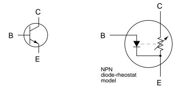
Figure 4.18: Elementary diode resistor transistor model.
