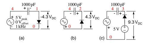
Figure 3.37: Clampers: (a) Positive peak clamped to 0 V. (b) Negative peak clamped to 0 V. (c) Negative peak clamped to 5 V.
