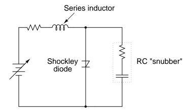
Figure 7.16: Both the series inductor and parallel resistor-capacitor "snubber" circuit help minimize the Shockley diode's exposure to excessively rising voltage.
