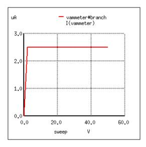
Not surprisingly, the drain current is now regulated at a lower value of 2.5  $\mu$ A (down from 10  $\mu$ A with zero input voltage). Now let's apply an input voltage of the other polarity, to *enhance* the IGFET:
