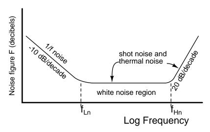
Figure 4.121: Small signal transistor noise figure vs Frequency. After Thiele, Figure 11.147 [1]
