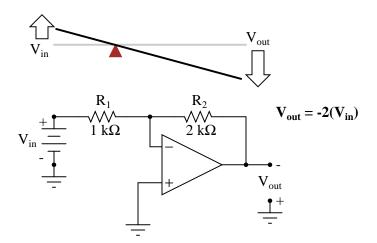
With the inverting amplifier configuration, though, gains of less than 1 are possible, just as with first-class levers. Reversing  $R_2$  and  $R_1$  values is analogous to moving the fulcrum to its complementary position on the lever: one-third of the way from the output end. There, the output displacement will be one-half the input displacement:
