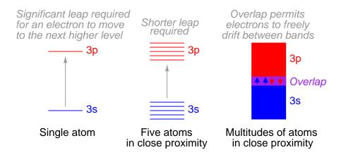
Figure 2.20: Electron band overlap in metallic elements.
