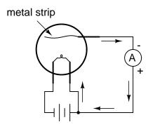
The white-hot filament in Edison's lamp was liberating free electrons into the vacuum of the lamp, those electrons finding their way to the metal strip, through the galvanometer, and back to the filament. His curiosity piqued, Edison then connected a fairly high-voltage battery in the galvanometer circuit to aid the small current:
