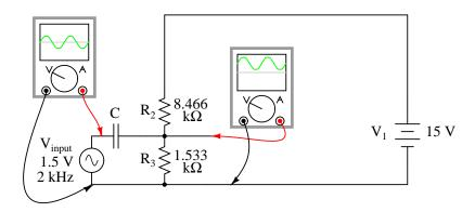
Figure 4.81: Combined AC and DC circuit.
