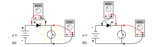
Figure 3.4: Diode circuit voltage measurements: (a) Forward biased. (b) Reverse biased.
