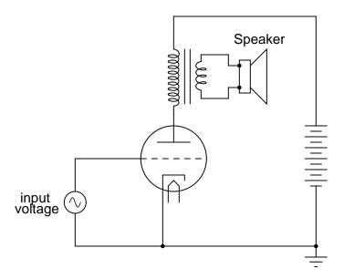
If we substitute a tetrode for a triode in this circuit, we will see improvements in circuit gain resulting from the electrostatic shielding offered by the screen, preventing unwanted feedback between the plate and control grid:
