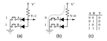
Figure 3.53: Diode AND gate
