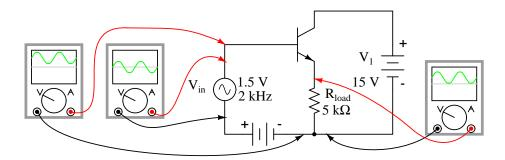
Figure 4.46: Common collector non-inverting voltage gain is 1.
