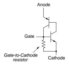
Figure 7.22: Larger SCRs have gate to cathode resistor.
