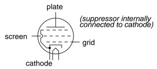
The suppressor's job was to repel any secondarily emitted electrons back to the plate: a structural equivalent of the beam power tube's space charge. This, of course, increased plate current and decreased screen current, resulting in better gain and overall performance. In some instances it allowed for greater operating plate voltage as well.
