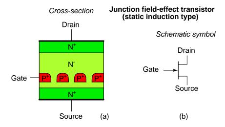
Figure 2.43: Junction field effect transistor (static induction type): (a) Cross-section, (b) schematic symbol.
