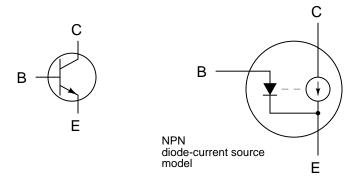
Figure 4.31: The model shows that base current flow in on direction.
