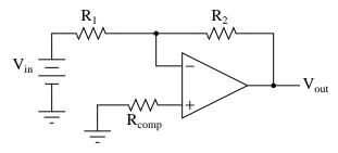
$$R_{comp} = R_1 // R_2$$
