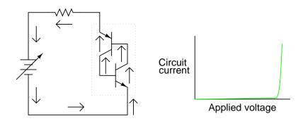
Figure 7.12: Transistors are now fully conducting.
