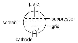
The suppressor was another wire coil or mesh situated between the screen and the plate, usually connected directly to ground potential. In some pentode tube designs, the suppressor was internally connected to the cathode so as to minimize the number of connection pins having to penetrate the tube envelope:
