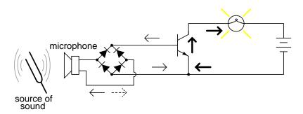
Figure 4.27: Transistor switch activated by audio.
