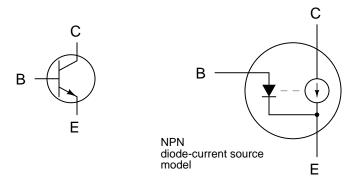
Figure 4.19: Current source model of transistor.
