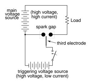
Spark gaps of both the triggered and untriggered variety can be built to handle huge amounts of current, some even into the range of mega-amps (millions of amps)! Physical size is the primary limiting factor to the amount of current a spark gap can safely and reliably handle.
