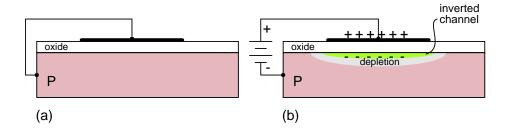
Figure 2.45: N-channel MOS capacitor: (a) no charge, (b) charged.
