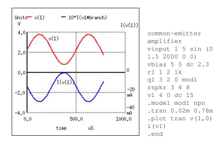
Figure 4.33: Undistorted output current I(v(1)) due to Vbias
