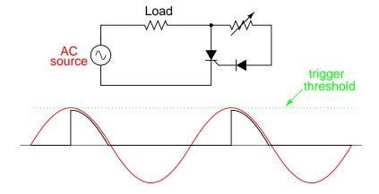
Figure 7.31: Circuit at minimum power setting
