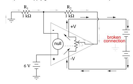
No electrons may flow in or out of the op-amp's output terminal, because the pathway to the power supply is a "dead end." Thus, no electrons flow through the ground connection to the left of  $R_1$ , neither through the feedback loop. This effectively renders the op-amp useless: it can neither sustain current through the feedback loop, nor through a grounded load, since there is no connection from any point of the power supply to ground.
