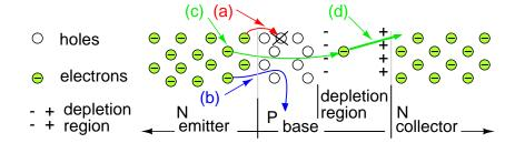
Figure 2.35: Disposition of electrons entering base: (a) Lost due to recombination with base holes. (b) Flows out base lead. (c) Most diffuse from emitter through thin base into base-collector depletion region, and (d) are rapidly swept by the strong depletion region electric field into the collector.
