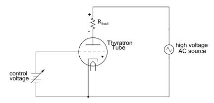
Figure 7.2: Simple thyratron control circuit
