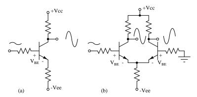
Figure 4.120: (a) single ended CE amplifier vs (b) differential amplifier with  $V_{\it BE}$  cancellation.
