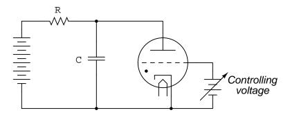
Figure 7.4: Voltage controlled thyratron relaxation oscillator
