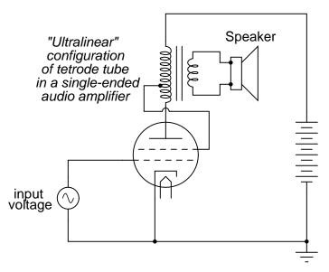
This signal feedback results in significant improvements in amplifier linearity (and consequently, distortion), so long as precautions are taken against "overpowering" the screen with
