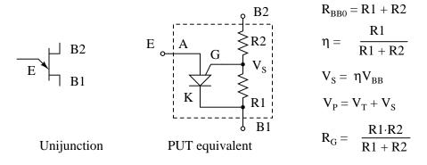
Figure 7.50: PUT equivalent of unijunction transistor
