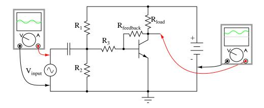
Figure 4.106: Negative feedback, collector feedback, decreases the output signal.
