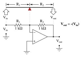
With equal-value resistors (equal-lengths of lever on each side of the fulcrum), the output voltage (displacement) will be equal in magnitude to the input voltage (displacement), but of the opposite polarity (direction). A positive input results in a negative output:
