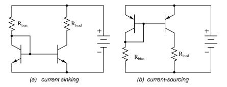
Figure 4.115: Current mirror circuits.
