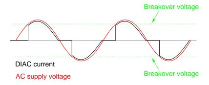
Figure 7.18: DIAC waveforms
