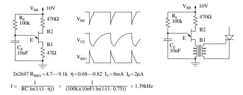
Figure 7.48: Unijunction transistor relaxation oscillator and waveforms. Oscillator drives SCR.
