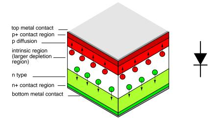
Figure 3.81: Pin diode: Cross section aligned with schematic symbol.
