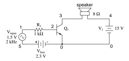
Figure 4.32:  $V_{bias}$  keeps transistor in the active region.
