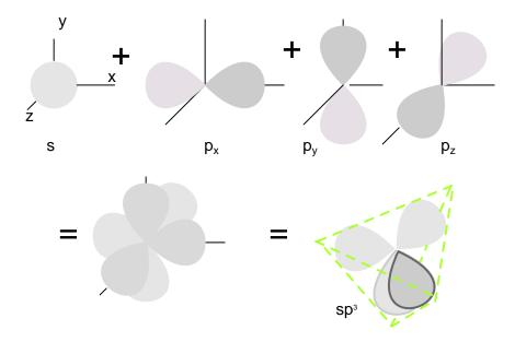
Figure 2.17: One s-orbital and three p-orbital electrons hybridize, forming four  ${\rm sp^3}$  molecular orbitals.
