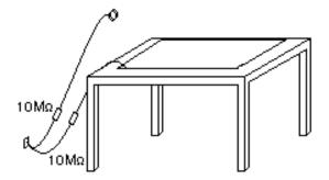
Correctly grounded station, the table surface and wrist strap each have their own path to ground.
