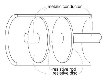
Coaxial  $\Pi$ -attenuator for radio frequency work
