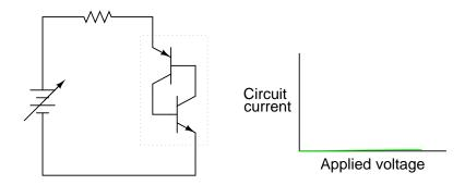
Figure 7.10: Some applied voltage; still no current
