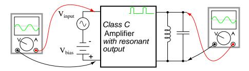
Figure 4.69: Class C amplifier driving a resonant circuit.
