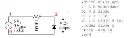
Figure 3.30: Clipper: clips negative peak at -0.7 V.
