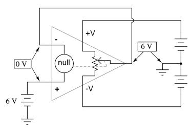
As the "potentiometer" will move to provide an output voltage necessary to satisfy the "null detector" at an "indication" of zero volts, the output voltage becomes equal to the input voltage: in this case, 6 volts. If the input voltage changes at all, the "potentiometer" inside the op-amp will change position to hold the "null detector" in balance (indicating zero volts), resulting in an output voltage approximately equal to the input voltage at all times.
