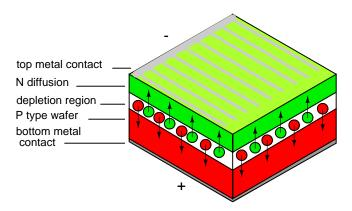
Figure 3.76: Silicon Solar cell
