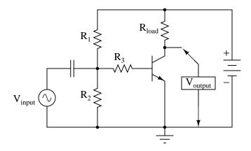
Figure 4.104: Common-emitter amplifier without feedback.
