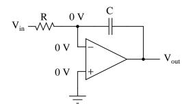
As before, the negative feedback of the op-amp ensures that the inverting input will be held at 0 volts (the virtual ground). If the input voltage is exactly 0 volts, there will be no current through the resistor, therefore no charging of the capacitor, and therefore the output voltage will not change. We cannot guarantee what voltage will be at the output with respect to ground in this condition, but we can say that the output voltage *will be constant*.
