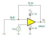
Figure 8.1: OPA227 Non-inverting stage
