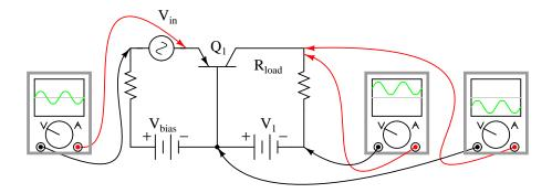
Figure 4.59: Phase relationships and offsets for PNP common base amplifier.
