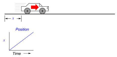
If we were to calculate the *derivative* of the car's position with respect to time (that is, determine the rate-of-change of the car's position with respect to time), we would arrive at a quantity representing the car's velocity. The differentiation function is represented by the fractional notation d/d, so when differentiating position (x) with respect to time (t), we denote the result (the derivative) as dx/dt:
