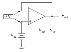
Whether the output is directly fed back to the inverting (-) input or coupled through a set of components, the effect is the same: the extremely high differential voltage gain of the op-amp will be "tamed" and the circuit will respond according to the dictates of the feedback "loop" connecting output to inverting input.
