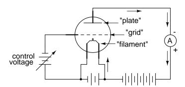
plate current can be controlled by the application of a small control voltage between the grid and filament!
