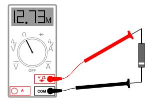
Figure 3.13: Ohmmeter equipped with a low test voltage, too low to forward bias diodes, does not see diodes.
