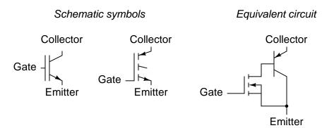
In essence, the IGFET controls the base current of a BJT, which handles the main load current between collector and emitter. This way, there is extremely high current gain (since the insulated gate of the IGFET draws practically no current from the control circuitry), but the collector-to-emitter voltage drop during full conduction is as low as that of an ordinary BJT.
