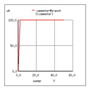
Sure enough, the drain current remains steady at a value of 100  $\mu$ A (1.000E-04 amps) no matter how high the power supply voltage is adjusted.
