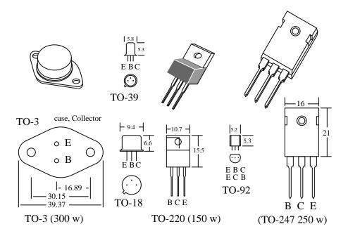
Figure 4.117: Transistor packages, dimensions in mm.
