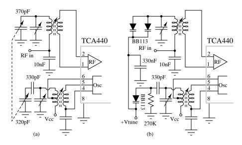
Figure 9.16: IC radio comparison of (a) mechanical tuning to (b) electronic varicap diode tuning.[3]
