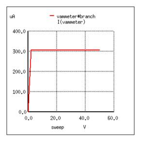
With the gate-source voltage set to 0.25 volts, one-half what it was before, the drain current is 306.3  $\mu$ A. Although this is still an increase over the 225  $\mu$ A from the prior simulation, it isn't proportional to the change of the controlling voltage.
