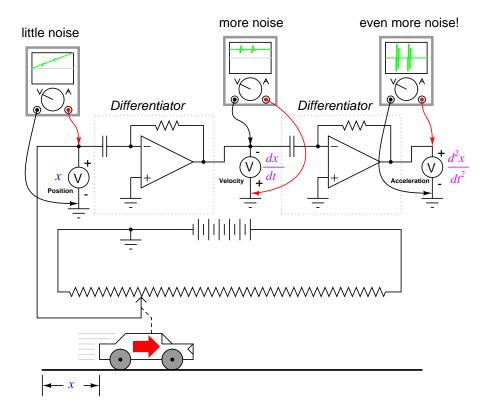
Integration does not suffer from this problem, because integrators act as low-pass filters, attenuating high-frequency input signals. In effect, all the high and low peaks resulting from noise on the signal become averaged together over time, for a diminished net result. One might suppose, then, that we could avoid all trouble by measuring acceleration directly and integrating that signal to obtain velocity; in effect, calculating in "reverse" from the way shown previously:
