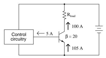
It would be nice from the standpoint of control circuitry to have power transistors with high current gain, so that far less current is needed for control of load current. Of course, we can use Darlington pair transistors to increase the current gain, but this kind of arrangement still requires *far* more controlling current than an equivalent power IGFET:
