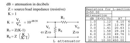
Figure 1.17: Alternate form L-section attenuator table for  $50 \Omega$  source and load impedance.
