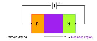
Figure 3.6: Depletion region expands with reverse bias.
