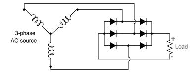
Figure 3.24: Three-phase full-wave bridge rectifier circuit.
