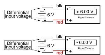
Just as a voltmeter will only display the voltage *between* its two test leads, an ideal differential amplifier only amplifies the potential difference between its two input connections, not the voltage between any one of those connections and ground. The output polarity of a differential amplifier, just like the signed indication of a digital voltmeter, depends on the relative polarities of the differential voltage between the two input connections.
