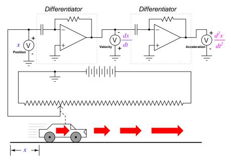
Deriving velocity from position, and acceleration from velocity, we see the principle of differentiation very clearly illustrated. These are not the only physical measurements related to each other in this way, but they are, perhaps, the most common. Another example of calculus in action is the relationship between liquid flow (q) and liquid volume (v) accumulated in a vessel over time:
