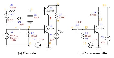
Figure 4.62: SPICE: Cascode and common-emitter for comparison.
