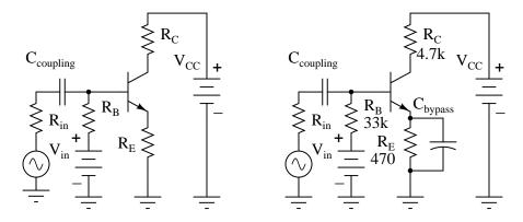
Figure 4.89: Chypass is required to prevent AC gain reduction.
