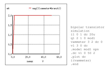
Figure 4.15: Sweeping collector voltage 0 to 50 V with base current constant at 20  $\mu$ A yields constant 2 mA collector current.
