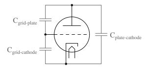
Now, this stray capacitance is quite small, and the reactive impedances usually high. Usually, that is, unless radio frequencies are being dealt with. As we saw with De Forest's Audion tube, radio was probably the prime application for this new technology, so these "tiny" capacitances became more than just a potential problem. Another refinement in tube technology was necessary to overcome the limitations of the triode.
