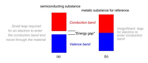
Figure 2.22: Electron band separation in semiconducting substances, (a) multitudes of semiconducting close atoms still results in a significant band gap, (b) multitudes of close metal atoms for reference.
