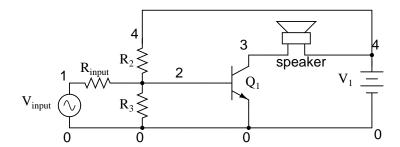
Figure 4.98: Direct coupled amplifier: direct coupling to speaker.
