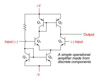
Figure 8.6: A simple operational amplifier made from discrete components.
