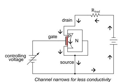
Illustrating the proper biasing polarities with standard IGFET symbols:
