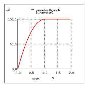
Here, the controlling signal is a steady voltage of 1 volt, applied with negative towards the JFET gate and positive toward the JFET source, to reverse-bias the PN junction. In the first BJT simulation of chapter 4, a constant-current source of 20  $\mu$ A was used for the controlling signal, but remember that a JFET is a *voltage-controlled* device, not a current-controlled device like the bipolar junction transistor.
