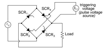
Figure 7.36: This strategy will not work for triggering SCR<sub>2</sub> and SCR<sub>4</sub> as a pair.
