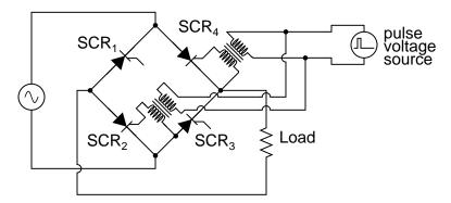
Figure 7.37: Transformer coupling of the gates allows triggering of SCR<sub>2</sub> and SCR<sub>4</sub>.
