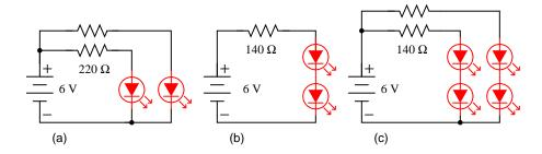
Figure 3.71: Multiple LEDs: (a) In parallel, (b) in series, (c) series-parallel
