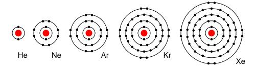
Figure 2.13: Group VIIIA elements: He, Ne, Ar, Kr, Xe are largely unreactive since the valence shell is complete..
