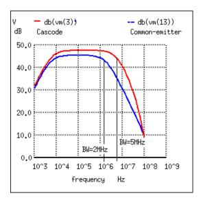
Figure 4.64: Cascode vs common-emitter banwidth.
