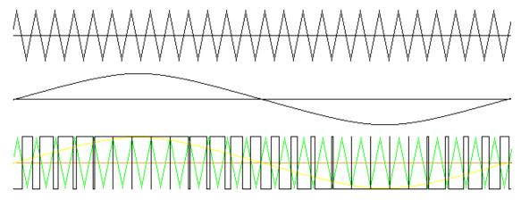
How an Audio Signal is modulated with PWM
