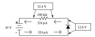
Figure 3.60: Zener regulator with 100 k $\Omega$  resistor.
