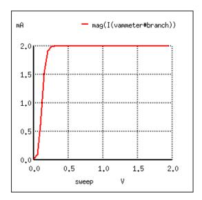
Figure 4.14: A Sweeping collector voltage 0 to 2 V with base current constant at 20  $\mu$ A yields constant 2 mA collector current in the saturation region.
