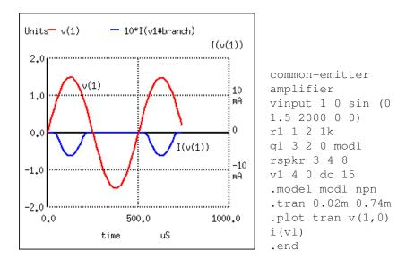
Figure 4.30: Signal clipped at collector due to lack of DC base bias.
