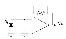
Figure 9.25: Photodiode amplifier.
