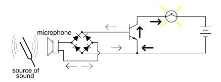
Figure 4.7: Amplified microphone signal is rectified to DC to bias the base of the transistor providing a larger collector current.
