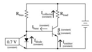
Figure 4.114: Diode junction 0.7 V maintains constant base voltage, and constant base current.
