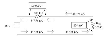
Figure 3.63: Non-regulator with Zener removed.
