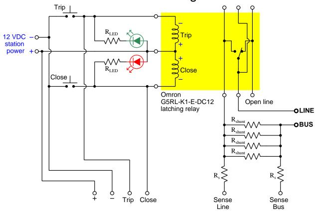
$R_{\rm shunt}$  resistors provide a means to infer current through breaker, by producing a voltage drop proportional to current.
