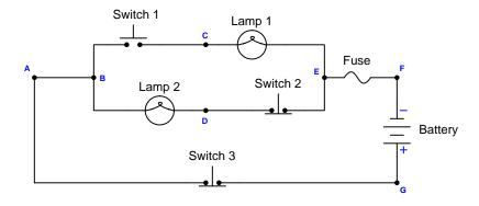
Identify the likelihood of each specified fault. Consider each fault one at a time (i.e. no coincidental faults), determining whether or not each fault is compatible with *all* measurements and symptoms in this circuit.
