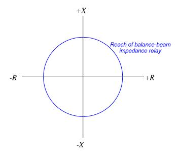
Any line condition placing the impedance phasor tip within this circle will cause the relay to trip. Any line condition placing the impedance phasor tip outside this circle will cause the relay to be restrained (i.e. it will not trip). Thus, the reach of this relay is represented by the radius of the circle sketched on the R-X diagram.
