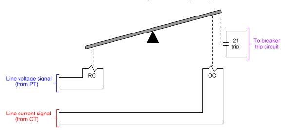
Balance-beam impedance relay design
