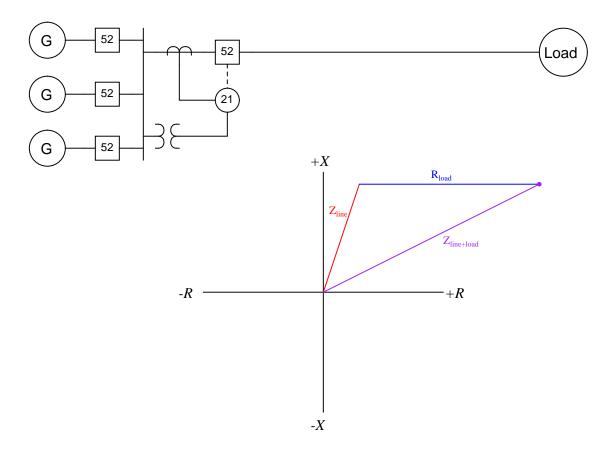
Short-circuit faults at various locations along a transmission line will cause the impedance phasor to vary primarily in magnitude and angle. Recall that during fault conditions, the resistance and reactance of the power line itself is the dominant impedance limiting fault current. The actual fault is predominantly resistive, with a very small impedance value.
