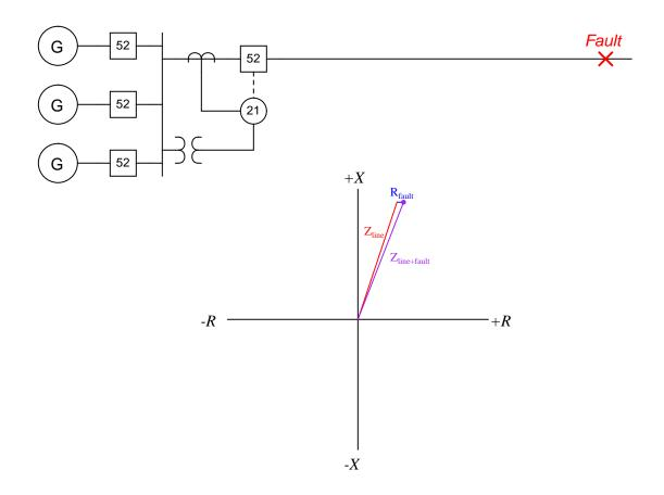
For a fault closer to the relay, the impedance phasor will be short (i.e. low impedance) with angle slightly less than that of the line impedance alone:
