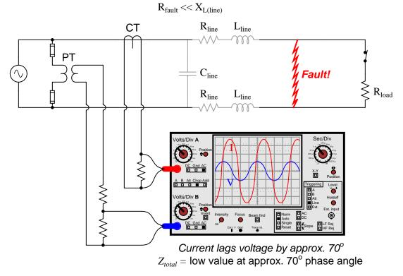
Line fault -- line inductive reactance dominates circuit impedance
