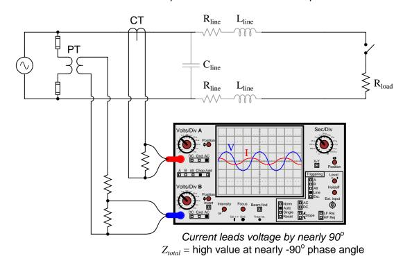
Load disconnected -- line capacitance dominates circuit impedance
