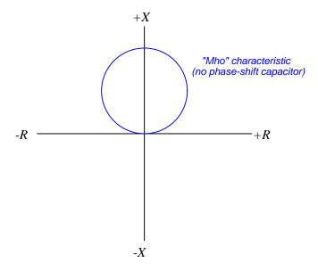
This relay's reach is defined as any impedance falling within the circle, just as we defined the reach of the impedance relay. The difference here, of course, is that the "mho" distance relay is entirely insensitive to conditions within the lower quadrants of the R-X diagram.
