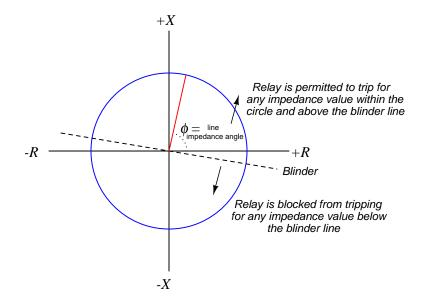
Phase-shifting components inside the directional relay mechanism tilt its blinder characteristic slightly clockwise from its natural (horizontal) characteristic. As you can see, the blinder prevents all operation in the lower-left quadrant, restricting operation of the impedance relay primarily to the upper-right and upper-left quadrants, with only a small portion of the lower-right quadrant active.
