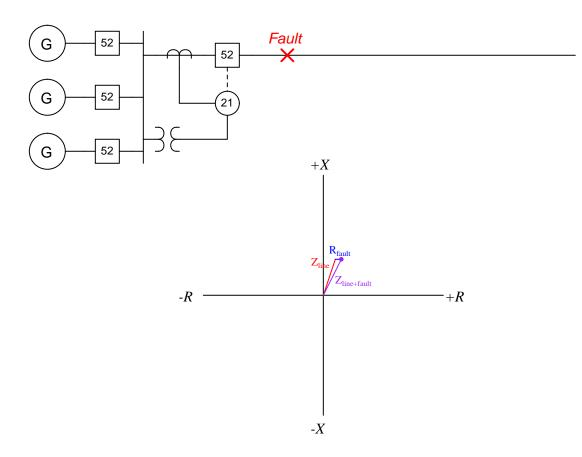
The goal of a distance relay (ANSI/IEEE code 21) is to trip its circuit breaker(s) if a fault occurs within its programmed "reach" and to ignore both normal operating loads and faults lying outside its reach.
