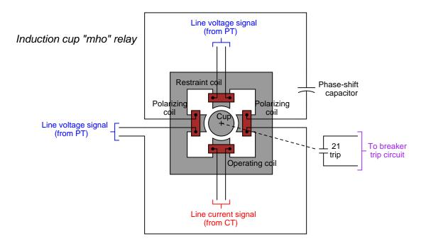
The amount of torque induced on the rotor (cup) is described by the following formula:
