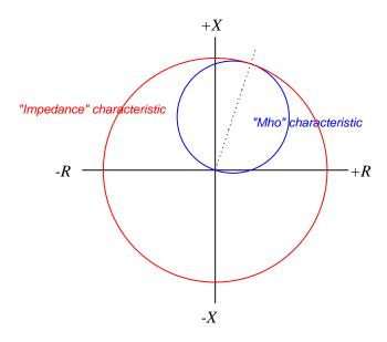
The "mho" relay reaches farthest only along the transmission line, while the impedance relay reaches the same distance indiscriminately
