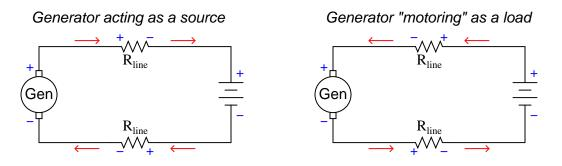
A generator acting as a source (in this case, to charge the battery) is fulfilling its intended function. A generator running as a motor, drawing energy from the battery as a load, is most definitely not fulfilling its intended function. Therefore, we would consider any current in the wrong (generator as load) direction to be excessive, while considerable current in the correct (generator as source) direction would be considered perfectly normal. If we were to install an overcurrent relay in
