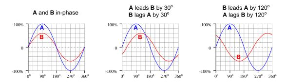
When two waveform reach their respective peaks at different times, the waveform that's ahead is said to be *leading* and the waveform that's behind is said to be *lagging*. Quantifying phase shift is as easy as measuring the difference in time between respective features (e.g. between positive peaks, between negative peaks, or between zero-crossing points of similar slope) and comparing that to the period, setting that quotient equal to a ratio between phase shift ( $\theta$ ) and 360°:
