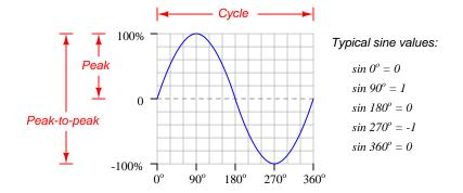
By definition, one *cycle* of a wave is 360 degrees of revolution, during which the wave will reach both a positive peak value as well as a negative peak value. *Peak* value, in fact, is a simple method of quantifying AC amplitude. Sometimes it is useful to express an AC quantity in terms of its over-all wave height from positive peak to negative peak, and we call this the *Peak-to-Peak* amplitude of the wave.
