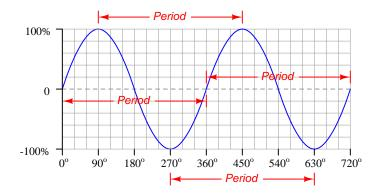
Period is typically measured in seconds, and the reciprocal of period is called *frequency* (f) which used to be measured in *cycles per second* (cps) but now has its own unit of the *Hertz* (Hz)<sup>4</sup>. For example, in many parts of the world the standard frequency for AC power systems is 60 Hz, equating to a period of 16.67 milliseconds. In other parts of the world the standard frequency for AC electric power is 50 Hz, with a period of 20 milliseconds.
