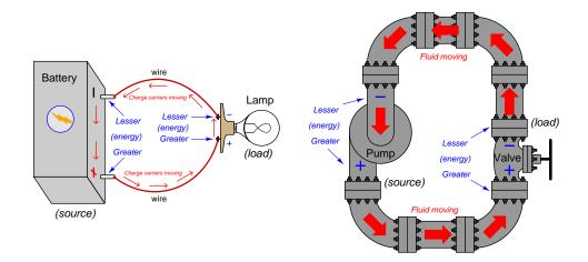
Each of these systems, in both orientations, delivers energy from source to load. Neither the electric lamp nor the hydraulic valve functions differently when direction of flow and voltage (pressure) polarities reverse. In fact, if the source in each circuit were replaced by one that periodically *oscillated* in direction, each system would continue to transfer energy from source to load, albeit in pulses rather than continuously.
