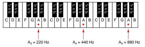
In the *equal-temperament* pitch system, each interval in the twelve-step division represents the same ratio of frequencies. Specifically, we may mathematically predict the next pitch in a twelve-tone equal-temperament system using the following formula:
