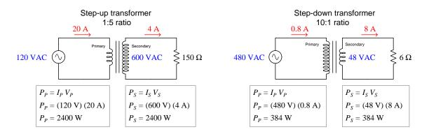
As you might imagine, an electrical component having no moving parts that is able to convert high-voltage to low-voltage (and vice-versa) is very useful, especially for electrical power systems. The fact that these devices require AC and cannot function on DC is one of the most significant historical reasons why AC triumphed over DC for electrical power distribution.
