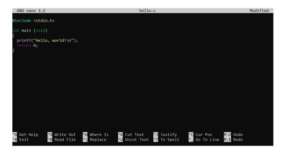
In order to save this new code to the file we must press Control-O ("Write Out"), or simply press Control-X ("Exit") to quit the text editor application. Like most editors, nano will ask the user if they wish to save any changes made to the file before exiting.
