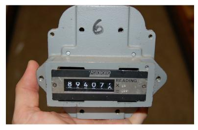
The fact that this instrument's display resembles the odometer of an automobile is no coincidence. Odometers are really just another form of mechanical integrator, "totalizing" the distance traveled by a vehicle. If the speedometer of a vehicle registers speed (v) in units of miles per hour, then the odometer will accumulate a distance  $(\Delta x)$  in units of miles, since distance (miles) is the time-integral of speed (miles per hour):
